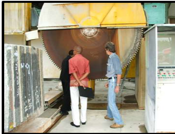
Figure 21: An example of a blade used to cut granite slabs
