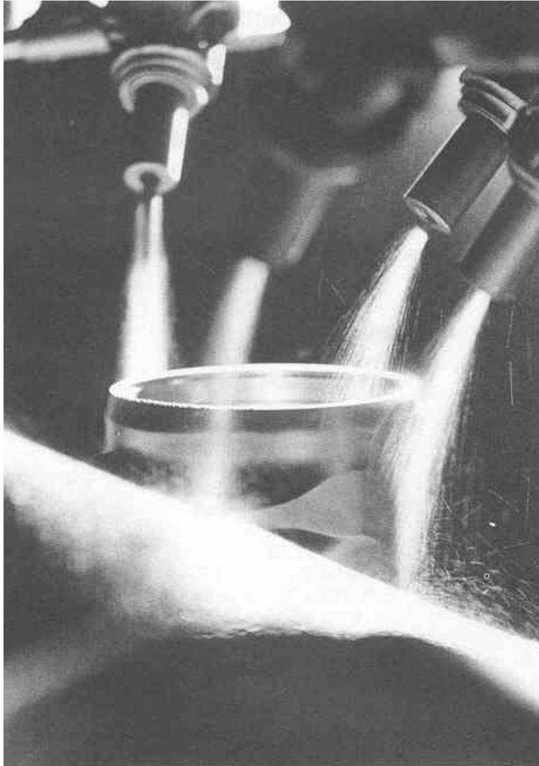
*Figure 7 Photo of shot peening in progress* <sup>[14]</sup>
