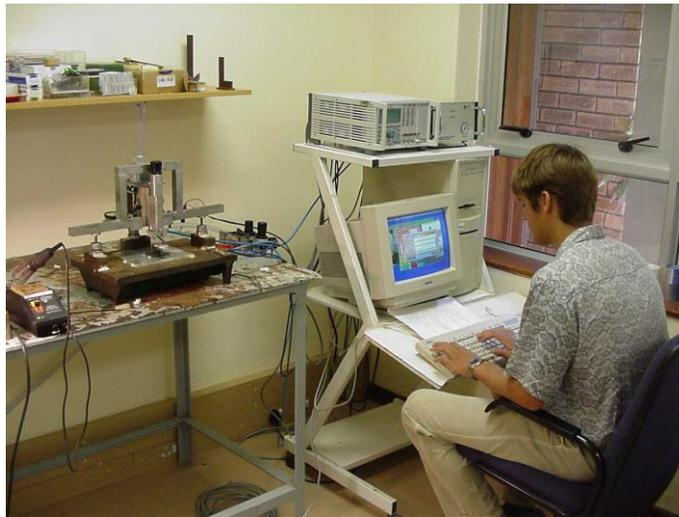
Figure 53 Air turbine hole drilling machine at NMMU
