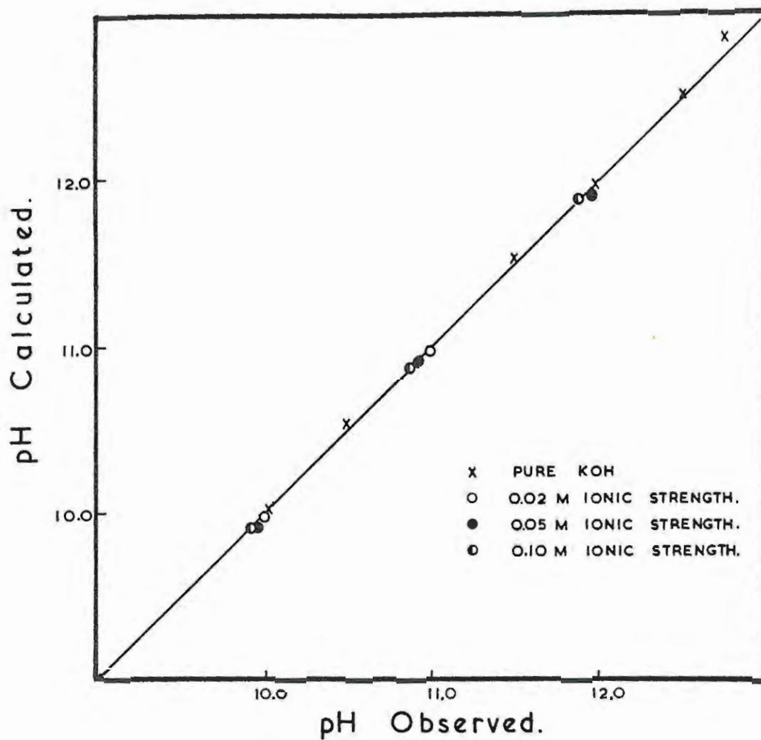
Fig. 15. Calibration of glass electrode No. 40308.
