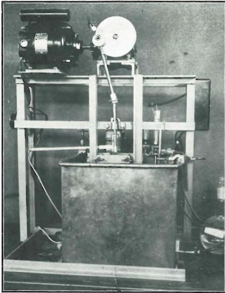
Fig. 6.. *Automatic pumping machine constructed to operate at 20 strokes/minute.*
