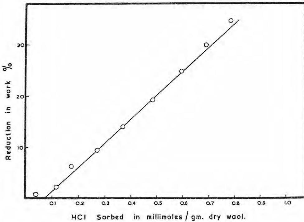
Fig. 1. (a, b). *The mechanical properties of wool fibres treated with dilute acid solutions* <sup>(1)</sup>.
