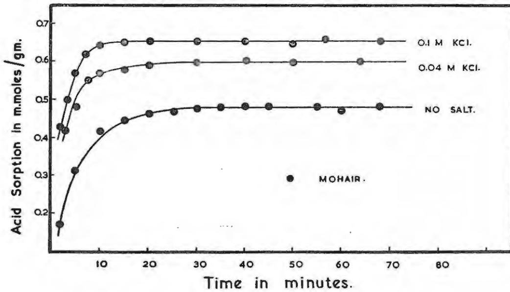
Fig. 7a (above). The sorption rate of HCl by wool and mohair at 25°C using the automatic pumping apparatus.
