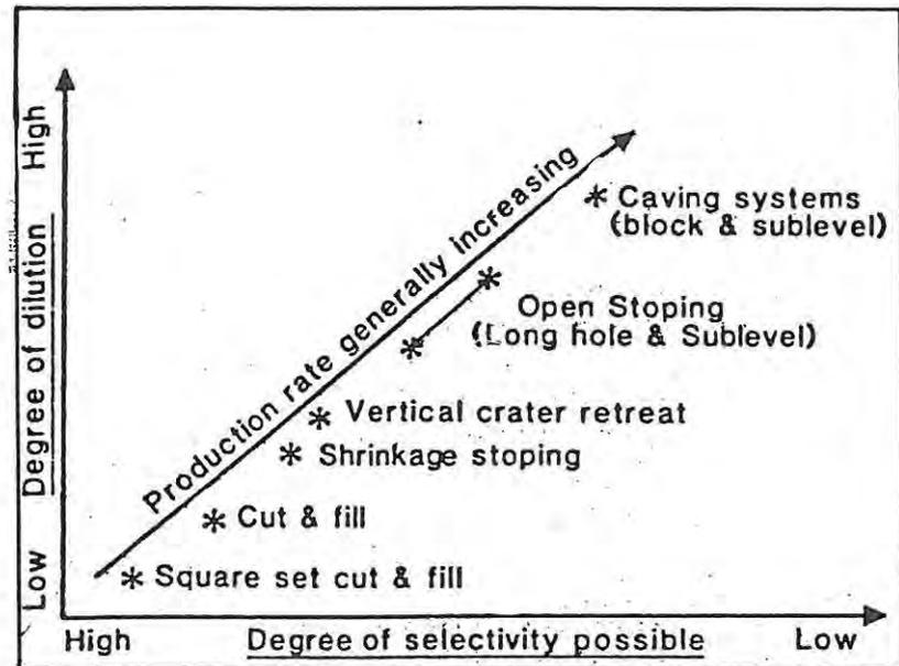
FIG B-7 THE DEGREE OF DILUTION ASSOCIATED WITH VARIOUS MINING METHODS (BUJTOR ET AL.1983)
