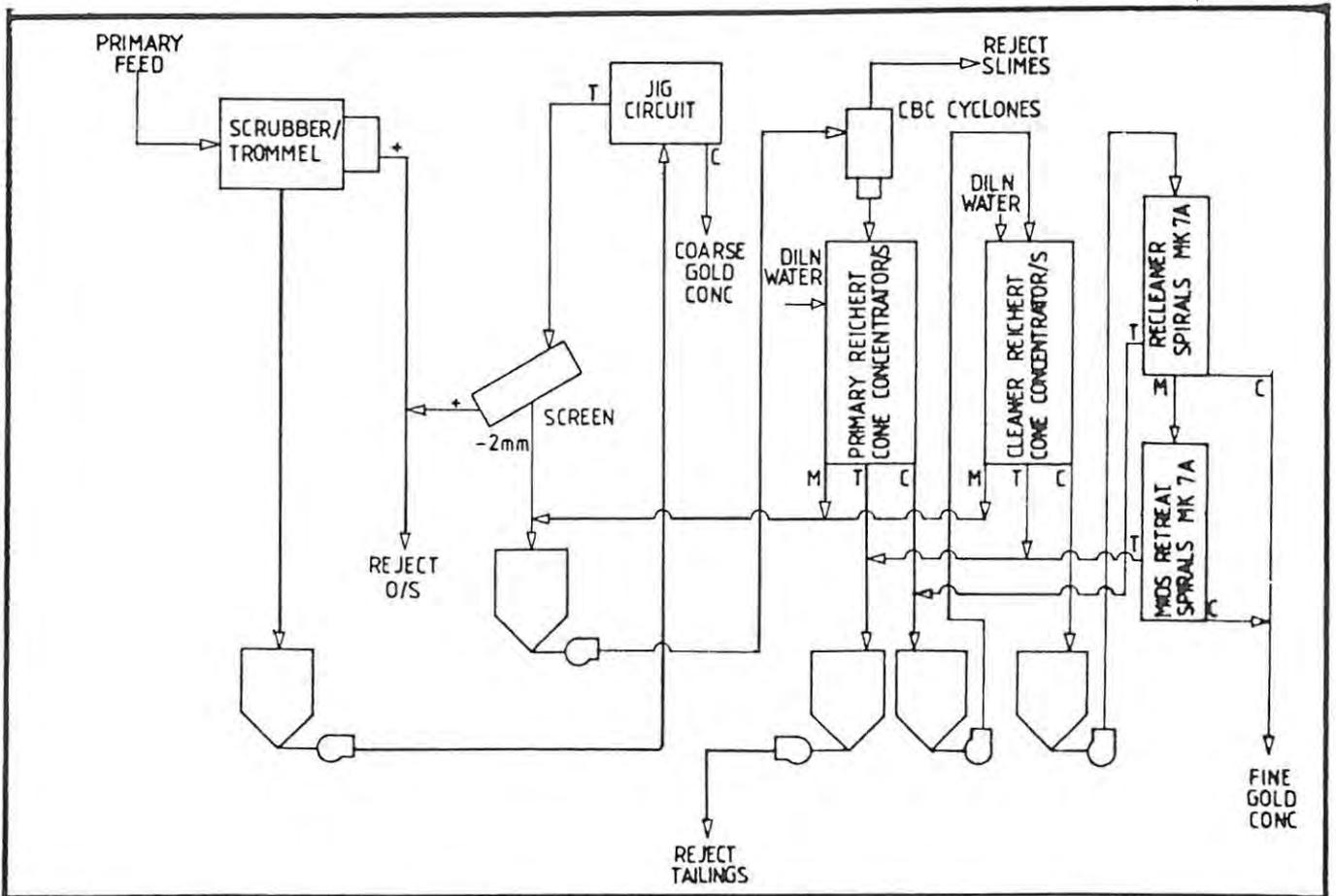
FIG C-4 CONCEPTUAL FLOW SHEET FOR ALLUVIAL FINE GOLD RECOVERY (RICHARDS ET AL. 1984)
