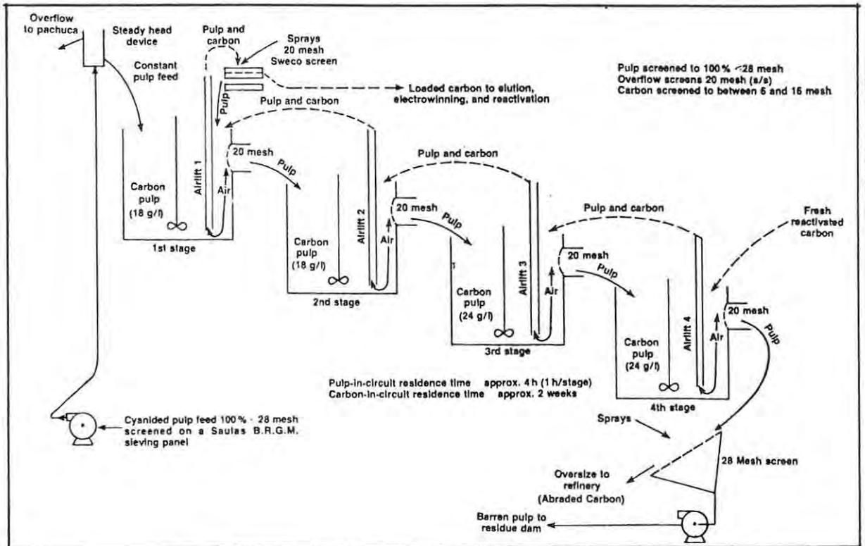
FIG C-7 CONCEPTUAL FLOW SHEET FOR A CIP CIRCUIT (LAXEN ET AL. 1979)
