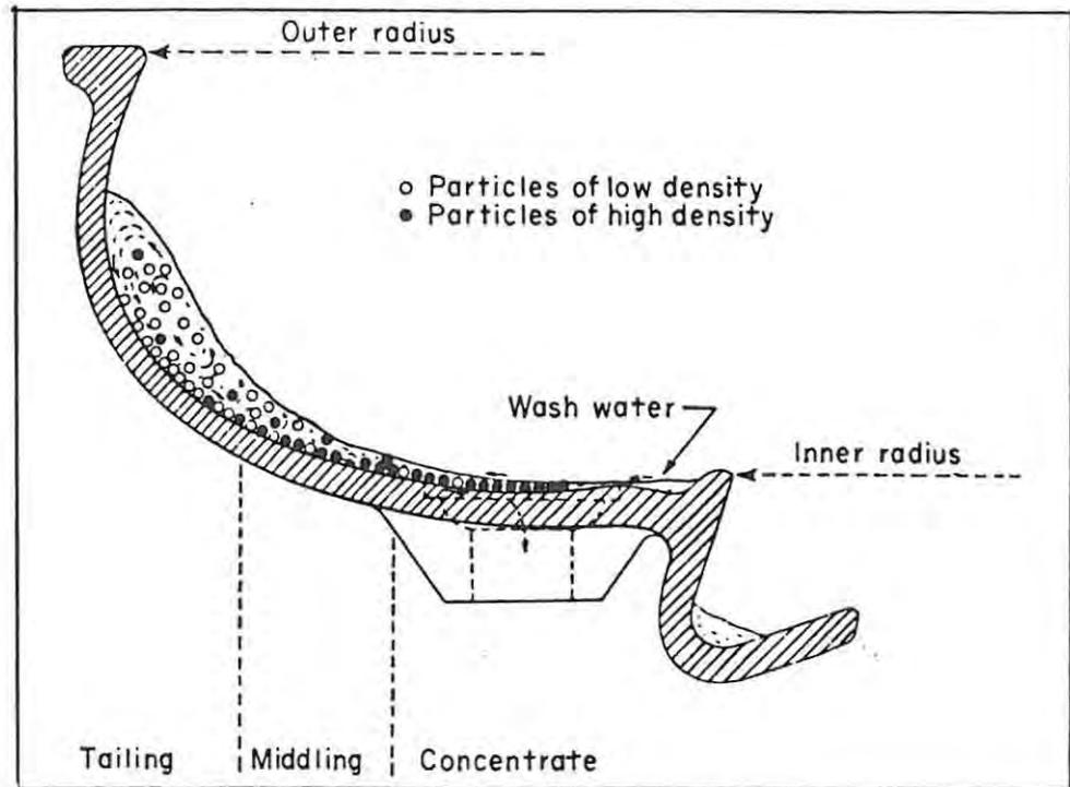
FIG C-2 CROSS SECTION OF A SPIRAL STREAM (WILLS 1979)
