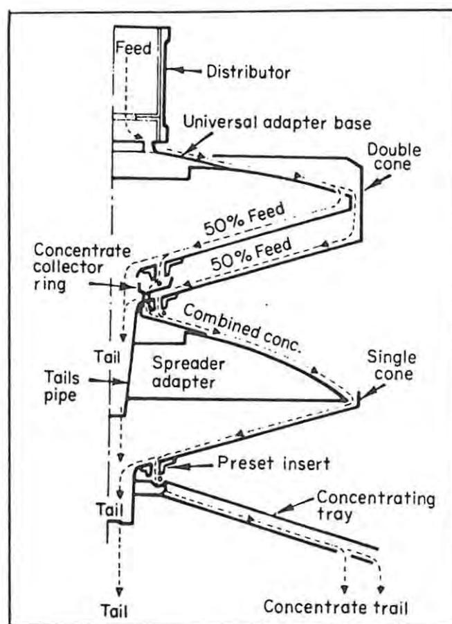
FIG C-1 CROSS SECTION THROUGH REICHERT CONE CONCENTRATOR SYSTEM. (WILLS 1979)
