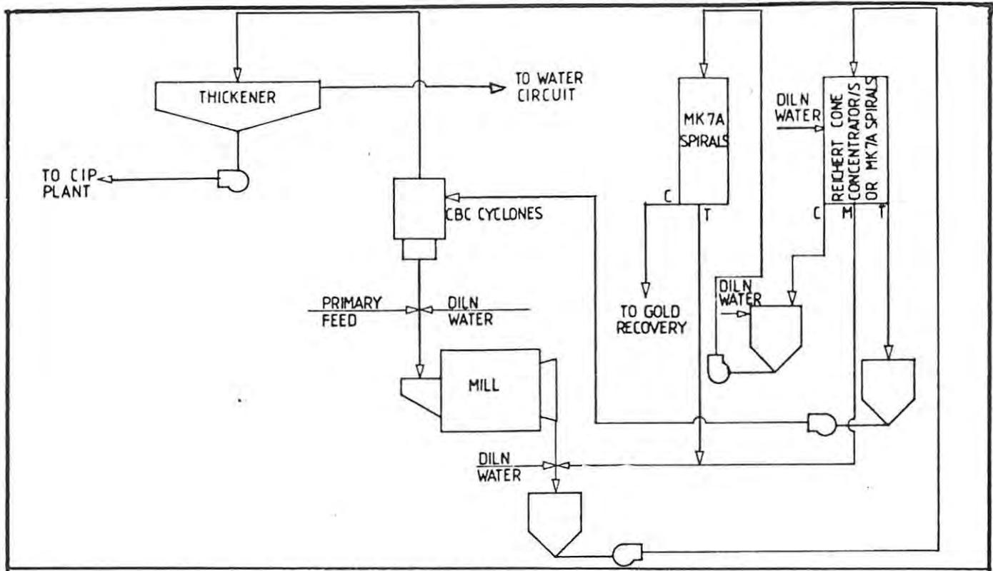
FIG C-5 CONCEPTUAL FLOW SHEET FOR GRAVITY CONCENTRATION IN A GOLD GRINDING CIRCUIT (RICHARDS ET AL. 1984)
