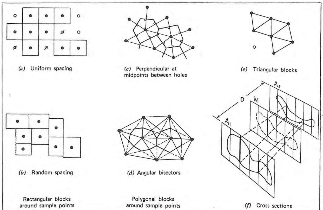
FIG B-1 GEOMETRIC PATTERNS USED FOR ORE RESERVE CALCULATIONS (PETERS 1987)
