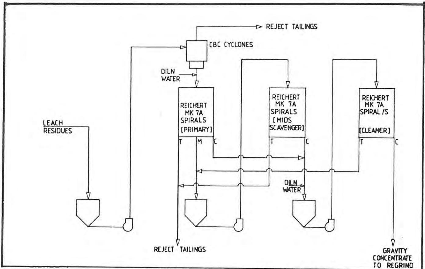
FIG C-6 CONCEPTUAL FLOW SHEET FOR GOLD LEACH PLANT TAILINGS SCAVENGING BY GRAVITY CONCENTRATION (RICHARDS ET AL. 1984)
