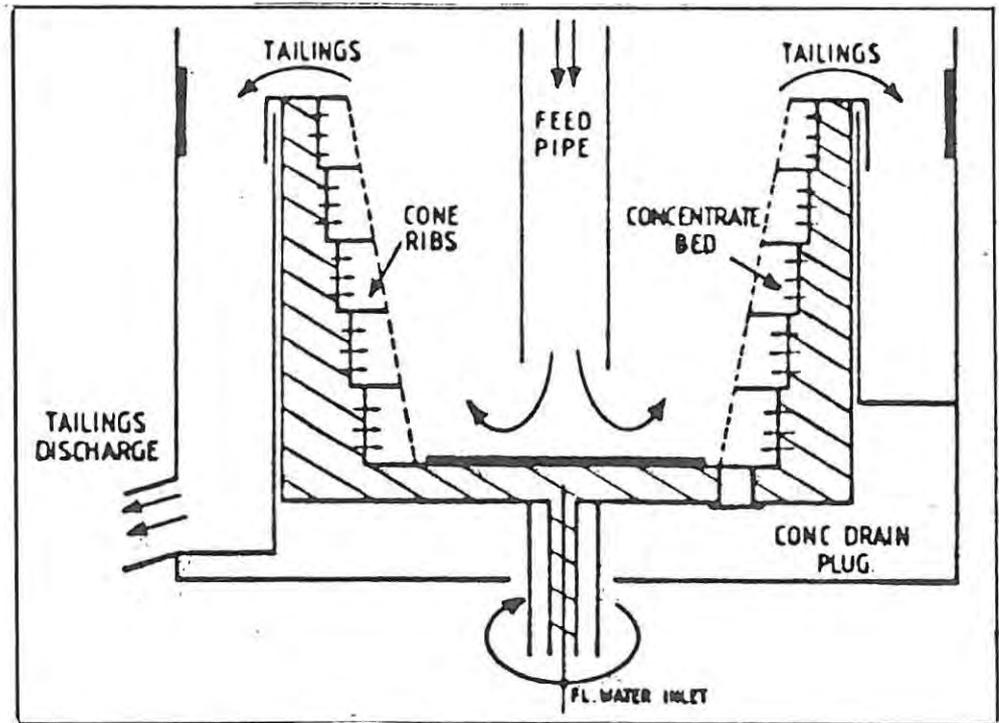
FIG C-3 CROSS SECTION OF A KNELSON CONCENTRATOR (HARRIS 1989)
