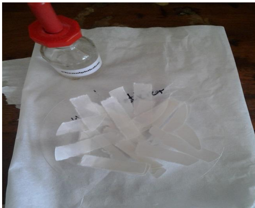
Fig. 3.15a: Filter paper strips impregnated with phenolphthalein solution indicator
