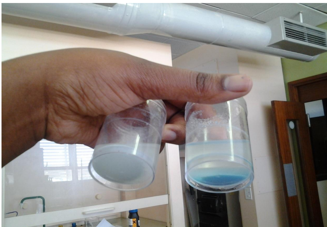
Fig. 3.21: Visual observation of biodiesel samples tested for the presence of water using anhydrous copper sulphate
