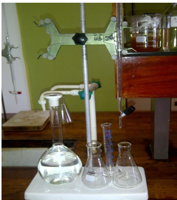
Fig. 1.6: Apparatus for the soap test kit (titration)
