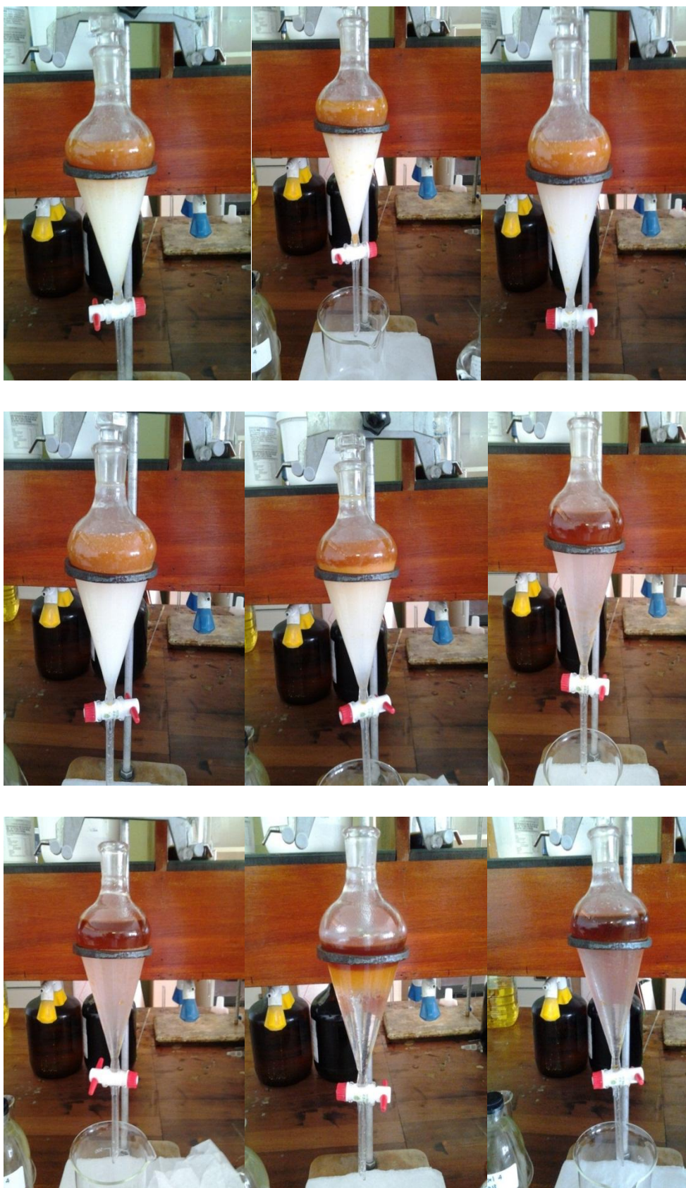
Fig. 3.8: Biodiesel soap test validation. The visual observation of the change in the waste water after each wash.
