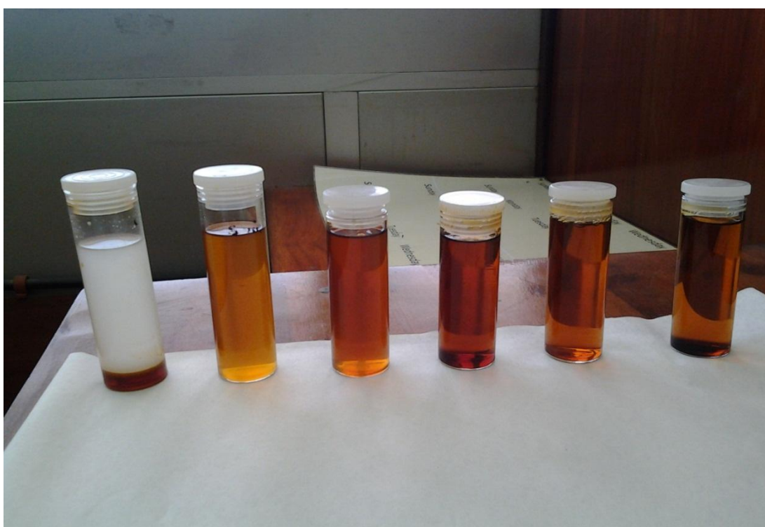
Fig. 3.4: 3/27 Test kit validation (used oil). Left to right are samples taken at different time intervals from 0-60 minutes.
