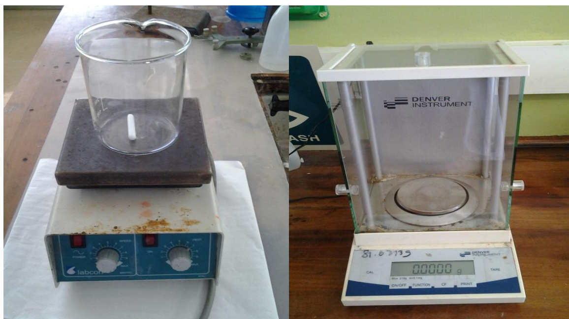
Fig. 1.3: Instrumentation for weight heat weight (WHW) water test kit
