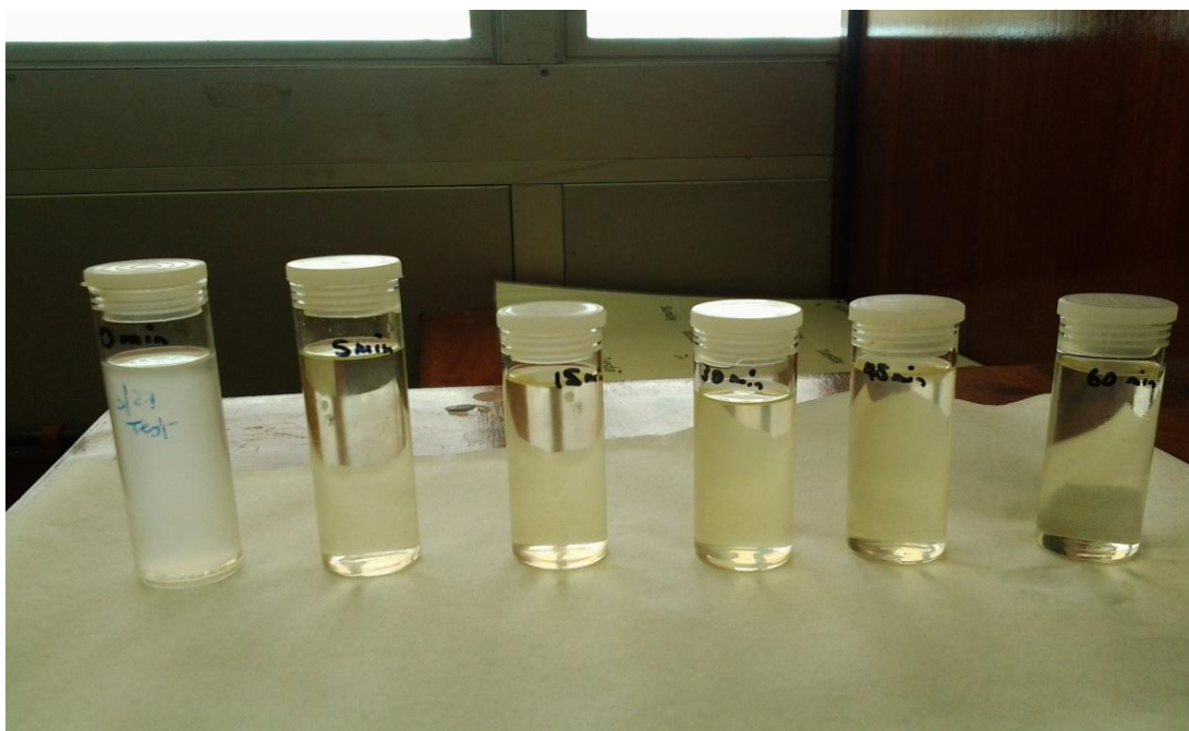
Fig. 3.3: 3/27 Test kit validation (pure oil). Left to right are samples taken at different time intervals from 0-60 minutes.
