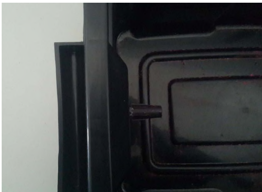
Figure 2.6: Position of black PVC pipe (highlighted by the arrow) on the interior of the flight chamber ensuring moths do not leave the chamber by crawling.
