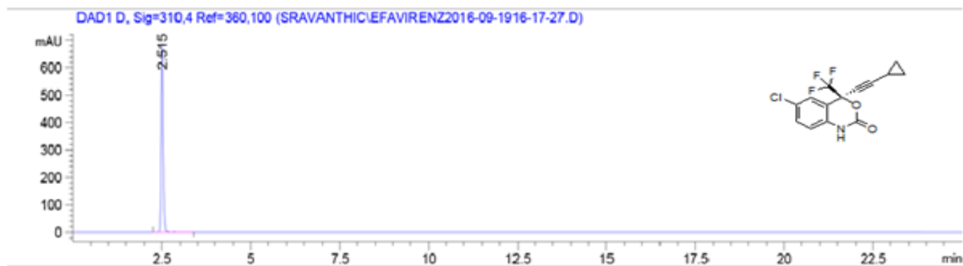
Chiral HPLC chromatogram of 6-chloro-2-(4-cyclopropylethynyl)-4-(trifluoromethyl)-1 H -benzo[ d ][1,3] oxazin-2-(4 H )-one 8
