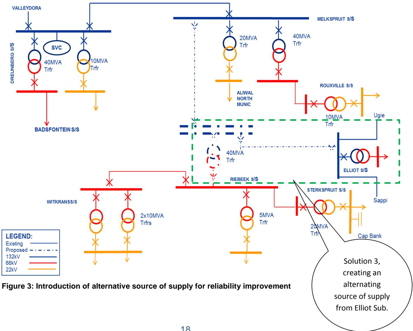
Figure 3: Introduction of alternative source of supply for reliability improvement
