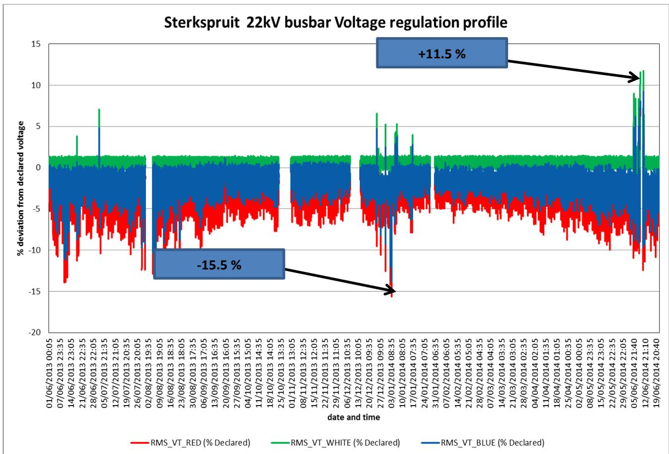
Figure 24: Voltage profile of Sterkspruit 22kV Busbar (Period June 2013 – June 2014)
