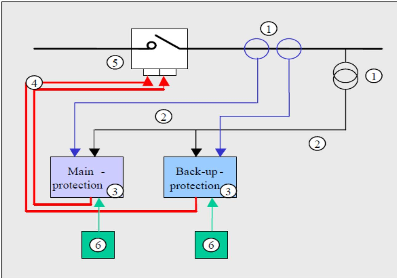
Figure 15: System components of the distance protection device
