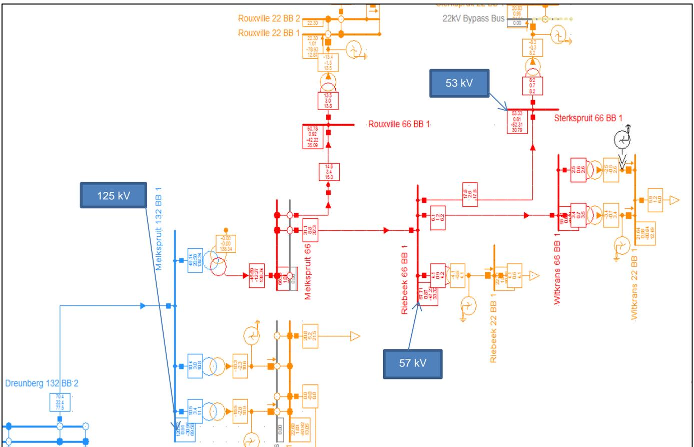
Figure 37: PowerFactory Results for the loading of Aliwal North Sector network
