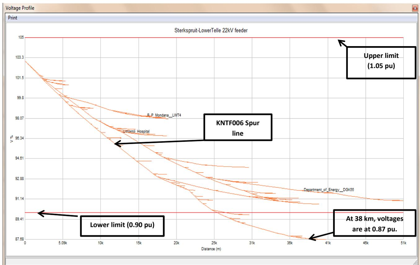
Figure 44: Voltage Profile for LowerTelle 22 kV line simulated from Retic Master under normal conditions.
