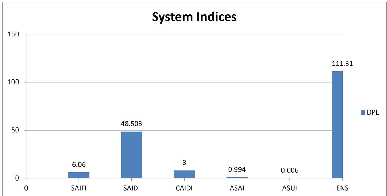
Figure 31: DigSilent (PowerFactory) 66 kV reliability graphical representation results
