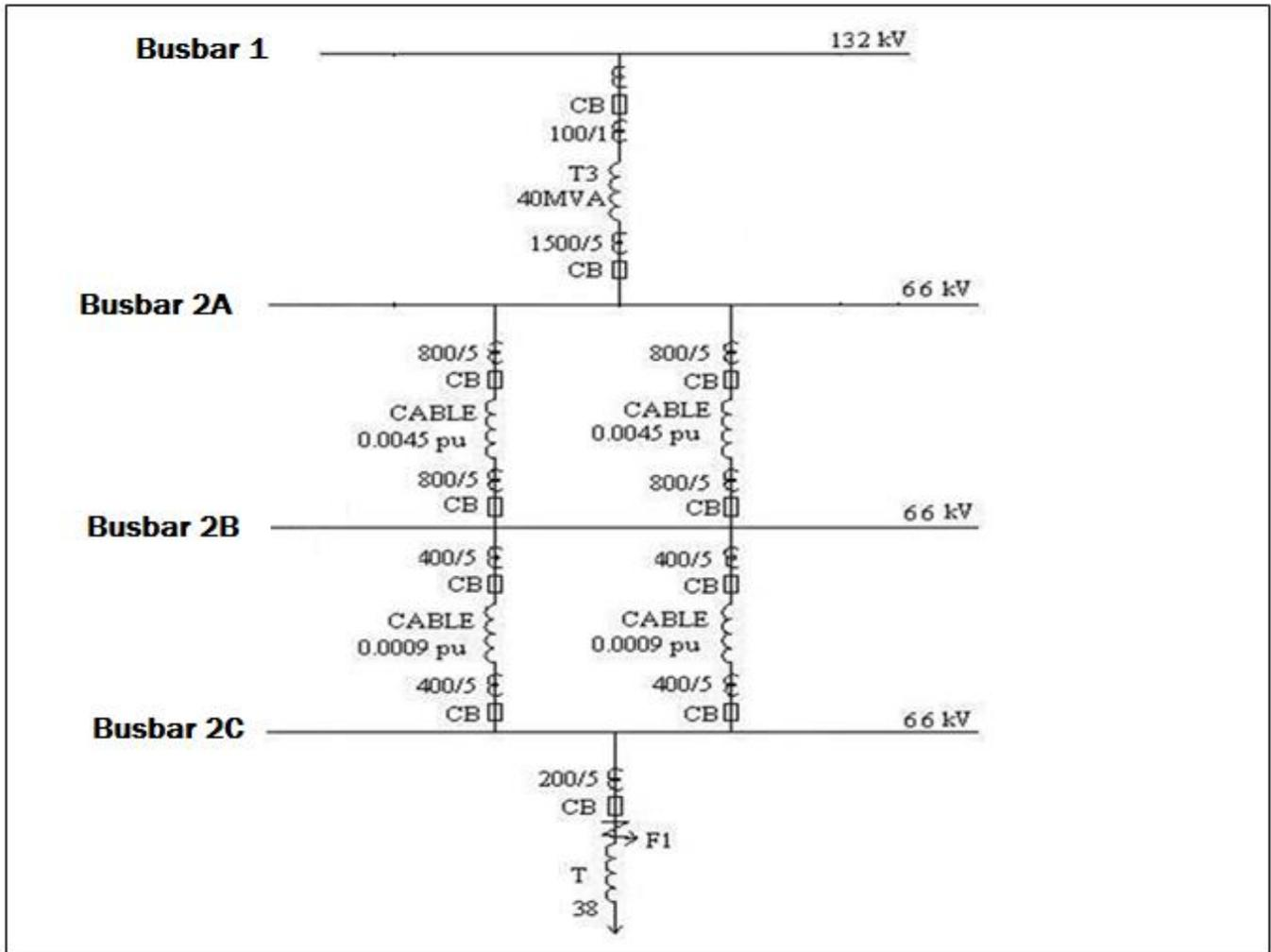
**Figure 56: Relay Co-ordination for Melkspruit Substation**
