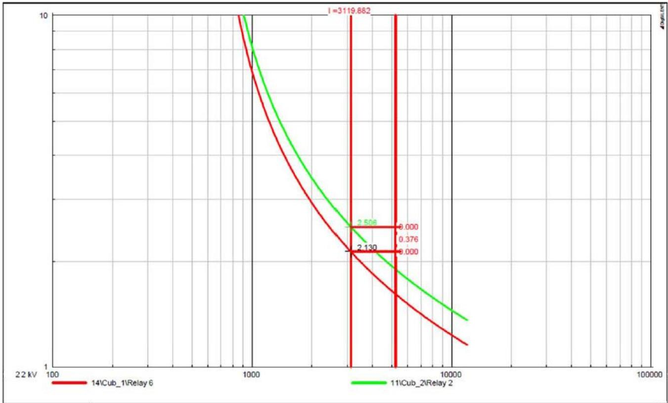
**Figure 63: Relay Coordination for Single phase to ground faults**
