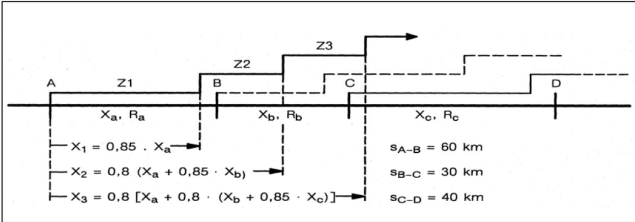
Figure 16: Protection zones of the distance protection at bus bar A
