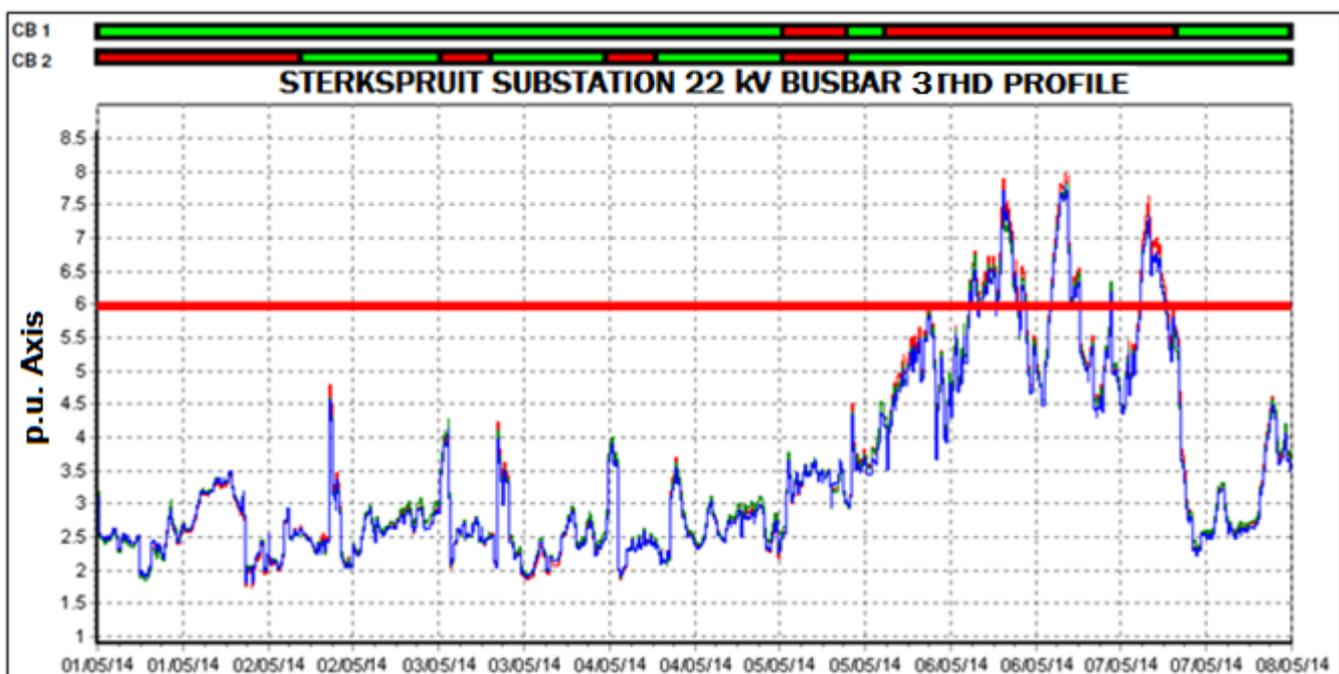
Figure 52: 3<sup>rd</sup> Harmonic in 22 kV busbar number 2
