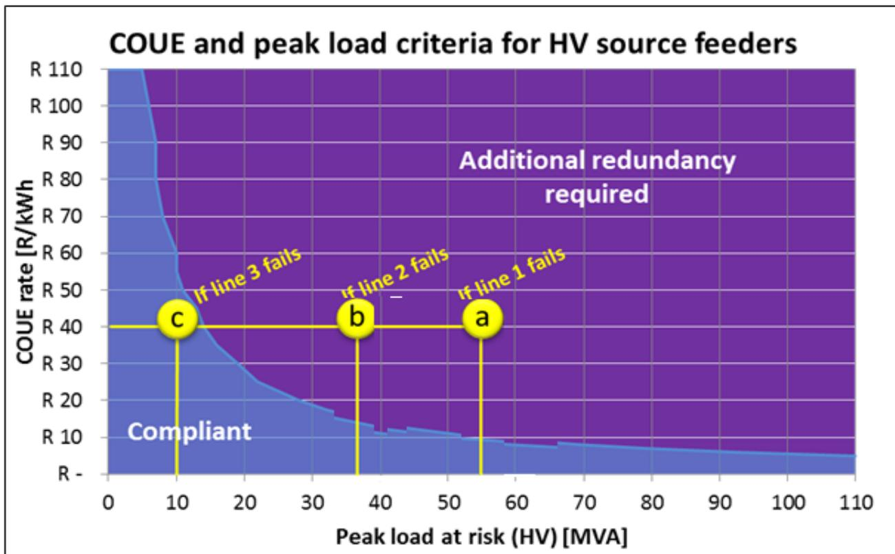
Figure 67: Calculating load at risk – radial network
