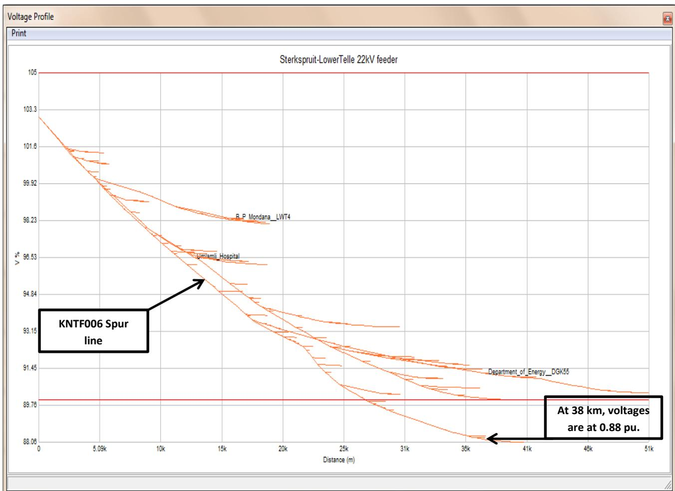
Figure 46: Voltage Profile Improvement using Shunt Capacitor.
