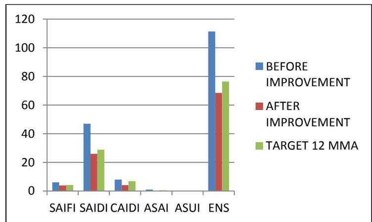
Figure8A: Aliwal reliability performance after network improvement all voltage levels i.e. 132/66/22 kV in average.
