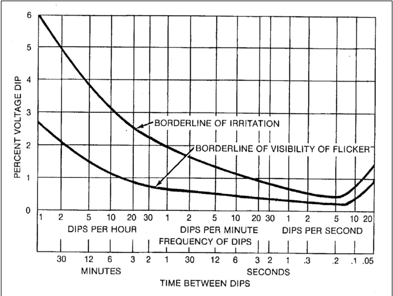
**Figure 40: Range of Observable and Objectionable Voltage Flicker versus Time.**
