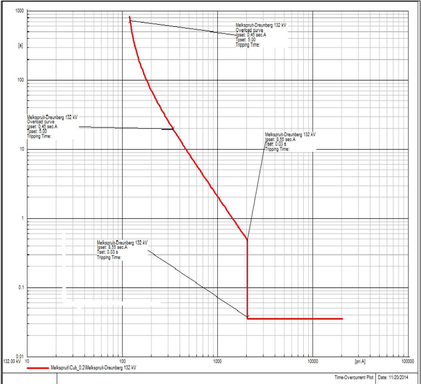
**Figure 59: Relay Co-ordination for Melkspruit Substation**
