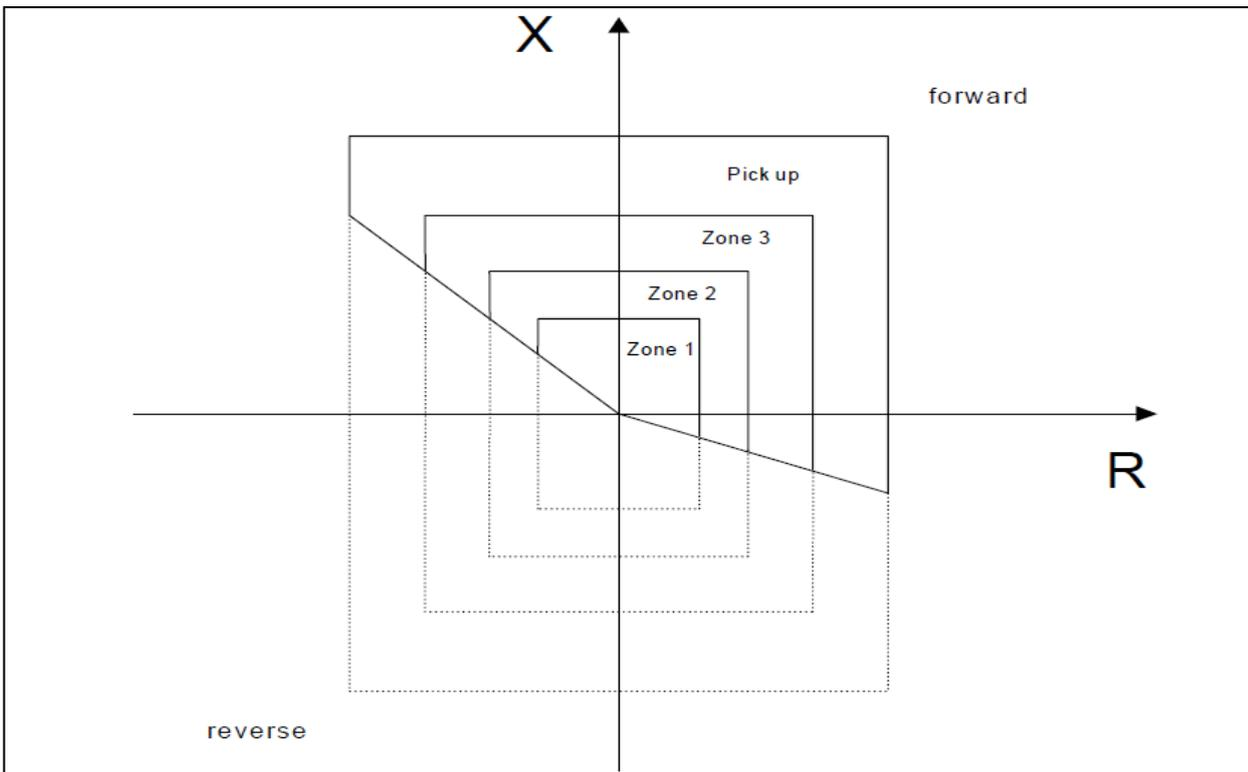
Figure 17: Tripping characteristics of a distance protection device
