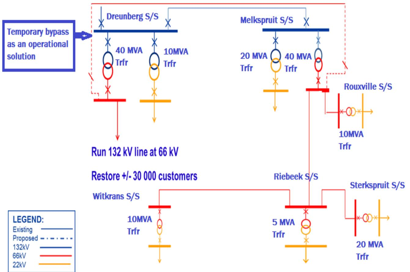
Figure 2: Operational Solution run 132 kV at 66 kV
