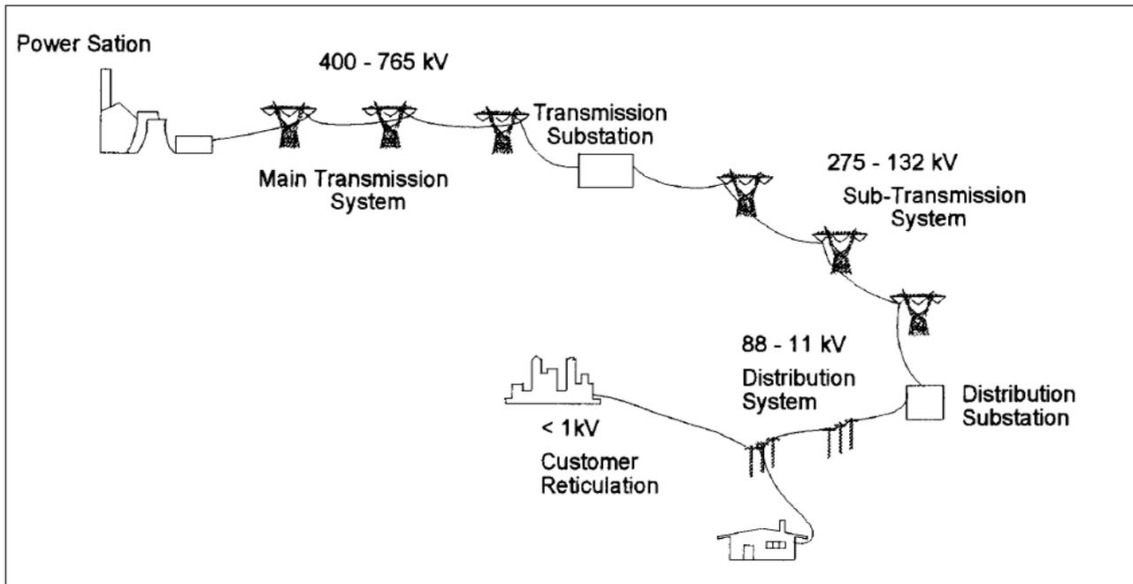
Figure 10: Typical power system representation [30]
