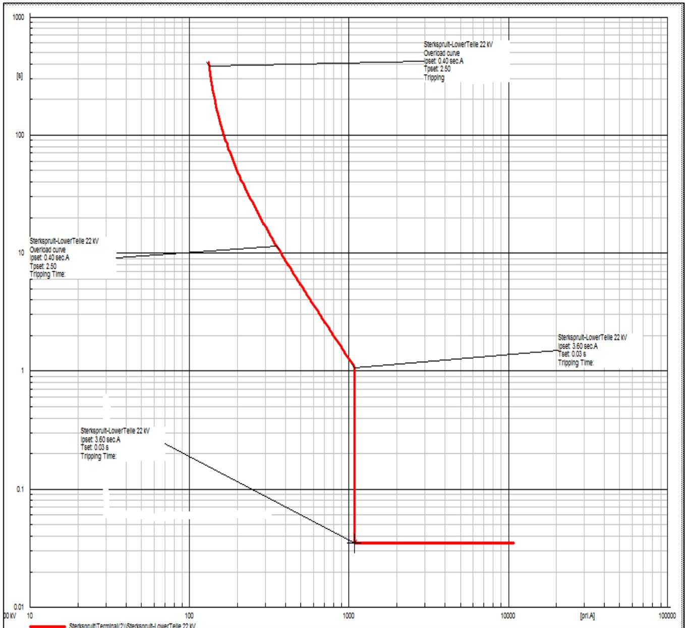
**Figure 61: Relay Co-ordination for Melkspruit Substation**
