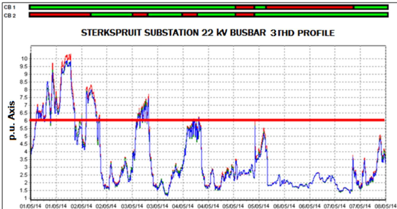
Figure 51: 3<sup>rd</sup> Harmonic in 22 kV Busbar number 1
