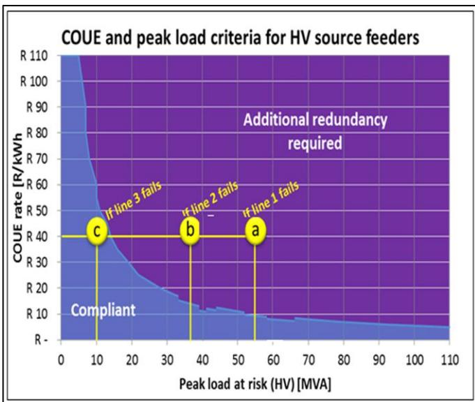
Figure 7: Calculating load at risk – radial network [3]
