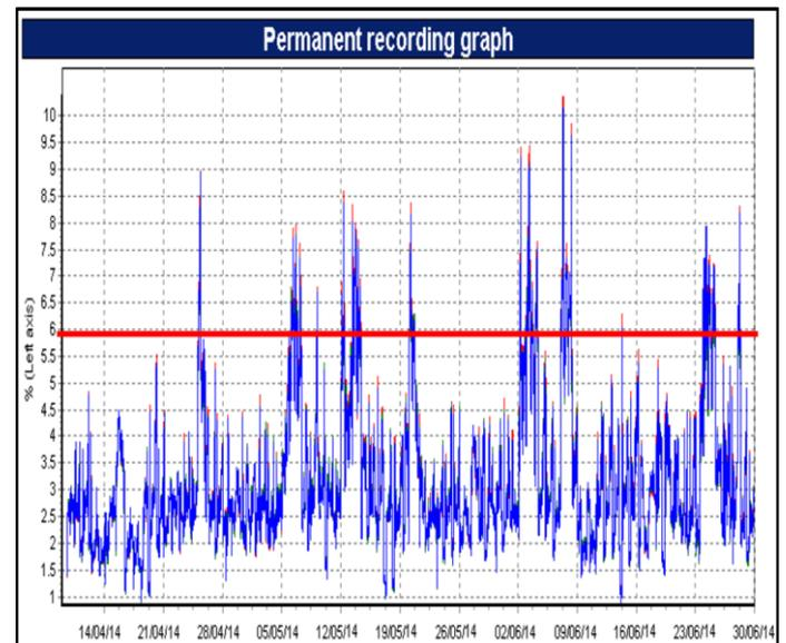
Figure 14: 3rd Harmonic in MV busbar 2.
