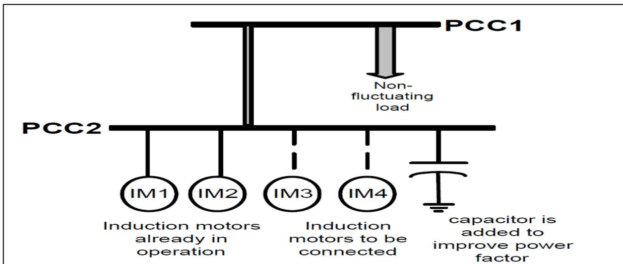
Figure 12 Shunt Capacitor Bank connected series with Motor Loads at PCC2.
