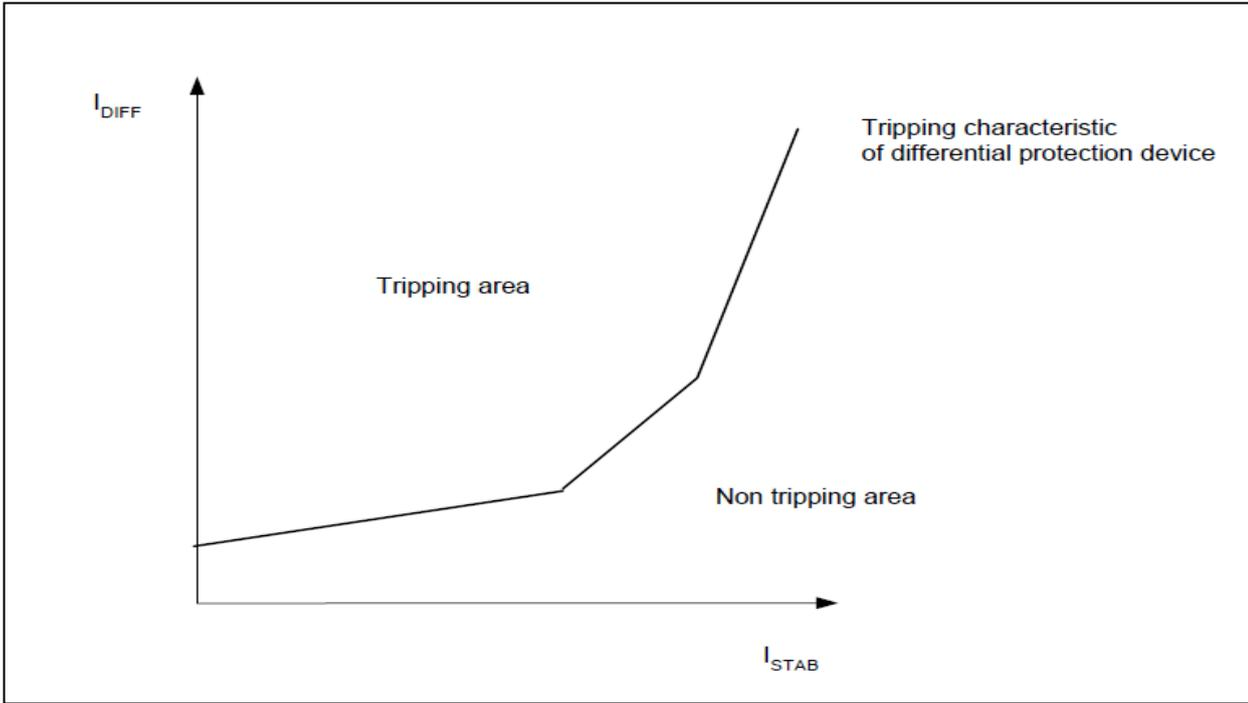
**Figure 19: Tripping of differential protection**
