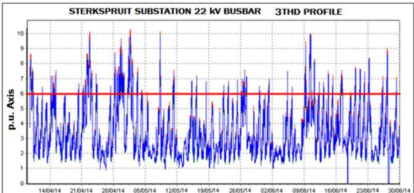
Figure 48: 3<sup>rd</sup> Harmonic in MV busbar 1.
