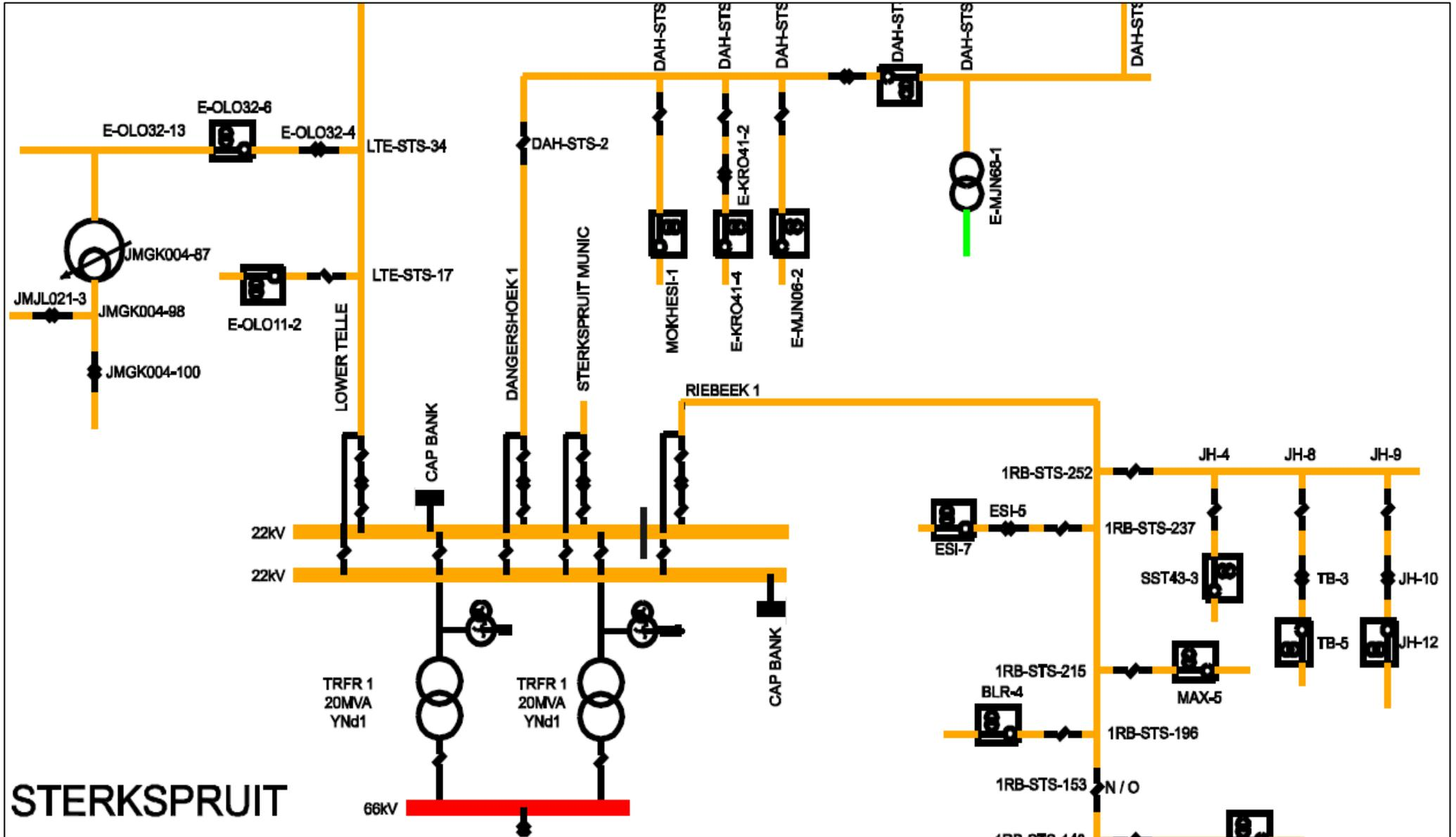
Figure 50: Single Diagram of 66/22 kV Sterkspruit Substation.
