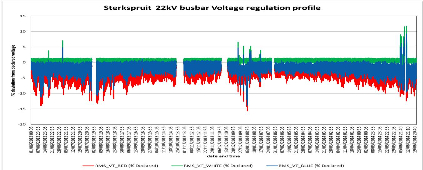
**Figure 38: Voltage Profile for unbalanced.**
