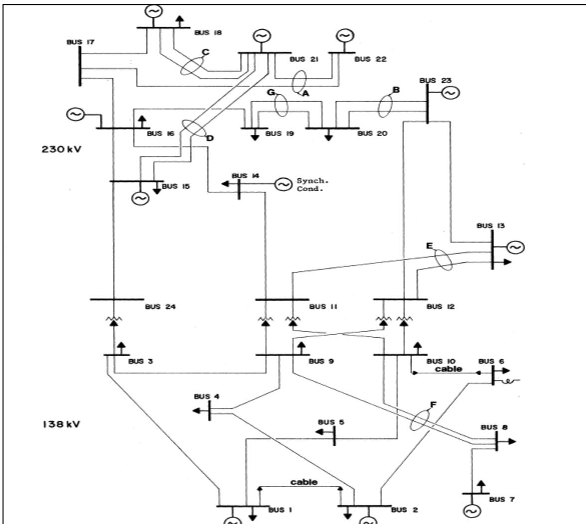
Figure 11: IEEE Reliability test system [33]
