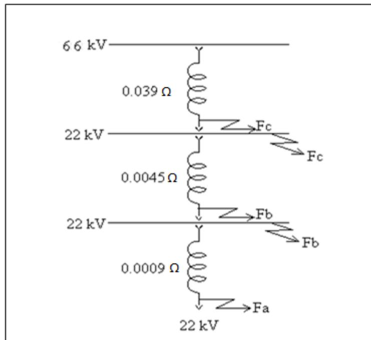
Figure 54: Impedance Diagram for Faults on 22 kV bus on Sterkspruit Substation
