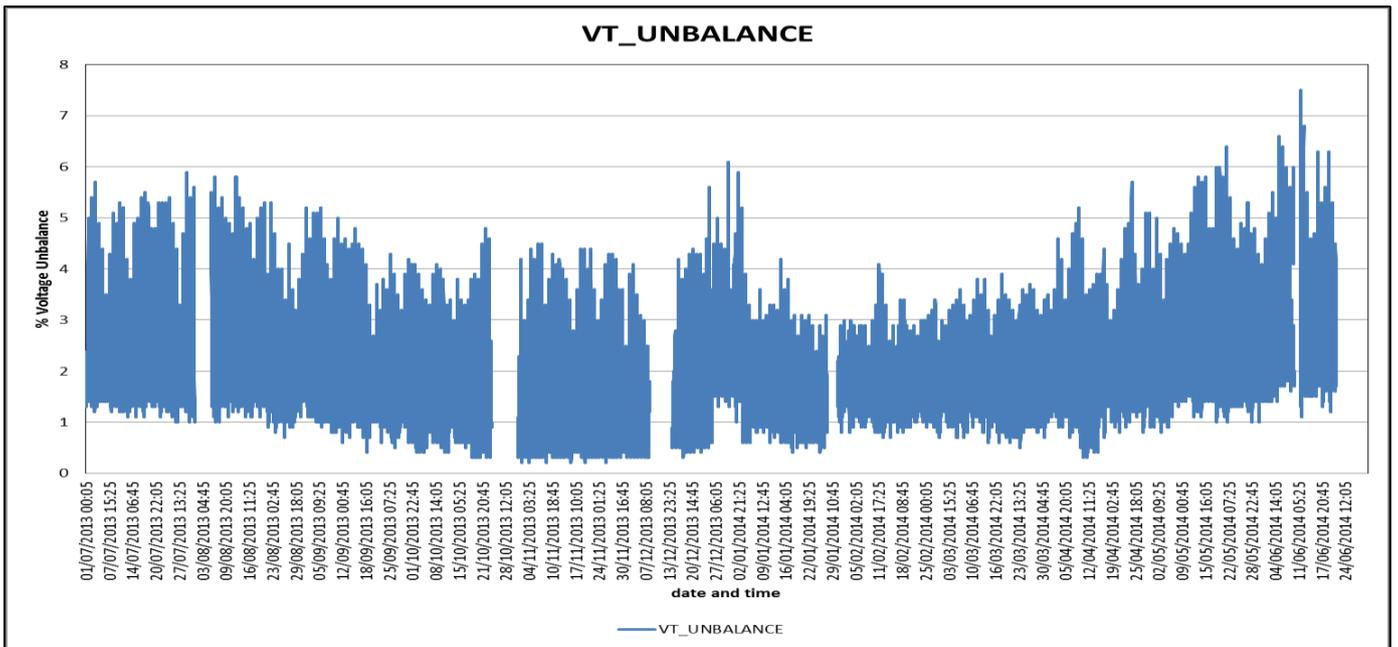
Figure 9: Voltage Profile for unbalanced
