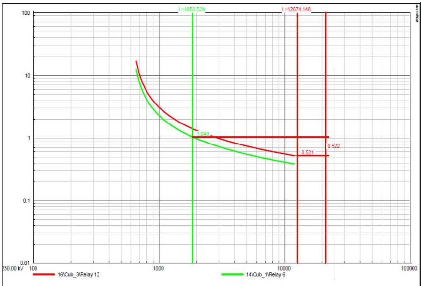
**Figure 64: Performance of Relay Coordination at Riebeek Substation**
