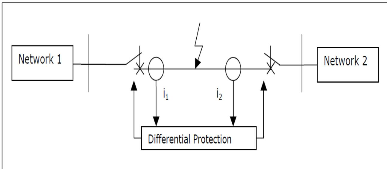
Figure 18: Functional principle of differential protection
