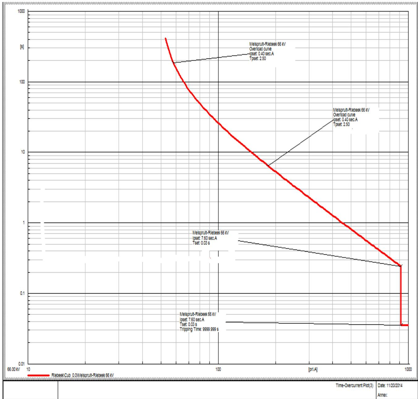
**Figure 57: Relay Co-ordination for Melkspruit Substation**
