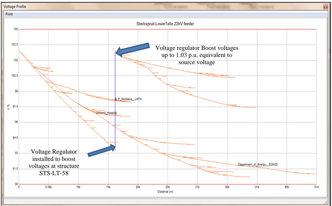
Figure 15: Voltage Profile Improvement using Voltage Regulator.
