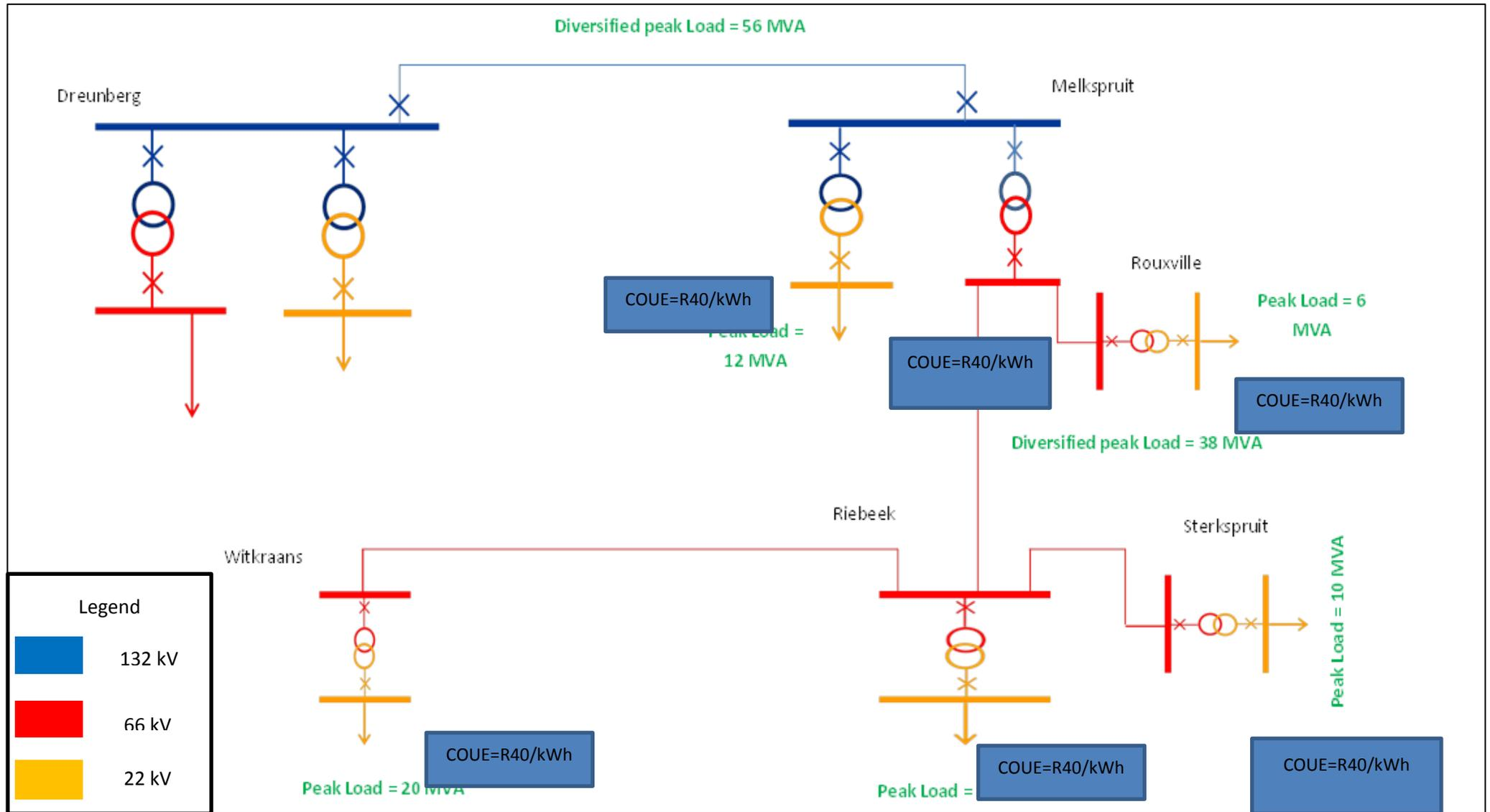
Figure 66: Calculating load at risk – radial network
