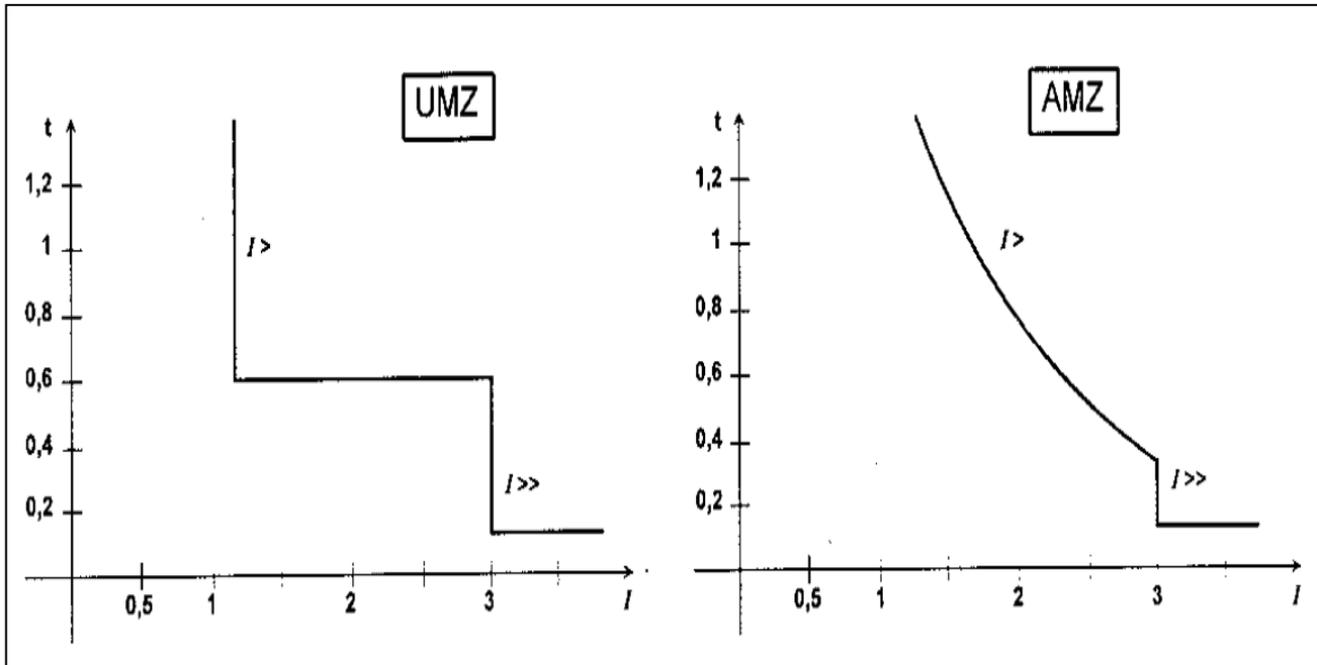
Figure 14: Types of over-current protection
