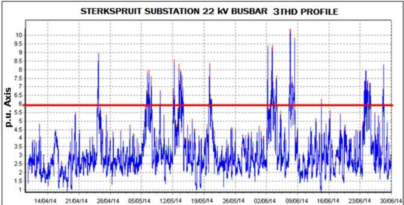
**Figure 49: 3<sup>rd</sup> Harmonic in MV busbar 2.**
