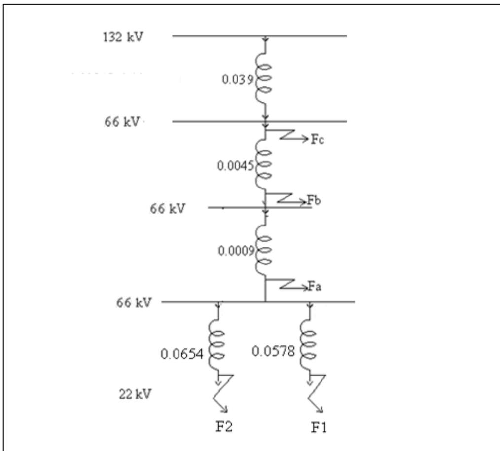
Figure 55: Impedance Diagram of Melkspruit Substation
