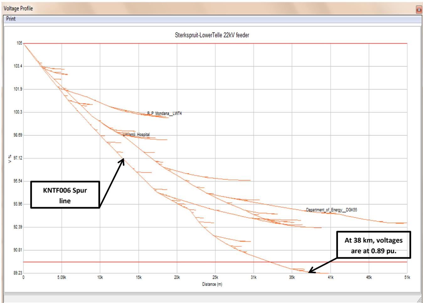
Figure 45: Voltage Profile Improvement using On-Load Tap Changer.
