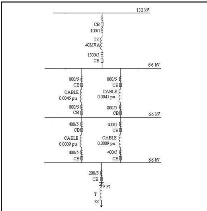
Figure 16: Impedance Diagram for Faults on 22 kV bus on Sterkspruit Substation
