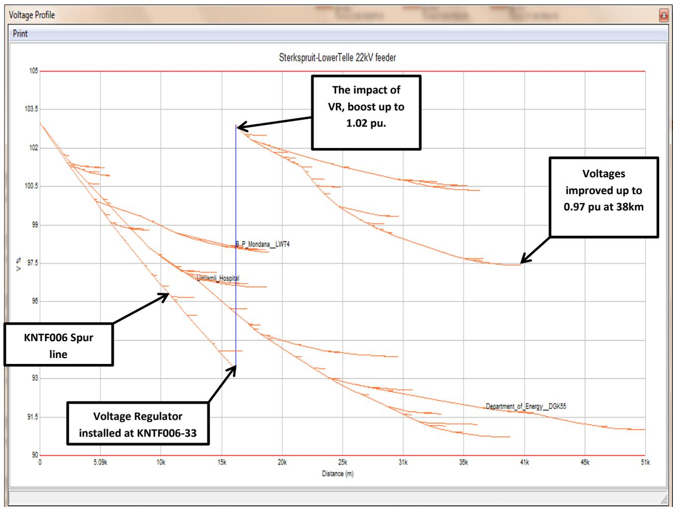
Figure 47: Voltage Profile Improvement using Voltage Regulator.
