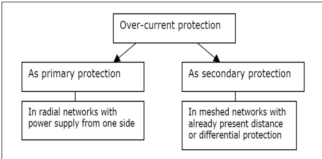
Figure 13: Implementation of over-current protection
