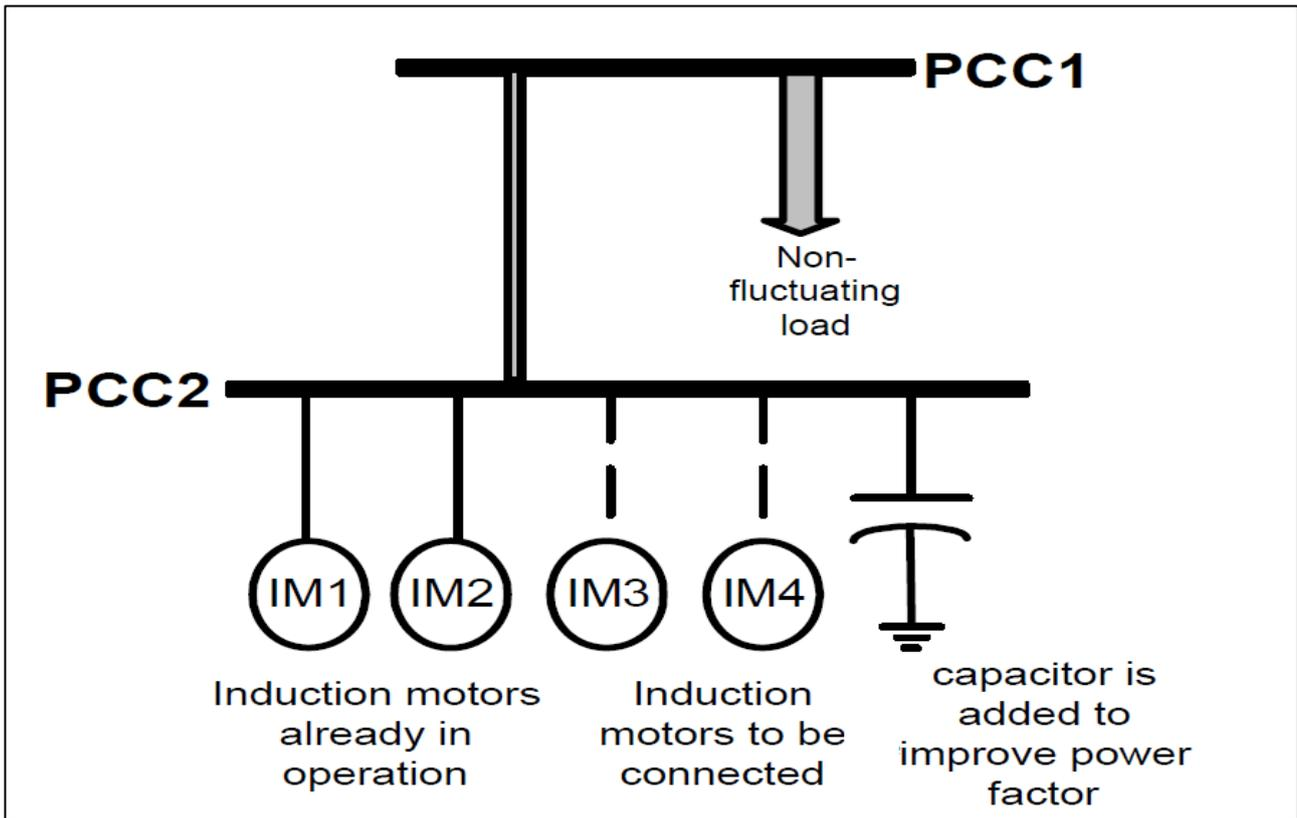
Figure 41: Shunt Capacitor Bank connected series with Motor Loads at PCC2 (Point of Common Coupling)
