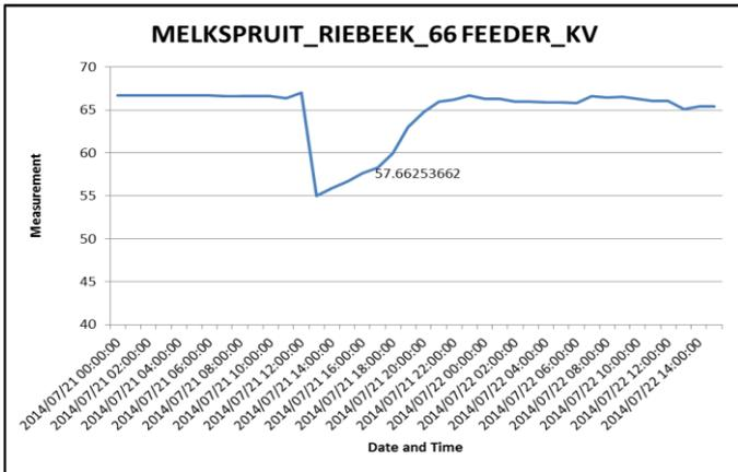
Figure 12: Voltage Profile with Voltage DIPS
