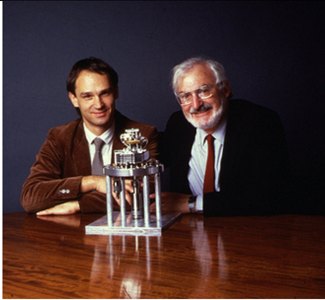
First Scanning Tunneling Microscope (STM) ( http://www.research.ibm.com/articles/heinrich-rohrer.shtml )
