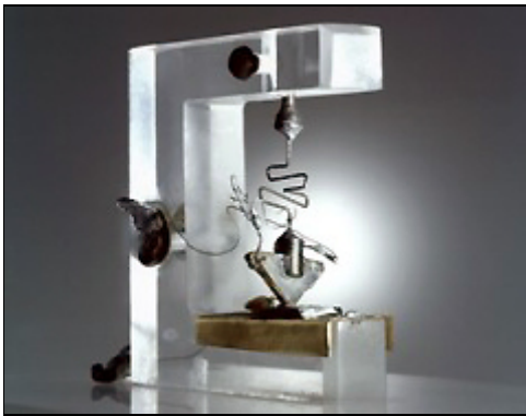
1947 transistor, Bell Labs
