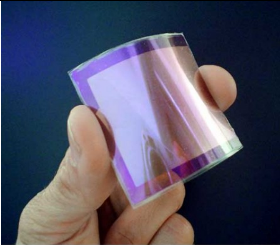
New solar panel films incorporate nanoparticles to create lightweight, flexible solar cells. (Image courtesy of Nanosys)
