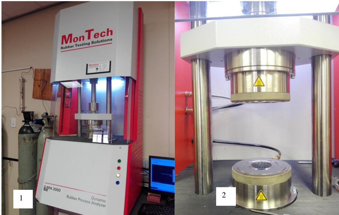
**Figure 2.12:** 1) Dynamic moving die rheometer 2) shows upper and lower die systems.
