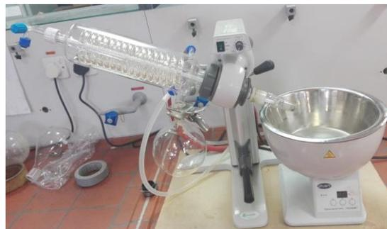
**Figure 2.18:** Rotary evaporator, RE300.
