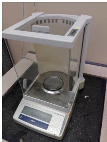
**Figure 2.9a:** Mettler Toledo weighing balance (AB204-S)
