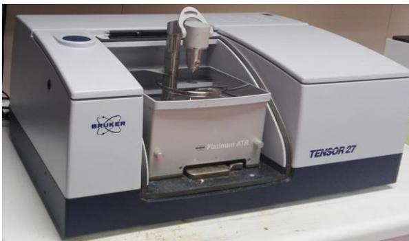
**Figure 2.20:** FTIR spectrophotometer, Tensor 27.
