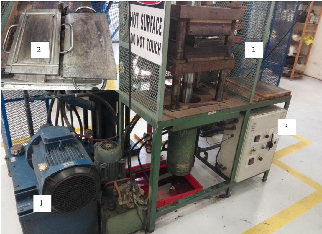
**Figure 2.13:** Cure press used for compression moulding. Indicated is the 1) motor for the hydraulic system, 2) mould plates, and 3) temperature control unit.
