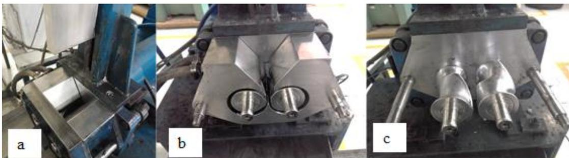
**Figure 2.10a:** Banbury internal mixer a) chamber b) open chamber c) tangential mixing blades.
