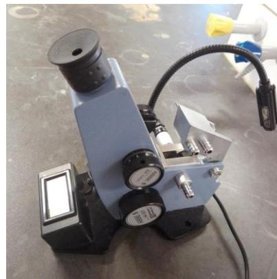
**Figure 2.15:** Refractometer for checking consistency in acetone/chloroform composition.
