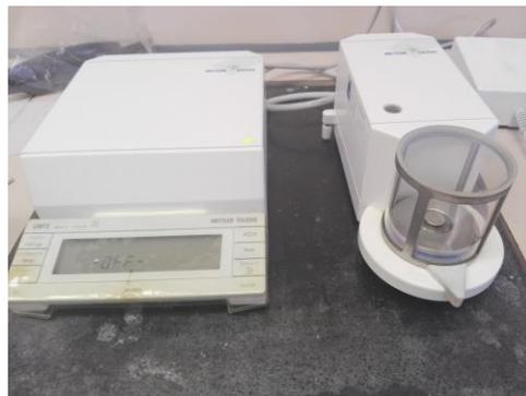
**Figure 2.9b:** Mettler Toledo microbalance (MX5 UMT2)
