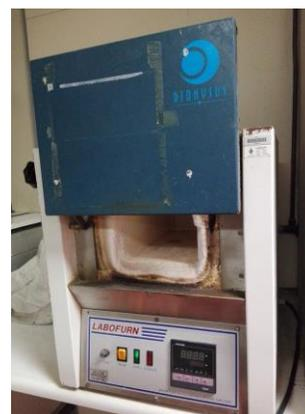
**Figure 2.19:** Muffle furnace used for GTR ash content
