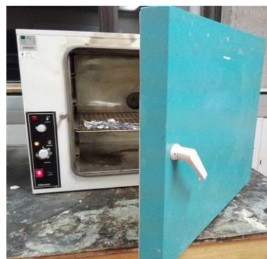
**Figure 2.17:** Forced air ventilation oven.
