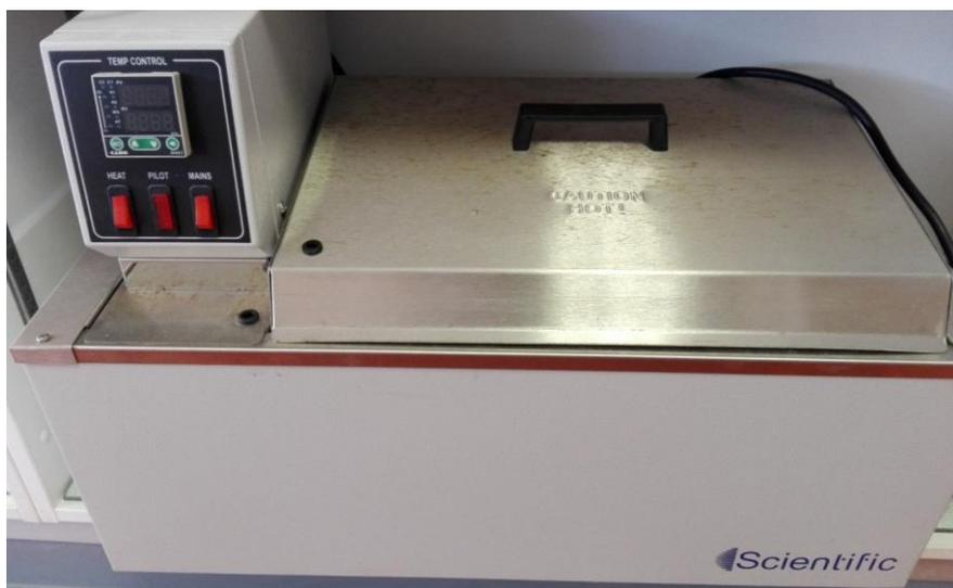
**Figure 2.14:** Water bath used for accelerated ageing.
