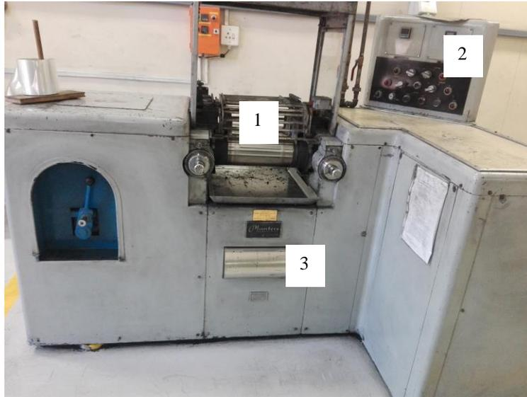
**Figure 2.11:** Two roll mill used for sheeting. Indicated are the 1) two rolls, 2) temperature and rotor speed regulator and 3) safety mechanism (trip switch).
