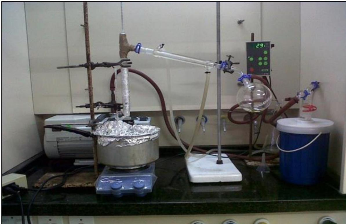
**Figure 2.3 Vacuum distillation set up for purification of PMD-citronellal acetal**
