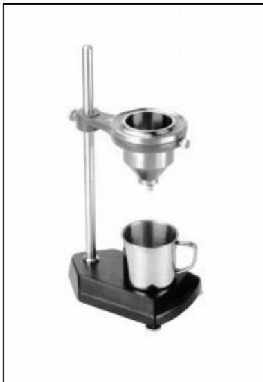
**Figure 4.4 Gardco viscosity cup and stand**
