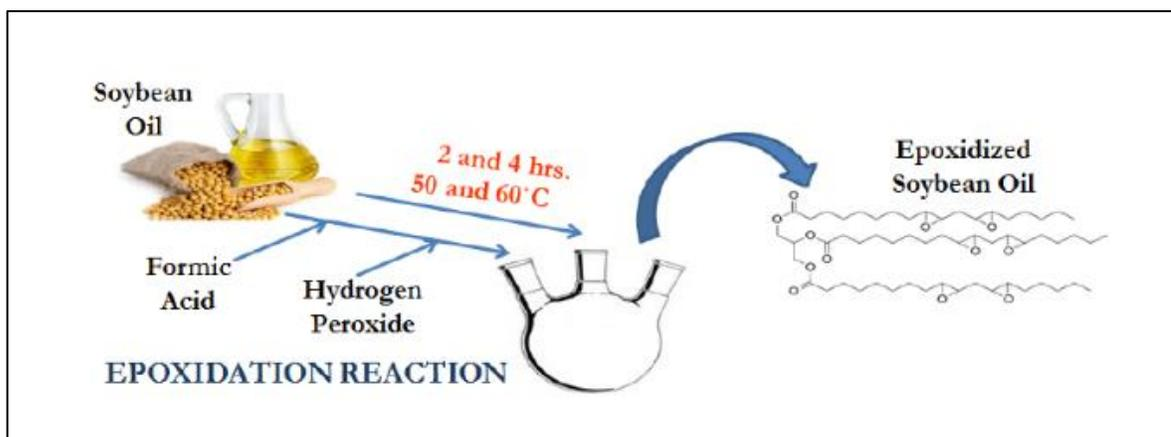
**Figure 1.8 Process for epoxidation of soybean oil [56]**
