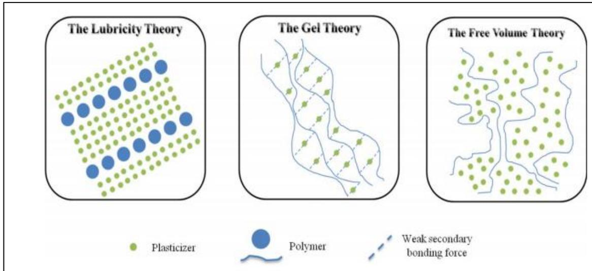
**Figure 1.2 Schematic illustration of plasticisation theories [18]**
