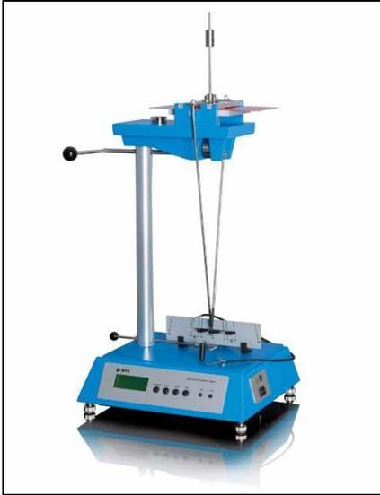
**Figure 4.2 König pendulum hardness tester [104]**
