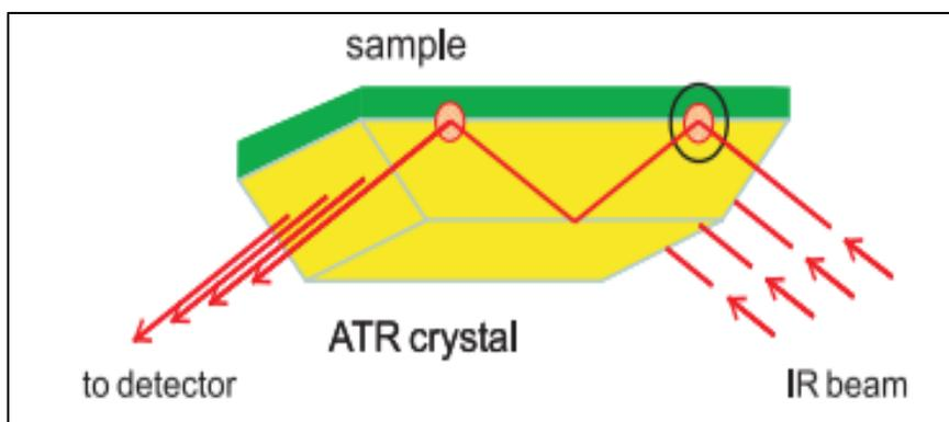
**Figure 5.1 Principle of ATR beams**
