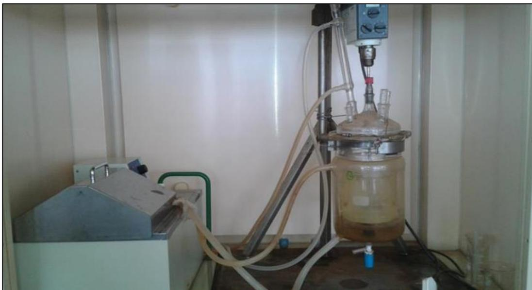
**Figure 2.2 Double-walled glass reactor used to synthesize *p*-menthane-3,8-diol**
