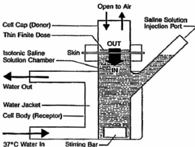
Figure 6.1 Schematic diagram of a modified Franz cell<sup>176</sup>
