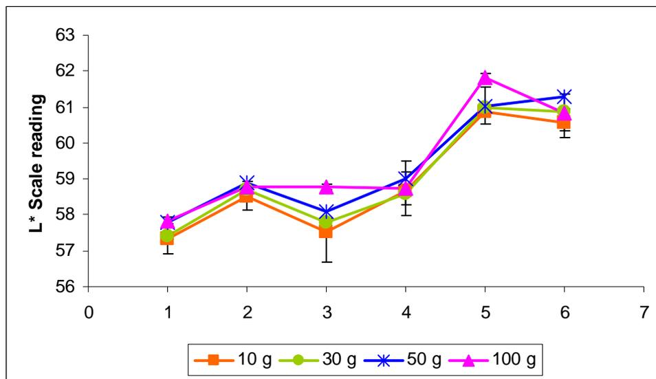
Figure 2.9 Effect of pressure on L\* reading – Operator 1
