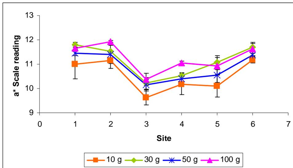
**Figure 2.8 Effect of pressure on a\* scale – Operator 2**
