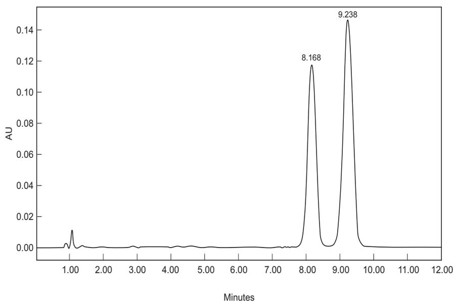
**Figure 4.3 Chromatogram of MF ( $t_R \sim 9.2$  min) and CP ( $t_R \sim 8.2$  min) at 238 nm**
