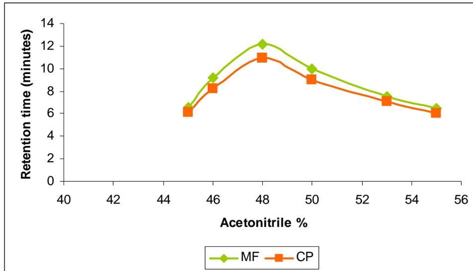
**Figure 4.4 Retention times versus percent acetonitrile in mobile phase**
