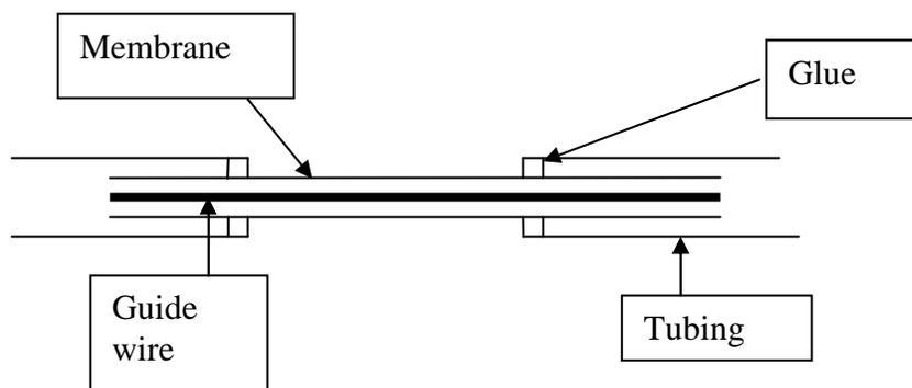
**Figure 5.1 Diagrammatic scheme of a linear microdialysis probe**
