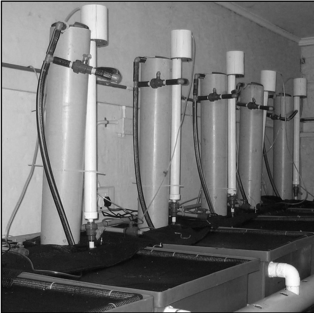
**Figure 2.2: Photograph of the independent re-circulating tanks used in experiments.**
