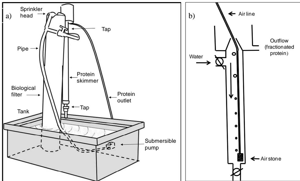
**Figure 2.1: a) Schematic of the independent re-circulating system and b) of the protein skimmer that was used during experiments**
