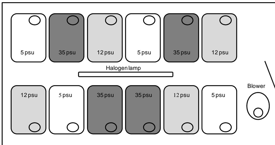
**Figure 2.2: Schematic overview of temperature controlled room and the placement of the independent re-circulating tanks with the randomly assigned salinities**
