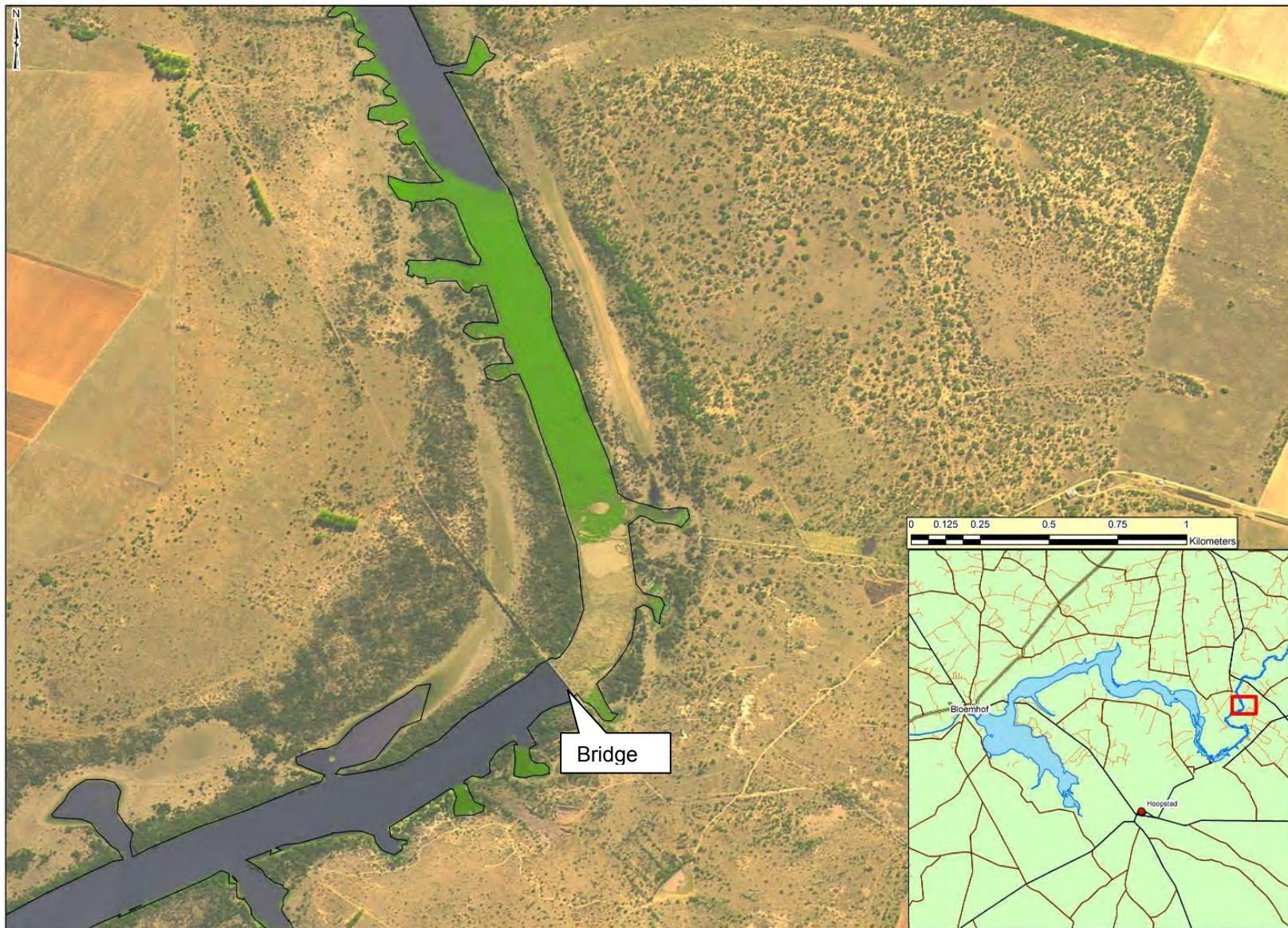
**Figure 1-4:** A 2009 SPOT V satellite image showing a 2km long infestation of water hyacinth that has resulted from backing up against a cable spanned across a bridge located at the top of Bloemhof Dam (insert depicting exact location of the bridge). The brown regions of the infestation, next to the bridge, have undergone herbicide treatment.
