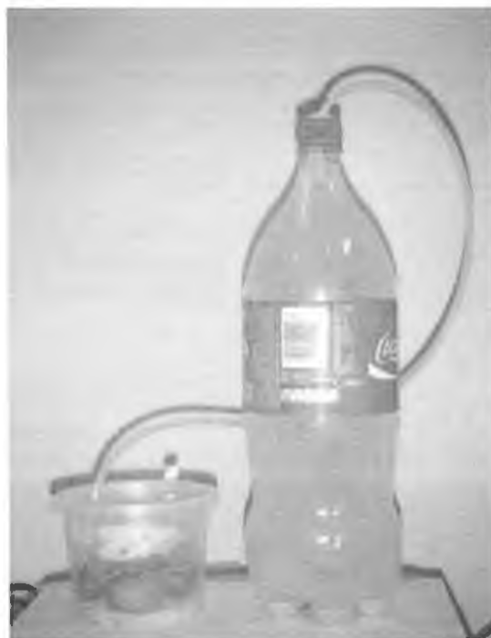
Figure 4.3: Carbon dioxide treatments were set up with a 2 litre bottle containing yeast, sugar and water. Carbon dioxide was fed into the container with the larvae and potatoes as shown.
