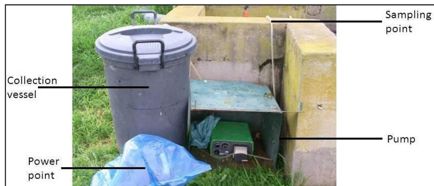
Figure 3 The setup of the collection of the composite sample abstracted over a 24 h period. An aliquot of the sample following mixing is then analysed in the laboratory for its physical, chemical and biological characteristics.
