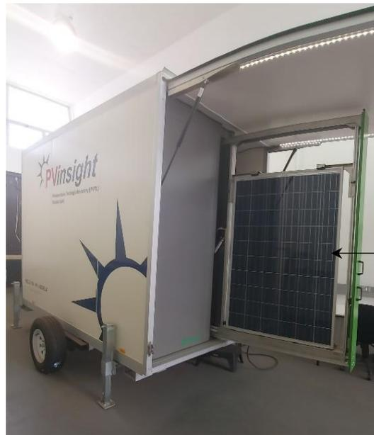
A PV module on a sliding door of the MBJ mobile Lab
