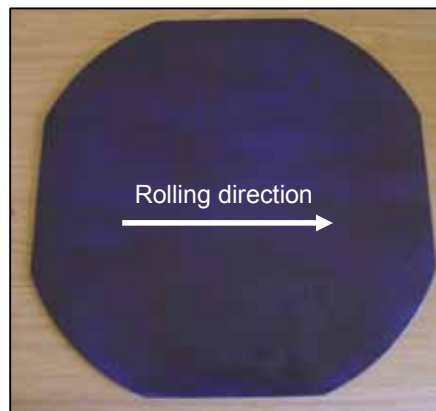
Figure 4.74: Blank of dual phase steel indicating rolling direction
