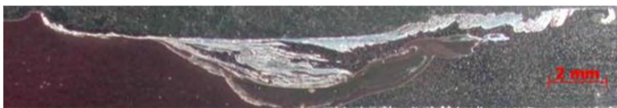
**Figure 4.5: Macro appearance of weld produced with the 18mm shoulder diameter tool at 600 rpm and 50 mm/min**
