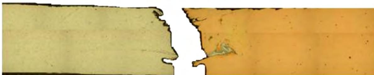
**Figure 4.11: Photo montage of fracture location of weld produced at 950 rpm and 300 mm/min with the 18 mm shoulder  $\phi$  due to weld defect**
