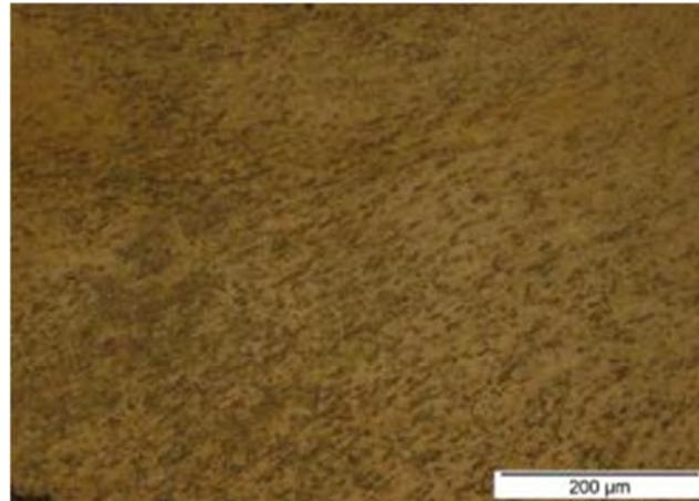
(b) TMAZ Cu produced with 18 mm  $\Phi$
