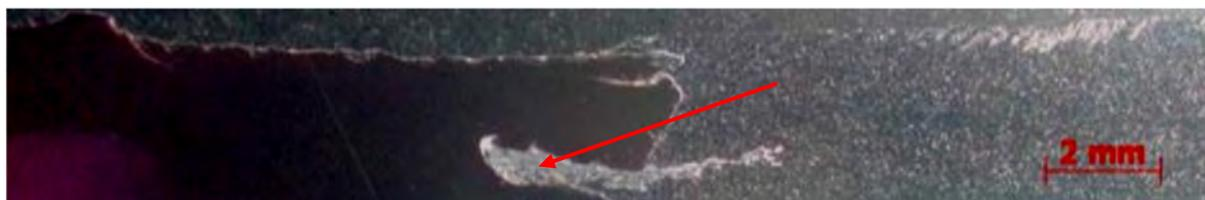
**Figure 4.3: Macro appearance of weld produced with the 18mm shoulder diameter tool at 950 rpm and 300 mm/min**
