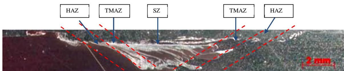
**Figure 4.4: Macro appearance of weld produced with the 18 mm shoulder diameter tool at 950 rpm and 50 mm/min**
