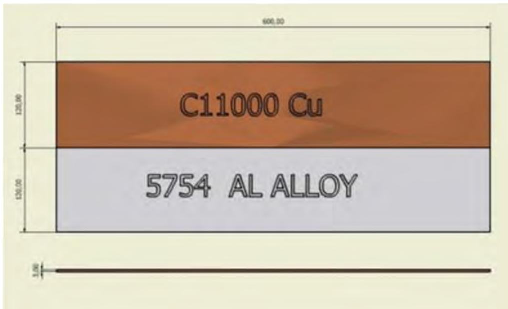
Figure 3.14: Research test coupon
