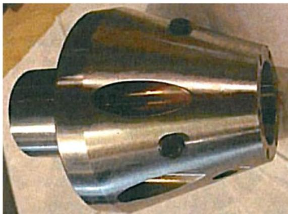
Figure B1a: FSW Tool holder<sup>137</sup>
