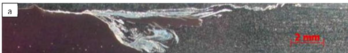
Figure 4.2 (a): Macro appearance of weld produced with the 15 mm shoulder diameter tool at 950 rpm and 50 mm/min
