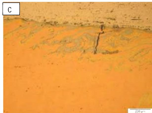
Figure 3c: Fracture location of tensile sample, T3 (x100).
