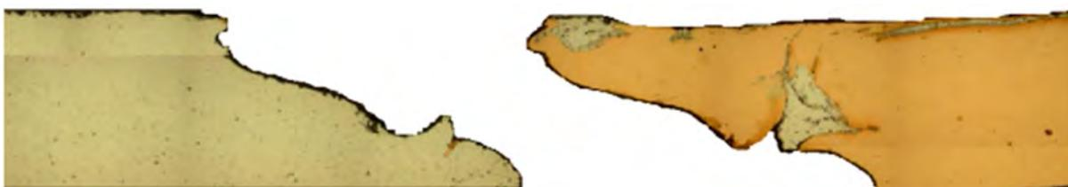
**(c) S25\_06 T1: Fractured surface of weld produced at 950 rpm and 300 mm/min with the 25 mm shoulder diameter tool**
