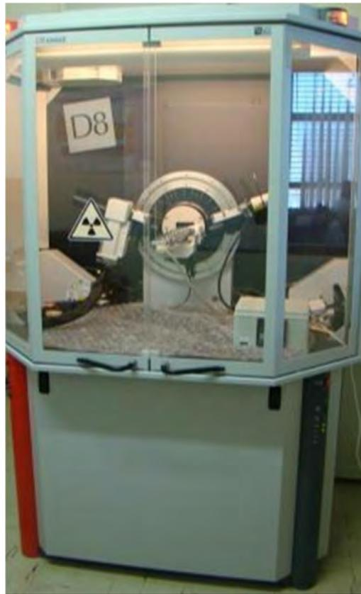
X- Ray Diffractometer (Bruker D8 Advance).
