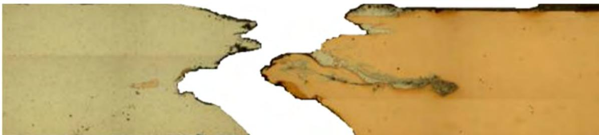
**(d) S25\_09 T1: Fractured surface of weld produced at 1200 rpm and 300 mm/min with the 25 mm shoulder diameter tool**
