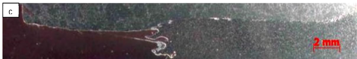
**Figure 4.2 (c): Macro appearance of weld produced with the 25mm shoulder diameter tool at 950 rpm and 50 mm/min**
