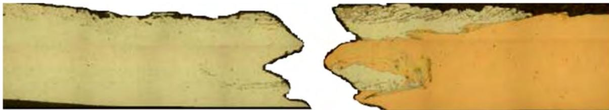
**(b) S18\_07 T1: Fractured surface of weld produced at 1200 rpm and 50 mm/min with the 18 mm shoulder diameter tool**
