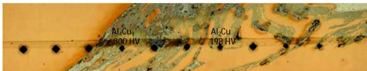
**Figure 4.19: Microhardness indentations at the interfacial region of S18\_04 produced at 950 rpm and 50 mm/min**
