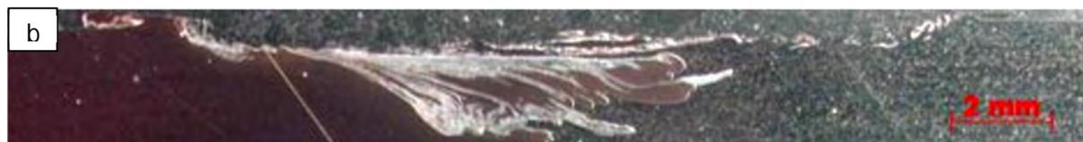
**Figure 4.2 (b): Macro appearance of weld produced with the 18mm shoulder diameter tool at 950 rpm and 50 mm/min**
