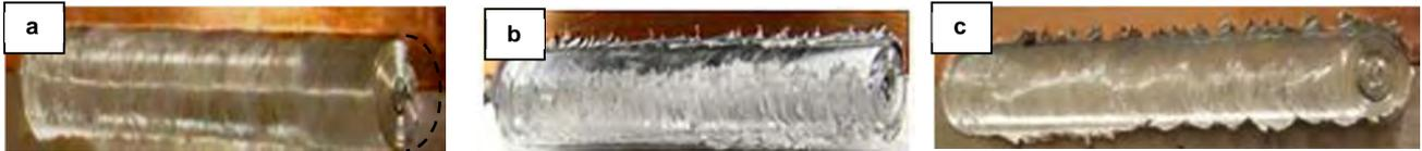
Figure 3.12: Welds produced at 950 rpm and 100 mm/min with (a) 1° tool tilt (b) 2° tool tilt (c) 3° tool tilt
