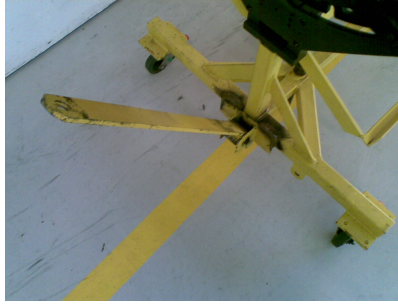
Figure 5.3: Tow Arm Welded to IP Trolley
