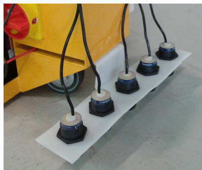
Figure 4.18: A Photo Showing the Mounted Bracket with Installed Sensors
