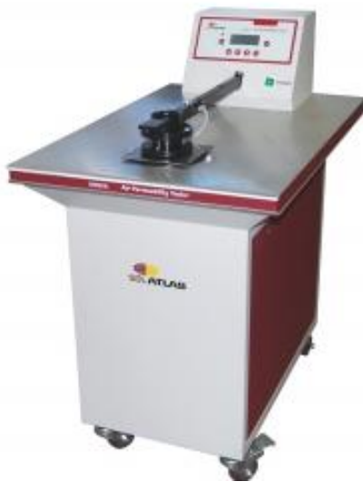
Figure 7: Atlas Air Permeability Tester (Source: SDL Atlas, n.d.)
