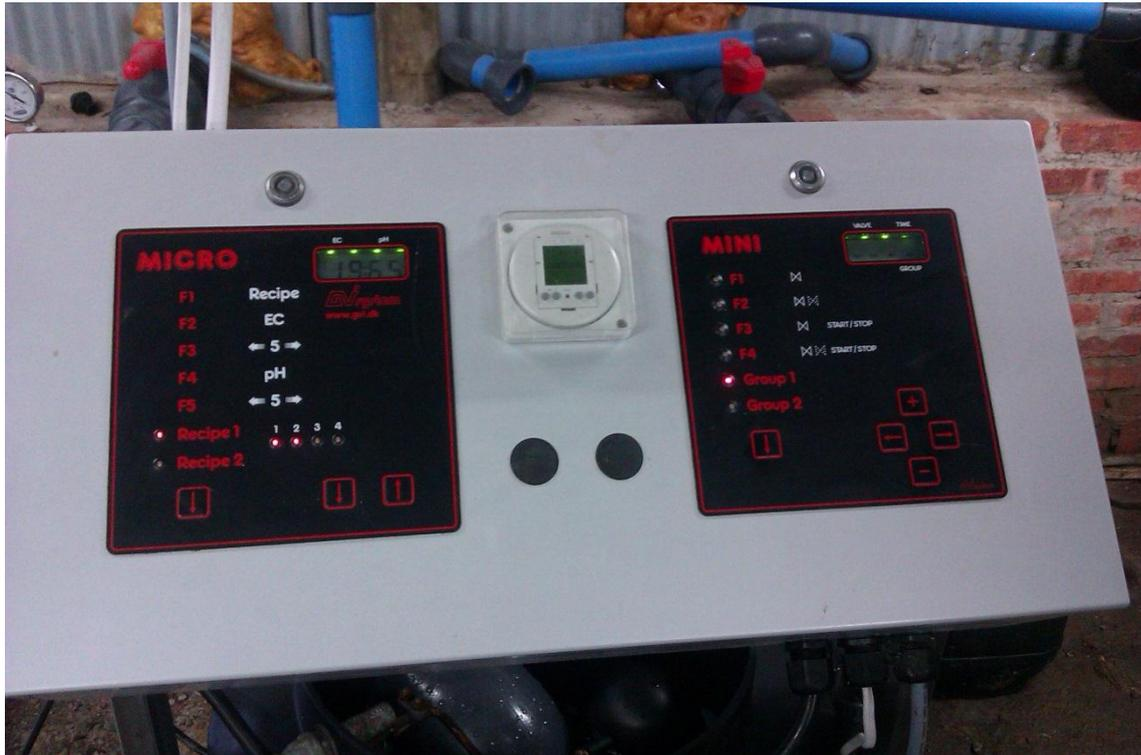
Figure 6- EC and pH measuring at Fertigation Point (pH in and EC in)
