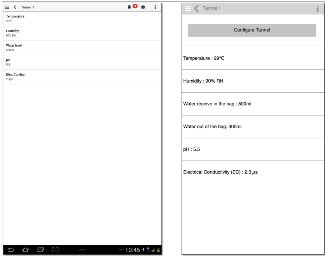
FIGURE 7.4: Real Time Monitoring Redesign (1<sup>st</sup>/2<sup>nd</sup> phase)
