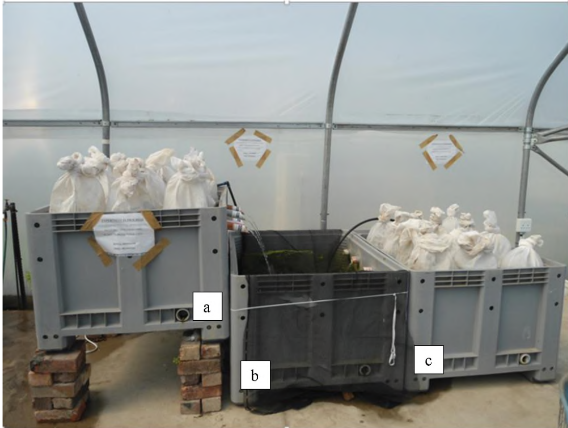
Figure 7.1 Photo of the experimental set up used during the two experiments carried out in South Africa. (a) the tidal tank, (b) reservoir and (c) the river tank.
