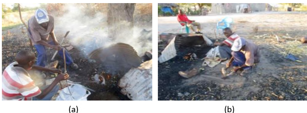
Figure 20: (a) Community member lifting hot metal from the mapukuta using a pipe insulated with a bark of a tree. (b) A community member hammering the metal using a hammer to turn it into a tool
