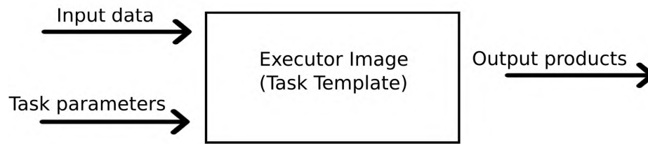
Figure 4.4: Structure of a stimela executor container.
