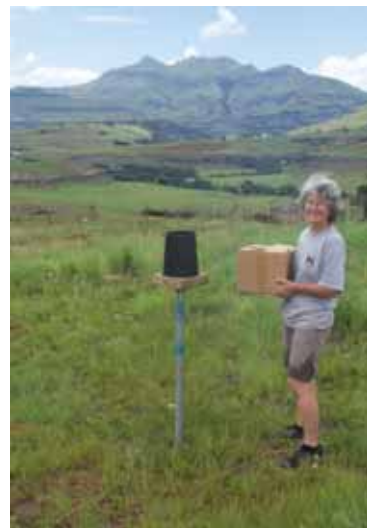
Laura Bannatyne setting up an autographic rain gauge in the upper Tsitsa catchment.
