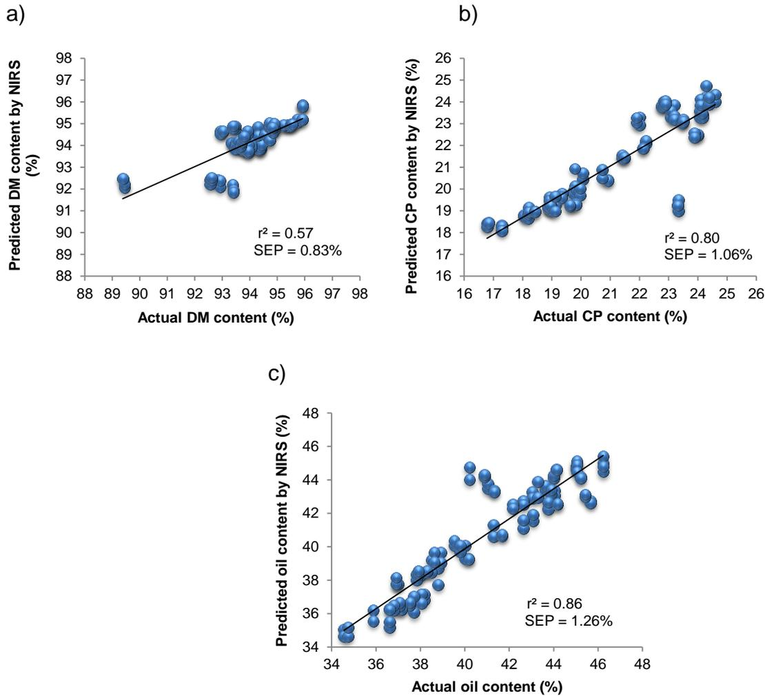
**Figure 4** The relationship between laboratory determined and NIR spectroscopy predicted content for (a) DM, (b) crude protein and (c) oil content in validation statistics for whole canola seed
