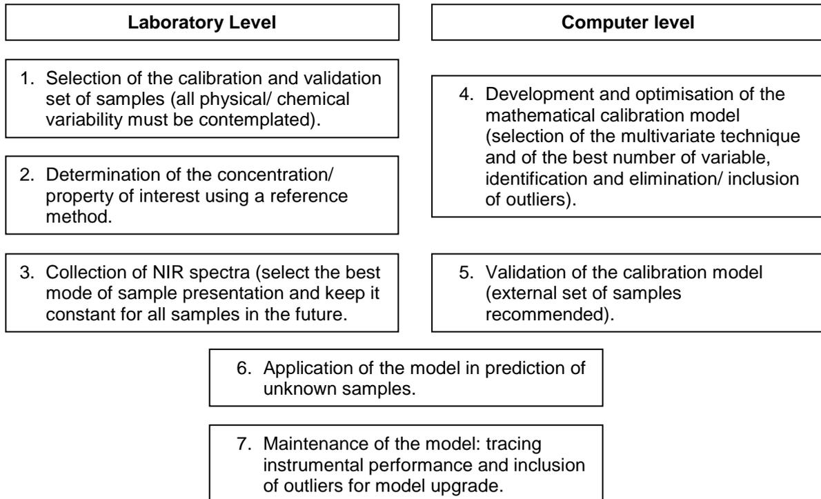
**Figure 1** Principal steps in the development, evaluation, use and maintenance of a quantitative model based on NIR spectroscopy (Pasquini, 2003)
