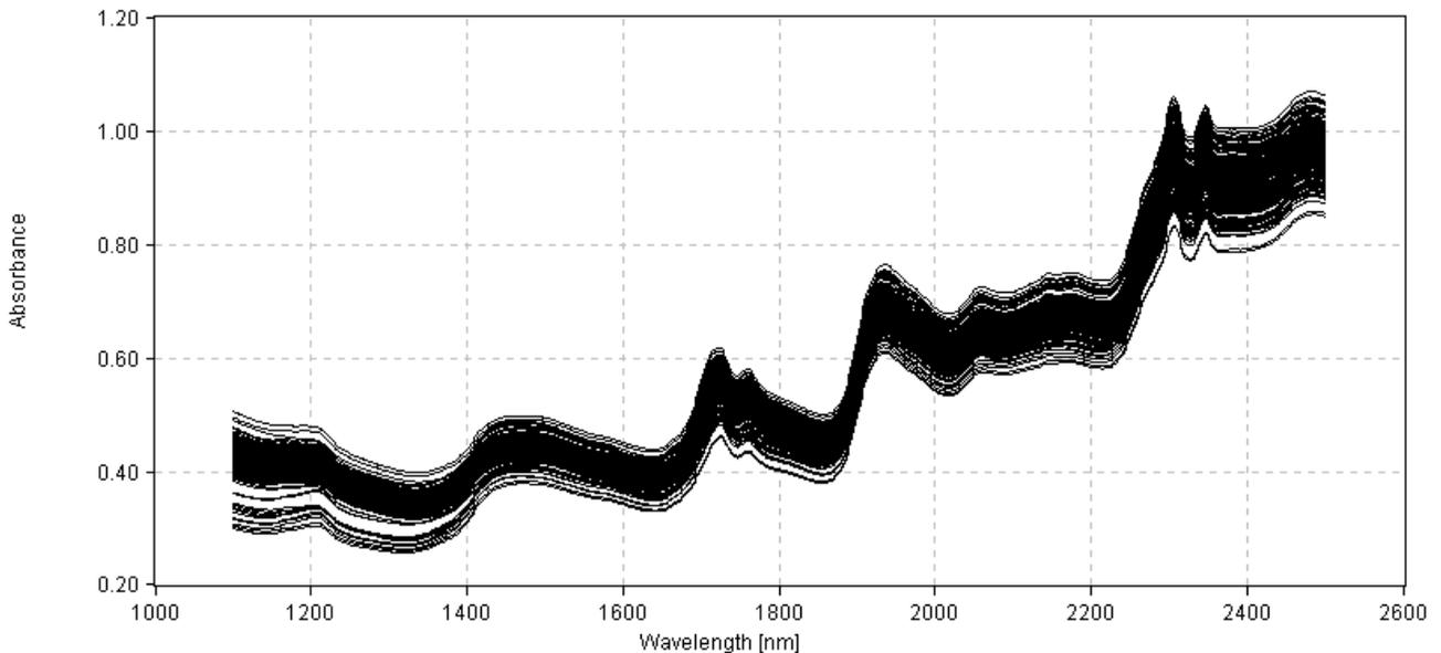
**Figure 1** Original near infrared reflectance spectra obtained for sunflower seed meal samples
