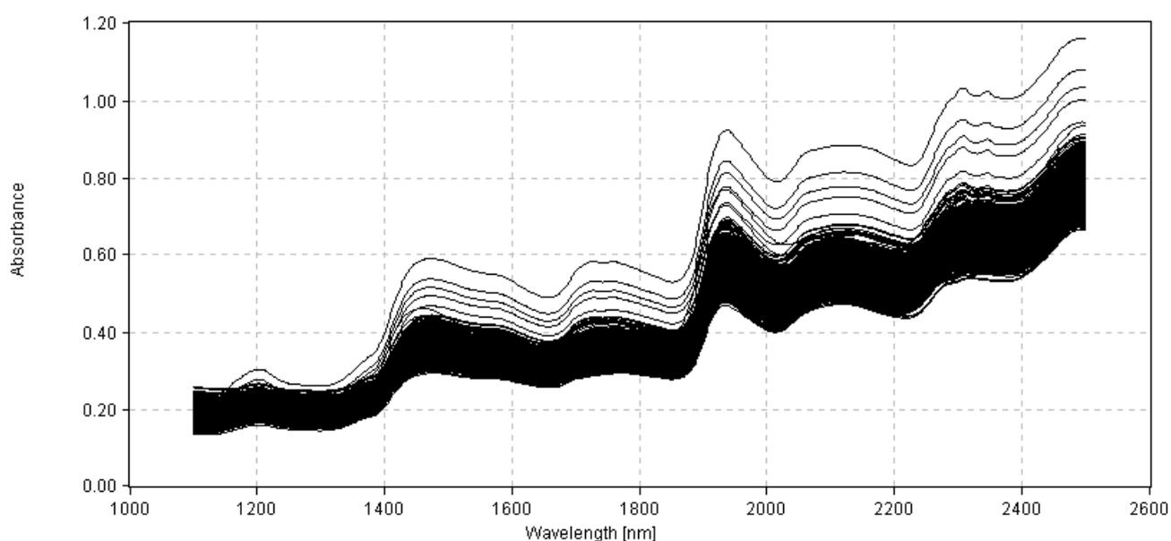
**Figure 1** Original absorbance spectra for ostrich total mixed rations scanned between 1100 - 2500 nm wavelengths
