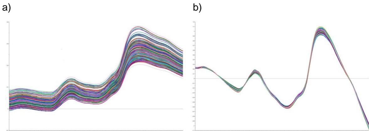
**Figure 1** Absorbance spectra for milled lupin seed for (a) raw data and (b) standard normal variate (SNV) detrend data in the NIR spectroscopy range
