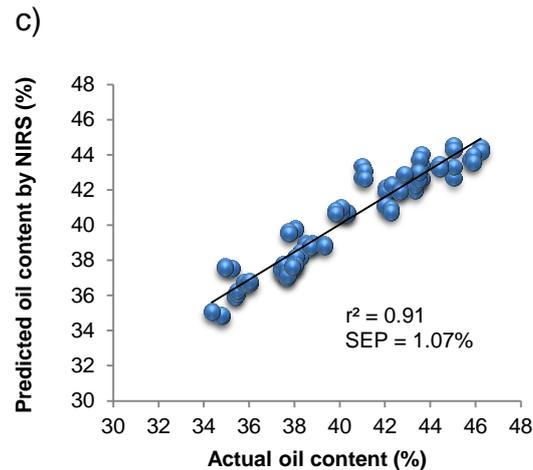
**Figure 3** The relationship between laboratory determined and NIR spectroscopy predicted content for (a) DM, (b) crude protein and (c) oil content in validation statistics for milled canola seed
