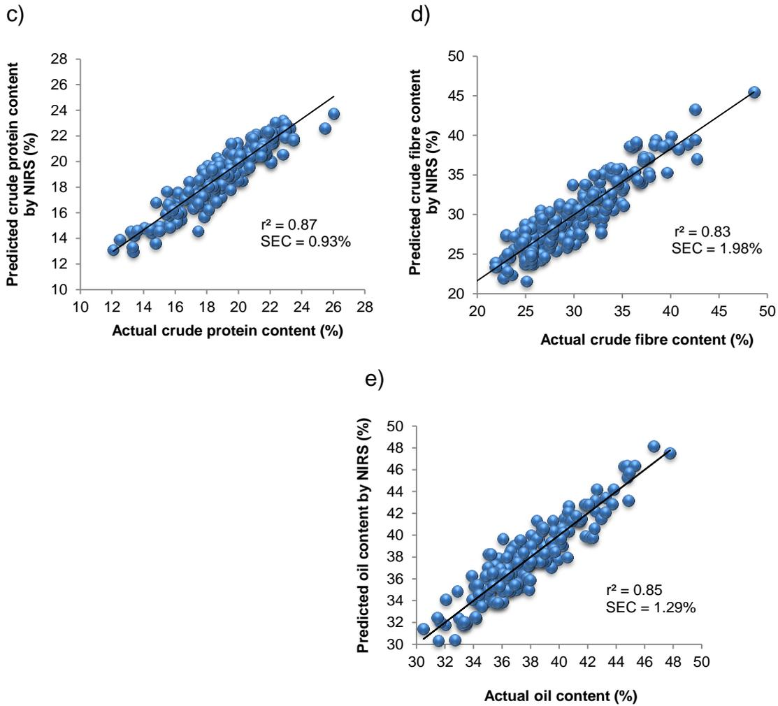
**Figure 1** The relationship between laboratory determined and NIR spectroscopy predicted values for (a) DM, (b) ash, (c) crude protein, (d) crude fibre and (e) oil content
