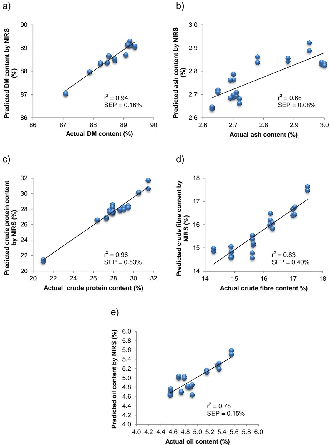
**Figure 3** The relationship between laboratory determined and NIR spectroscopy predicted values for (a) dry matter, (b) ash, (c) crude protein (d) crude fibre and (e) oil content in whole lupin seeds
