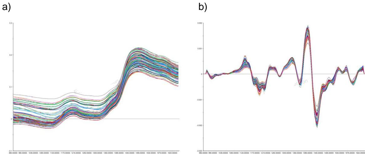
**Figure 1** Absorbance spectra for 60 alfalfa hay samples for (a) raw data and (b) Savitzky Golay 2<sup>nd</sup> derivative spectra in the NIR spectroscopy range
