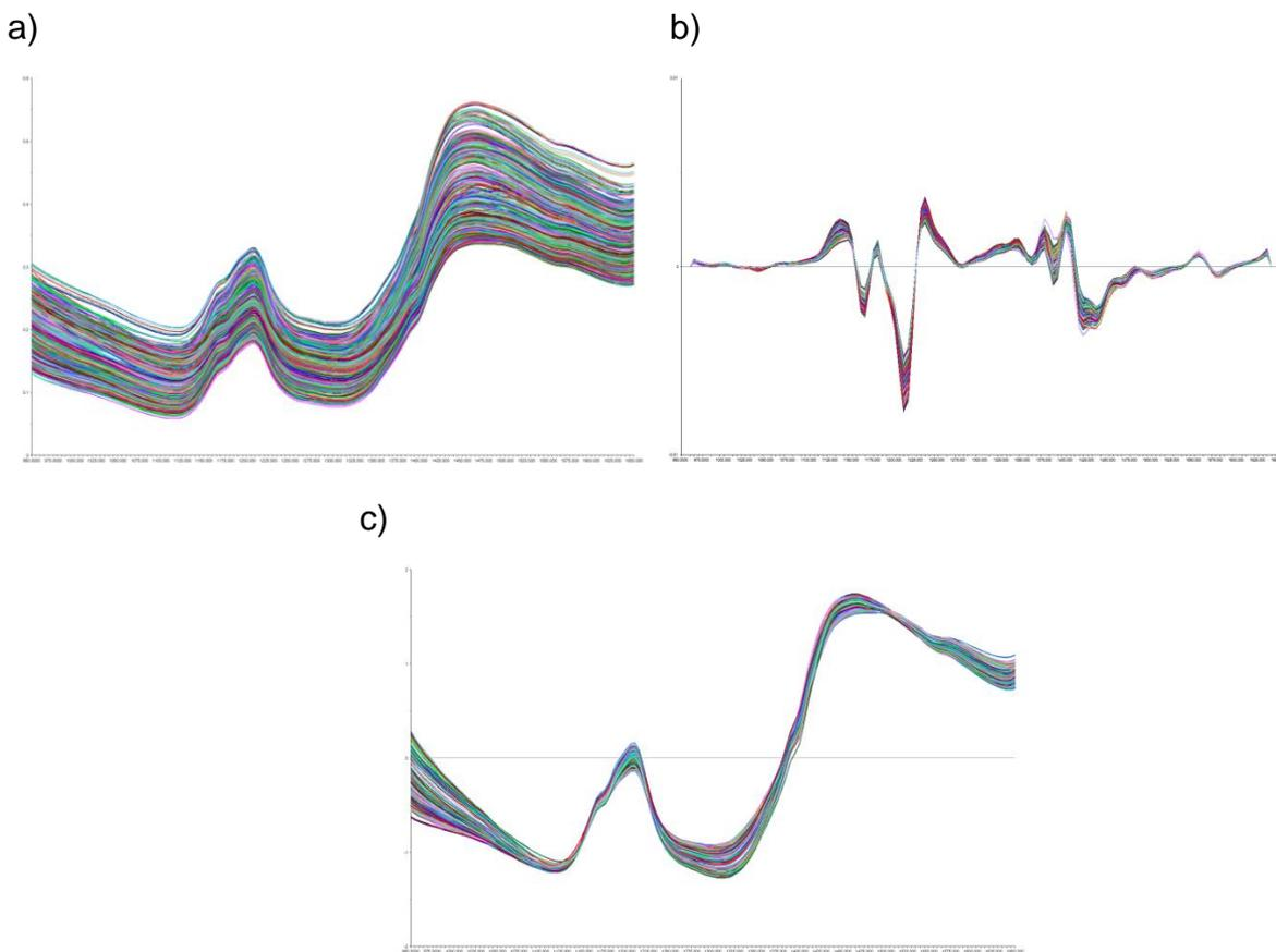
**Figure 1** Absorbance spectra for milled canola seeds from (a) raw data, (b) Savitzky Golay 2<sup>nd</sup> derivative data and (c) standard normal variate (SNV)
