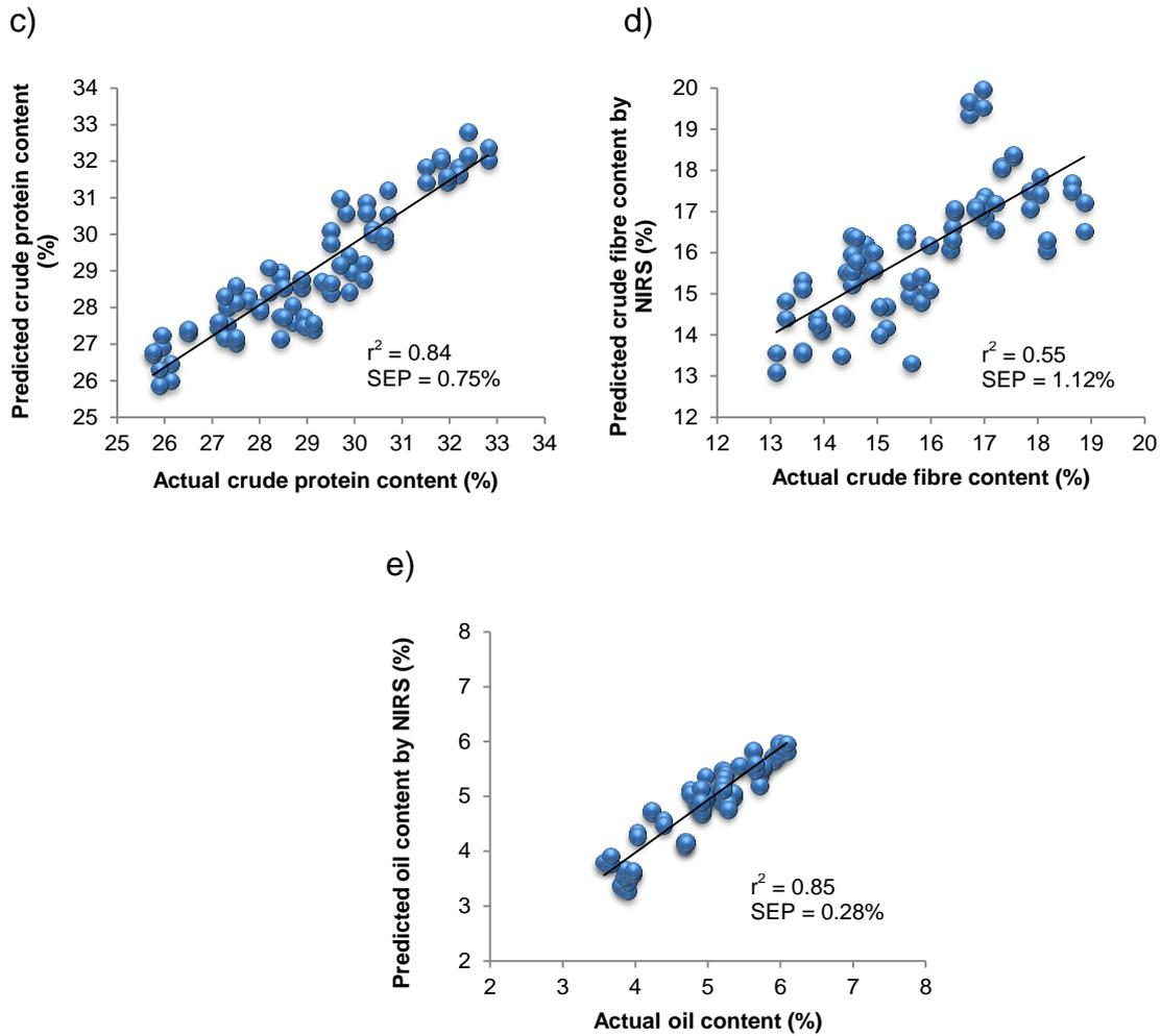
**Figure 2** The relationship between laboratory determined and NIR spectroscopy predicted values for (a) dry matter, (b) ash, (c) crude protein (d) crude fibre and (e) oil content in milled lupin seeds
