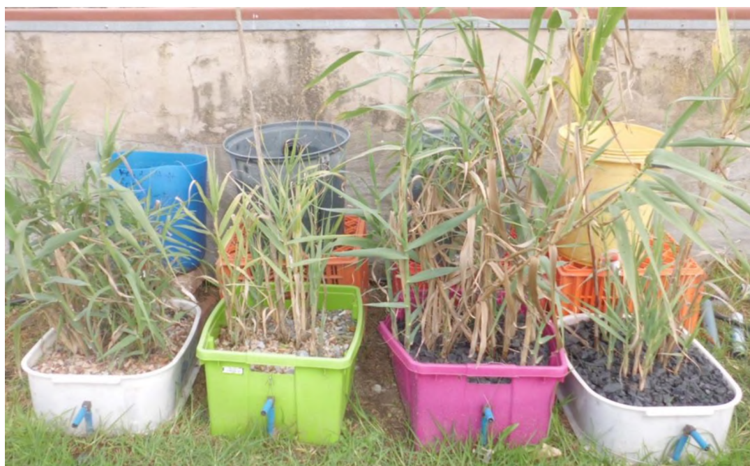
Figure 4-1. Image of the experimental set-up that was used in the study from right to left: discard coal + tap water, discard coal + AFP water, gravel + tap water and gravel + AFP effluent.
