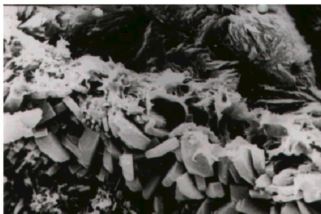
FIGURE 1 - The SEM image of the clinoptilolite sample used.
