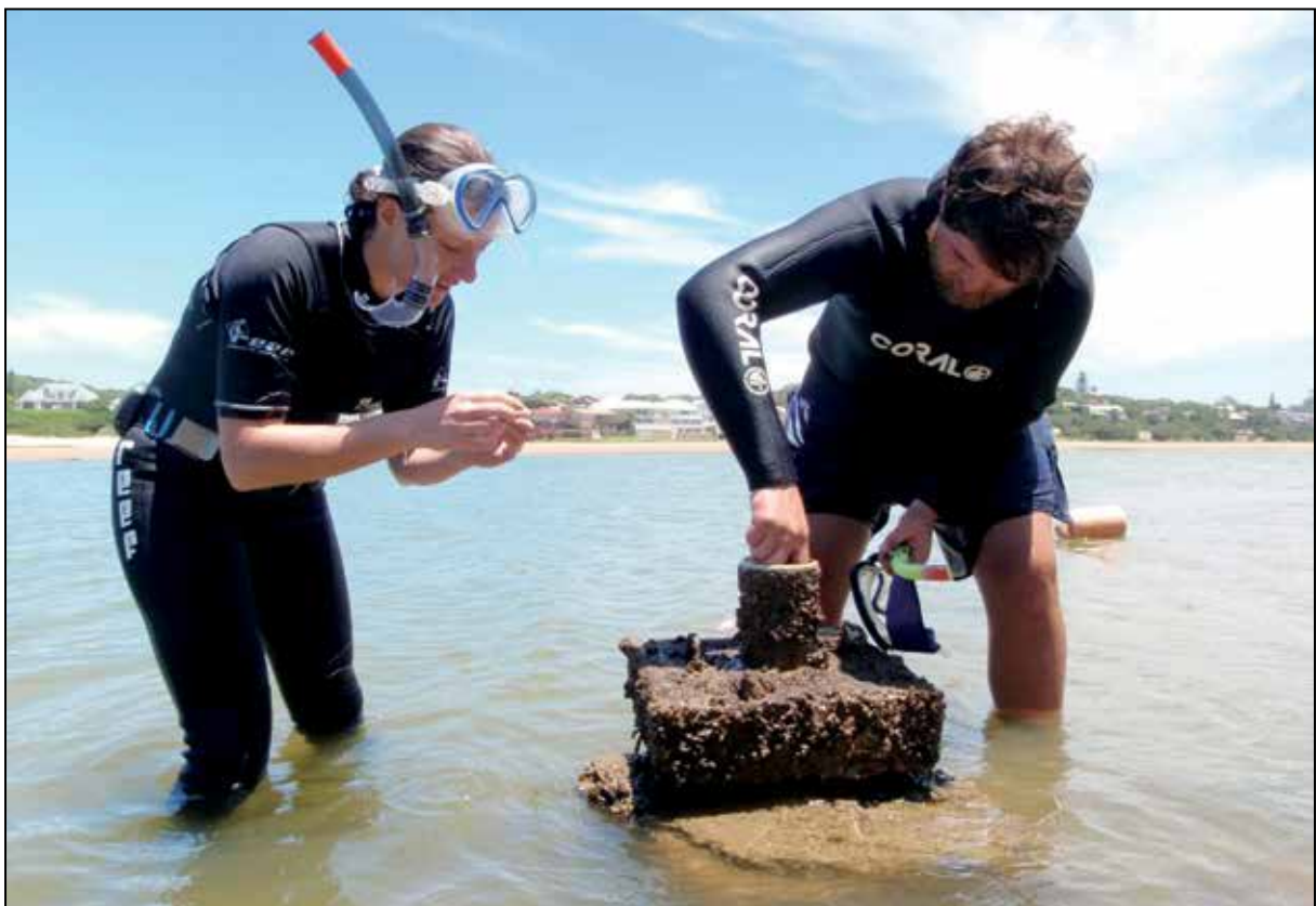
Figure 35. Taryn Murray and Dylan Howell retrieving an acoustic 'listening station' that had been recording the movements of acoustically tagged fish in the Bushmans Estuary (Photo: Paul Cowley).
