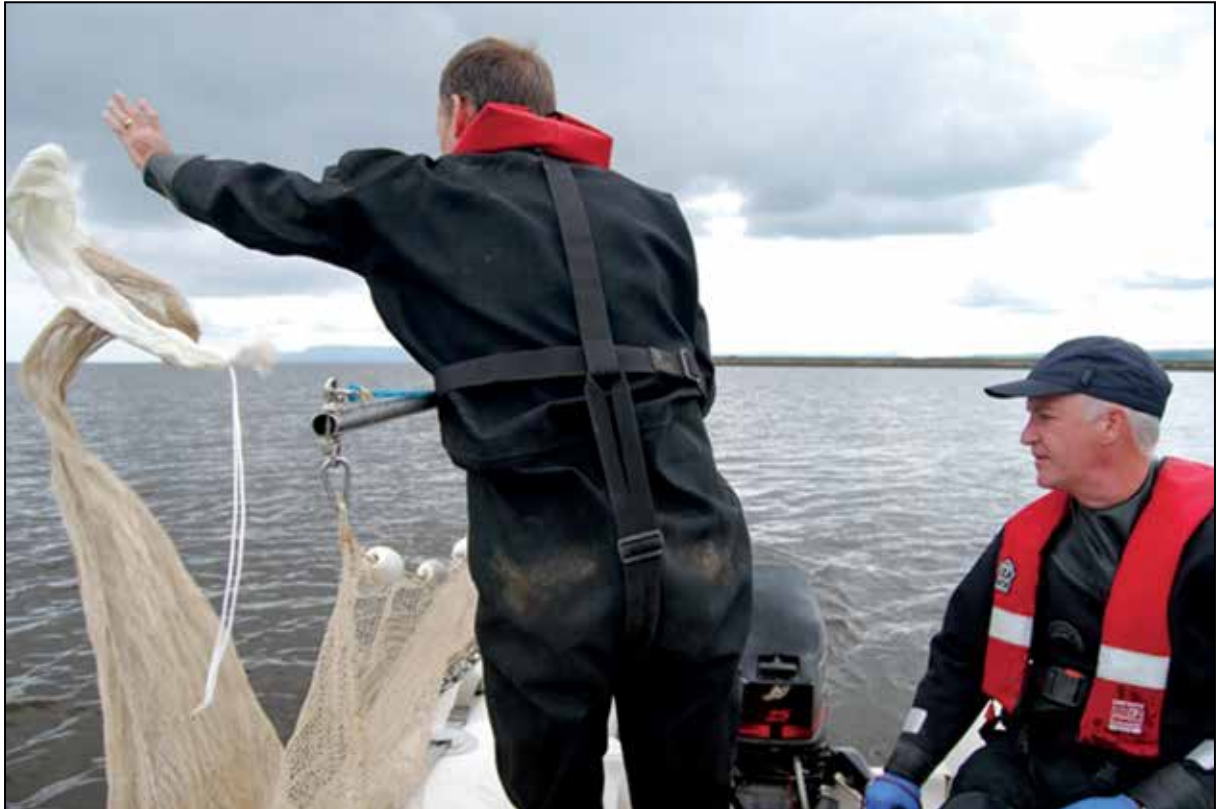
Figure 31. Deployment of the shoeless beam trawl, especially designed for use in estuaries, by Trevor Harrison, the creator of this particular sampling gear (Photo: Alan Whitfield).
