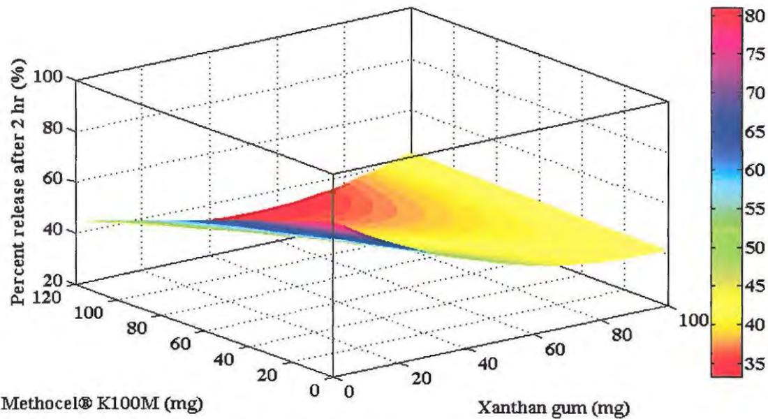
Figure 6.12 Response surface plot depicting the effect of Methocel<sup>®</sup> K100M and xanthan gum on percent SBS released after 2 hr with Carbopol<sup>®</sup> 974P and Surelease<sup>®</sup> concentrations at the centre level
