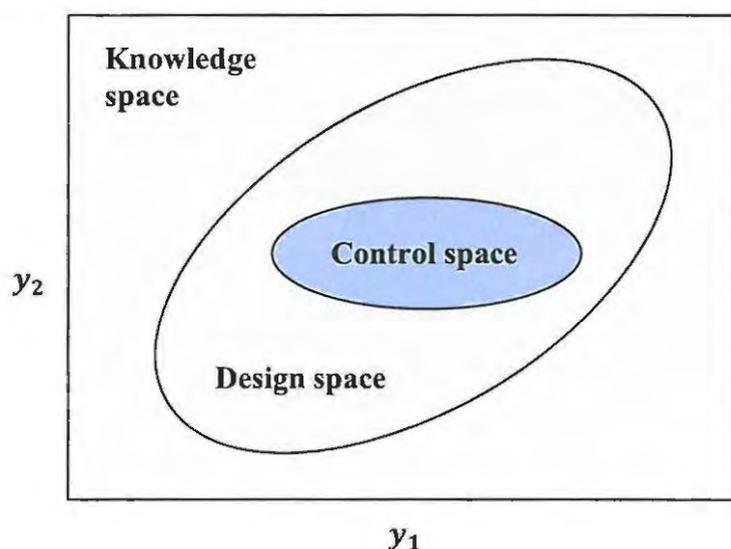
**Figure 8.1** The interrelationship between knowledge, design and control spaces with respect to CQA, redrawn and adapted from [227]
