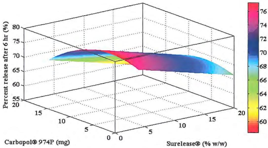
Figure 6.27 Response surface plot depicting the effect of Carbopol® 974P and Surelease® on percent SBS released after 6 hr with Methocel® K100M and xanthan gum concentrations at the centre level
