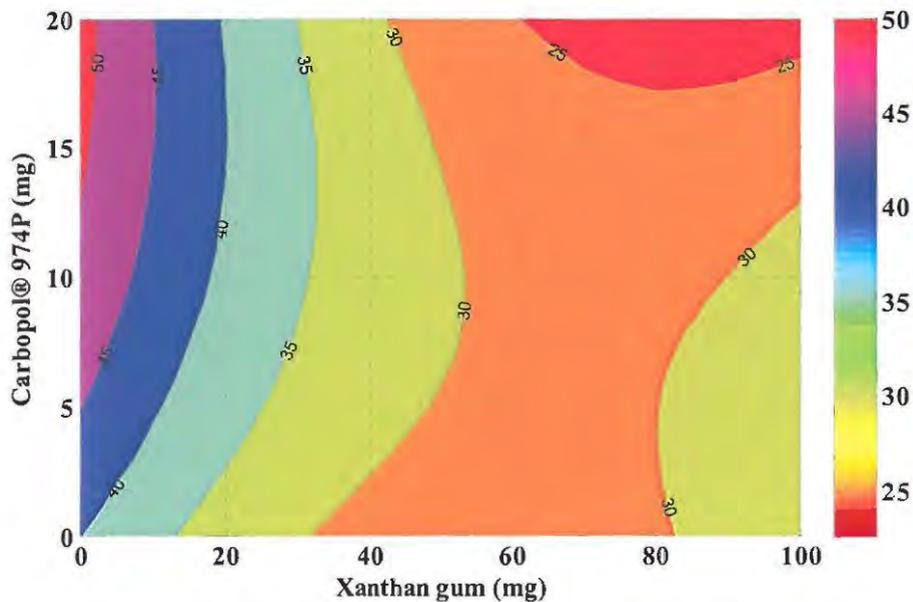
Figure 6.22 Contour plot depicting the effect of xanthan gum and Carbopol® 974P on percent SBS released after 1 hr with Methocel® K100M and Surelease® concentrations at the centre level
