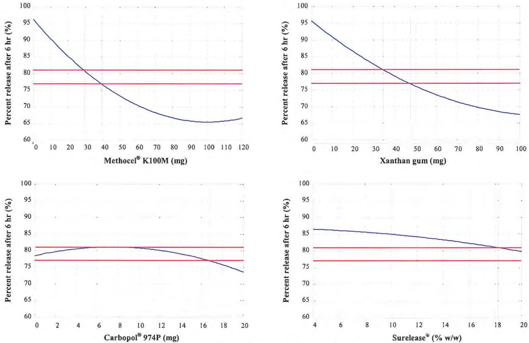
Figure 8.5 Constraint plots for percent SBS released after 6 hr dissolution testing
