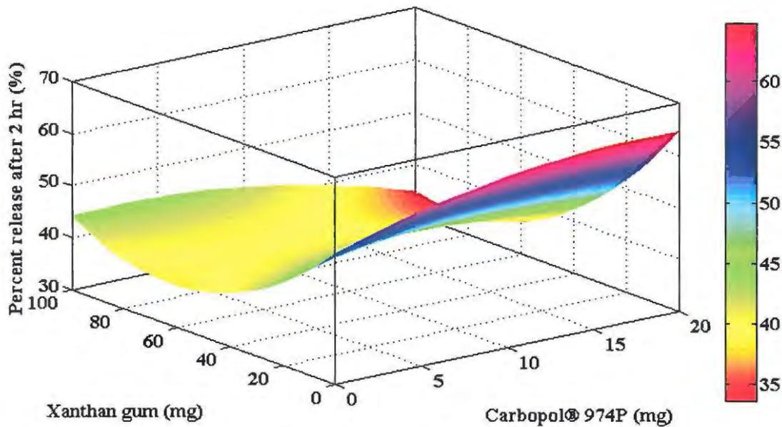
Figure 6.23 Response surface plot depicting the effect of xanthan gum and Carbopol® 974P on percent SBS released after 2 hr with Methocel® K100M and Surelease® concentrations at the centre level
