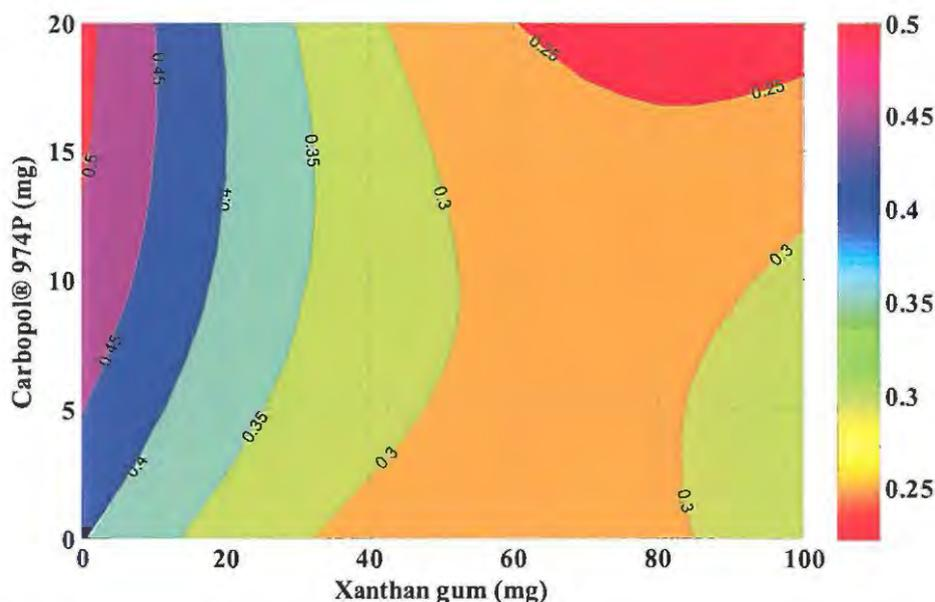
Figure 6.34 Contour plot depicting the effect of xanthan gum and Carbopol® 974P on the rate of SBS release with Methocel® K100M and Surelease® concentrations at the centre level
