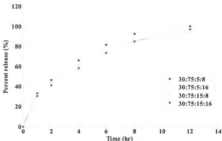
Figure 6.8 *In vitro* release of formulations containing low levels of Methocel® K100M and high levels of xanthan gum
