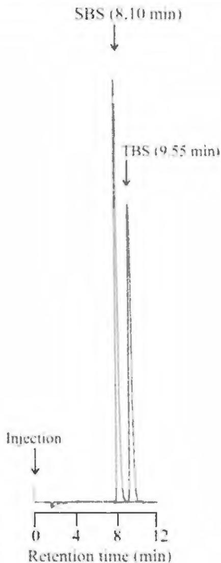
Figure 3.9 Representative chromatogram of SBS and TBS using the optimised mobile phase
