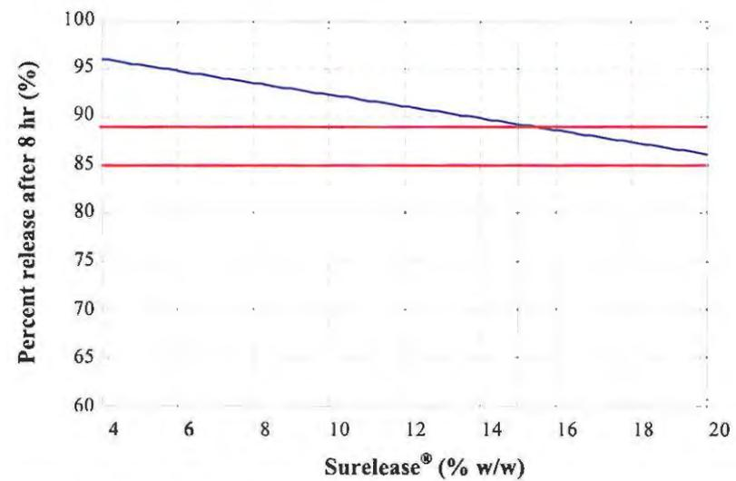
Figure 8.6 Constraint plots for percent SBS released after 8 hr of dissolution testing
