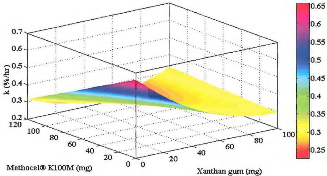
Figure 6.31 Response surface plot depicting the effect of Methocel® K100M and xanthan gum on SBS release rate with Carbopol® 974P and Surelease® concentration at the centre level
