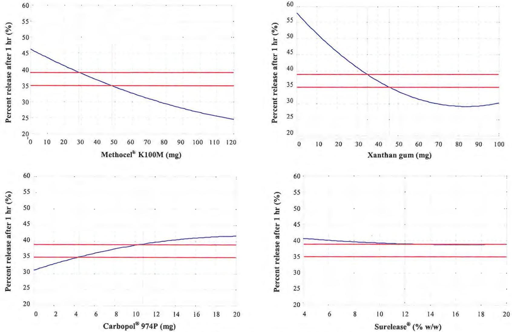
Figure 8.2 Constraints plots for percent SBS released after 1 hr of dissolution testing
