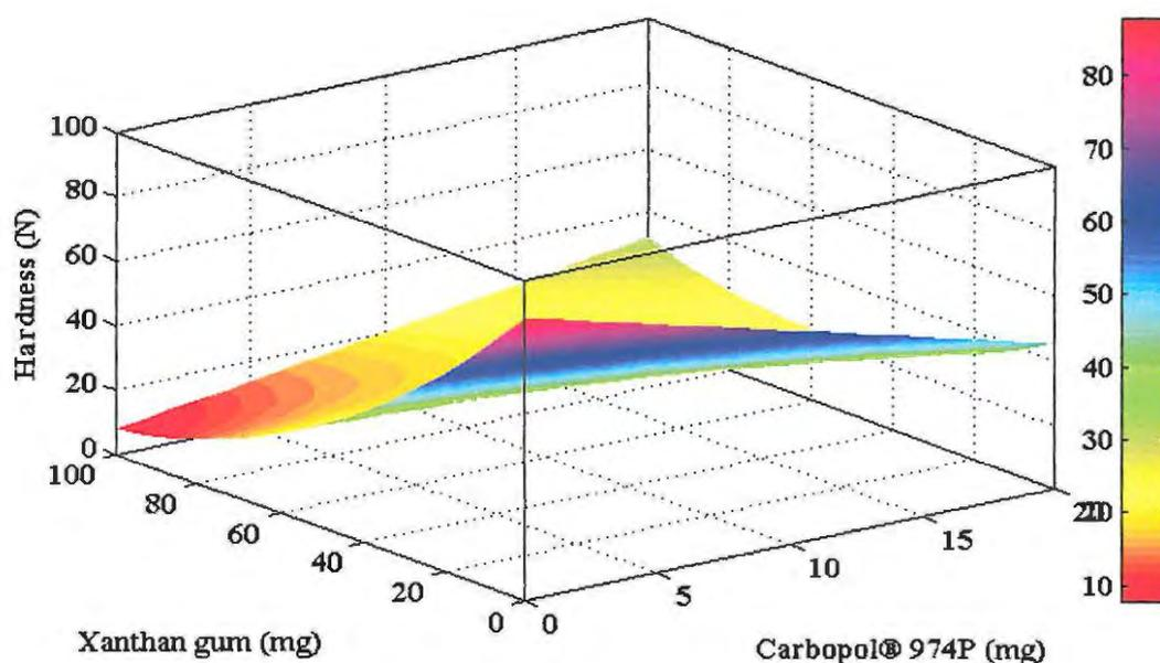
**Figure 6.2** Response surface plot depicting the effect of and xanthan gum and Carbopol® 974P on tablet crushing strength with Methocel® K100M and Surelease at the centre levels
