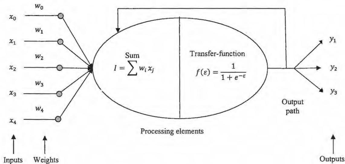
Figure 7.1 A simple artificial neuron, adapted from [209,211]
