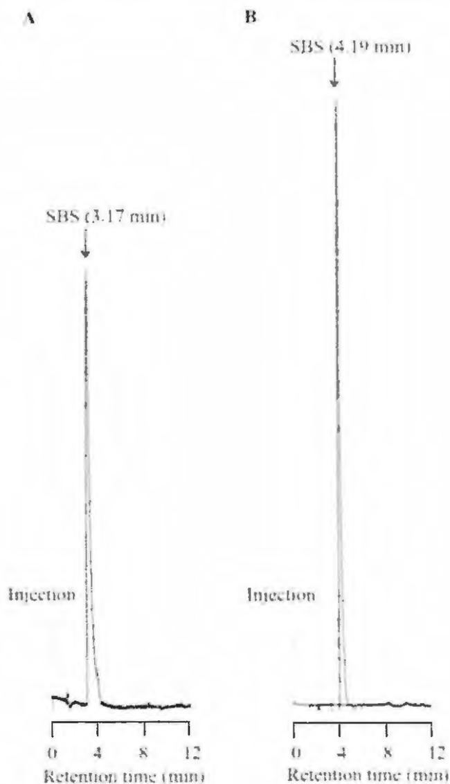
**Figure 3.2** Representative chromatograms developed using USP [95] (A) or BP [23] (B) chromatographic conditions
