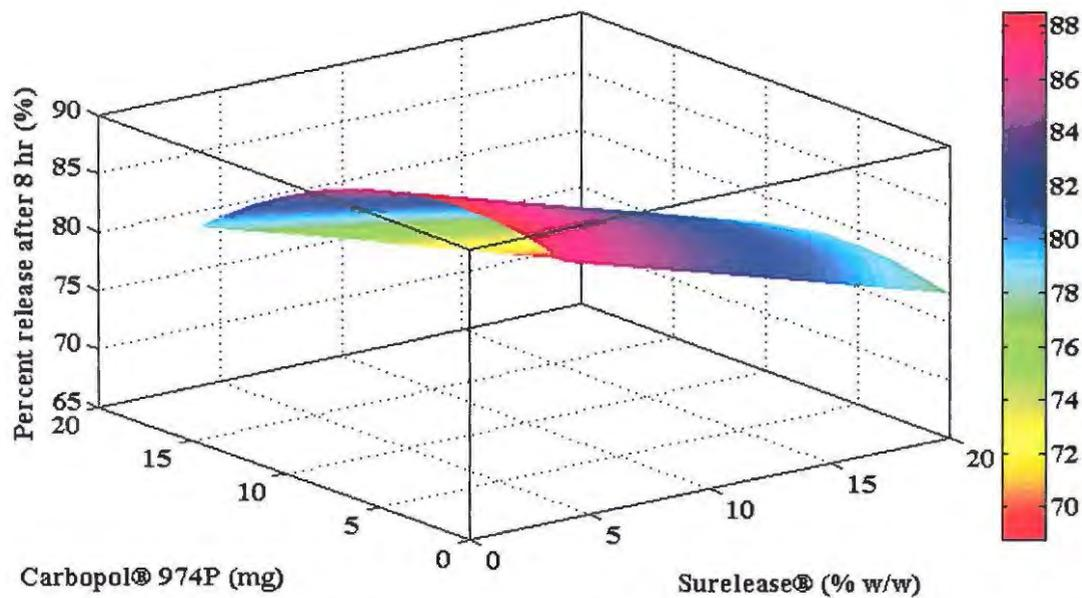
Figure 6.29 Response surface plot depicting the effect of Carbopol® 974P and Surelease® on percent SBS released after 8 hr with Methocel® K100M and xanthan gum concentrations at the centre level
