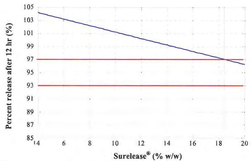
Figure 8.7 Constraint plots for percent SBS released after 12 hr of dissolution testing
