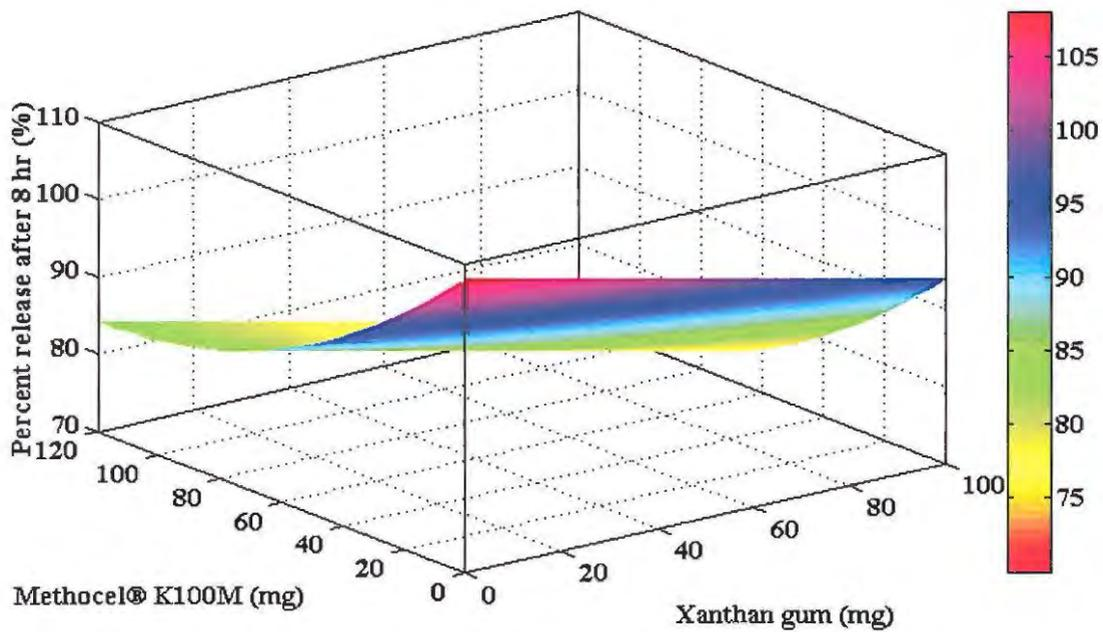
Figure 6.18 Response surface plot depicting the effect of Methocel® K100M and xanthan gum on percent SBS released after 8 hr with Carbopol® 974P and Surelease® concentrations at the centre level
