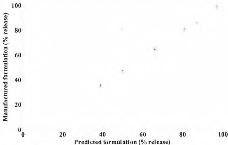
Figure 6.43 Percent release of the manufactured formulation vs. predicted formulation,  $y = x - 2.6$ ,  $R^2 = 0.9928$
