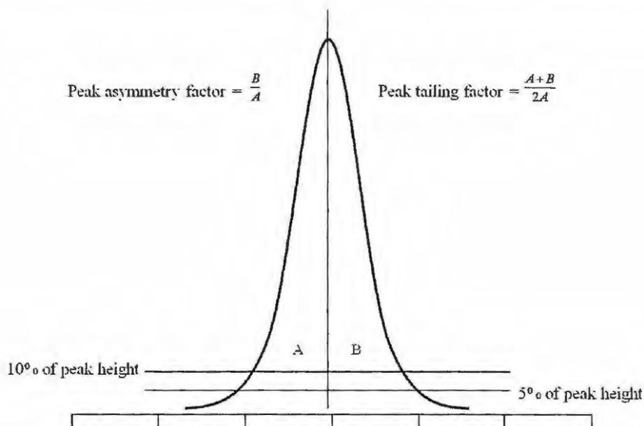
Figure 3.3 Schematic representation for the determination of peak asymmetry and peak tailing factors
