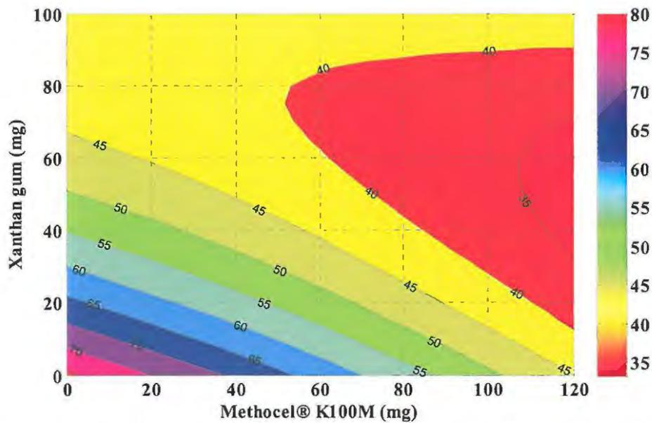
**Figure 6.13** Contour plot depicting the effect of Methocel<sup>®</sup> K100M and xanthan gum on percent SBS released after 2 hr with Carbopol<sup>®</sup> 974P and Surelease<sup>®</sup> concentrations at the centre level
