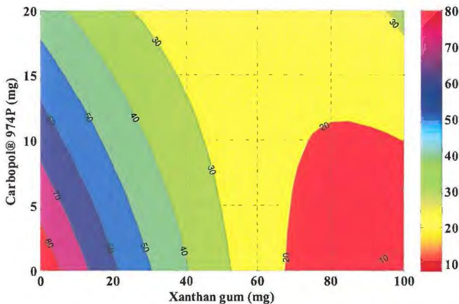
**Figure 6.3** Contour plot depicting the effect of and xanthan gum and Carbopol® 974P on tablet crushing strength with Methocel® K100M and Surelease at their centre levels
