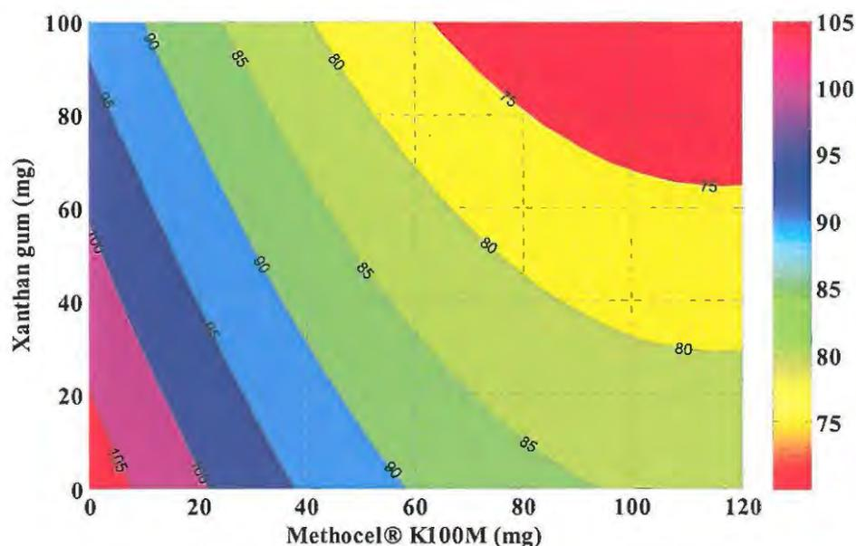
**Figure 6.19** Contour plot depicting the effect of Methocel® K100M and xanthan gum on percent SBS released after 8 hr with Carbopol® 974P and Surelease® concentrations at the centre level
