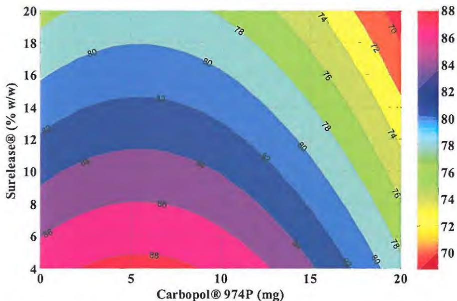
Figure 6.30 Contour plot depicting the effect of Carbopol® 974P and Surelease® on percent SBS released after 8 hr with Methocel® K100M and xanthan gum concentrations at the centre level
