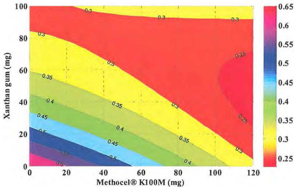
Figure 6.32 Contour plot depicting the effect of Methocel® K100M and xanthan gum on SBS release rate with Carbopol® 974P and Surelease® concentrations at the centre level
