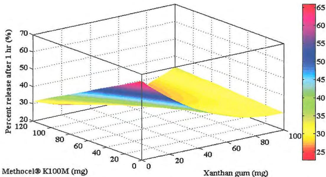
Figure 6.10 Response surface plot depicting the effect of Methocel<sup>®</sup> K100M and xanthan gum on percent SBS released after 1 hr with Carbopol<sup>®</sup> 974P and Surelease<sup>®</sup> concentrations at the centre level
