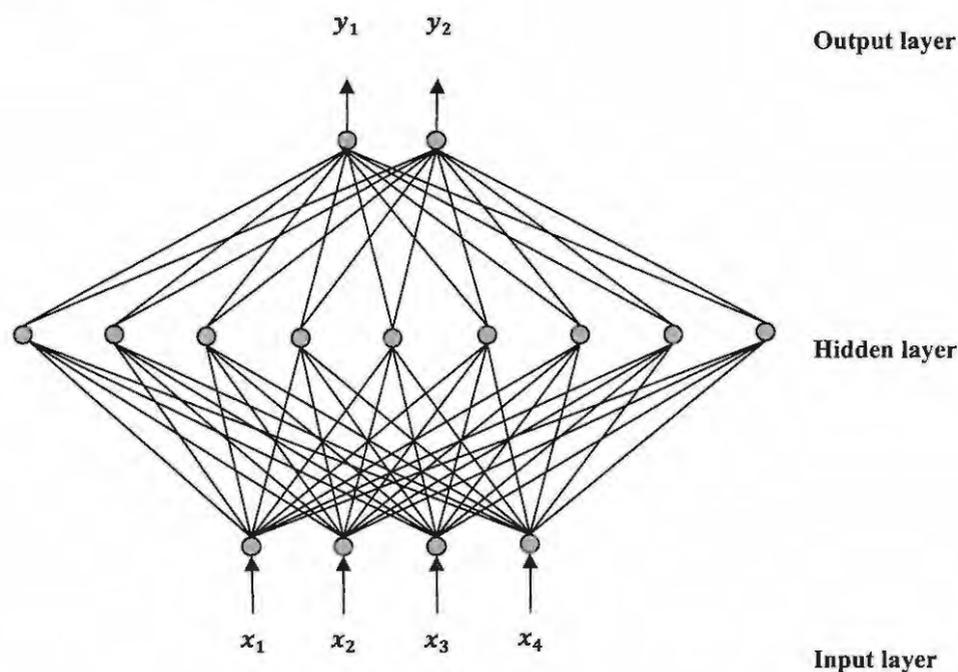
**Figure 7.2** MLP architecture for ANN where  $x_1 - x_4$  are inputs and  $y_1$  and  $y_2$  represent response factors, adapted and redrawn from [209,211]
