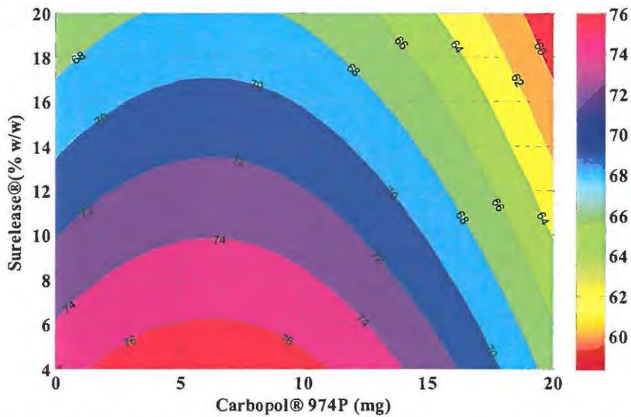
Figure 6.28 Contour plot depicting the effect of Carbopol® 974P and Surelease® on percent SBS released after 6 hr with Methocel® K100M and xanthan gum concentrations at the centre level
