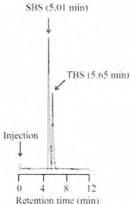
**Figure 3.6** Typical chromatogram showing the separation of SBS and TBS using 20% v/v ACN in 18 mM phosphate buffer at pH 4, containing 15 mM sodium octane sulphonate
