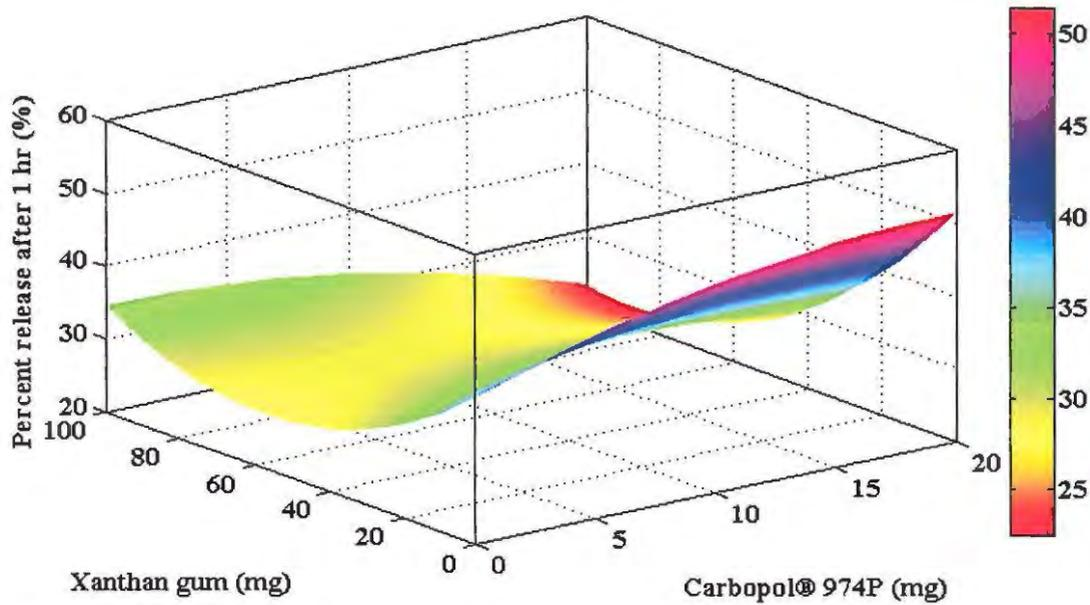
Figure 6.21 Response surface plot depicting the effect of xanthan gum and Carbopol® 974P on percent SBS released after 1 hr with Methocel® K100M and Surelease® concentrations at the centre level
