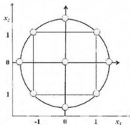
**Figure 6.1** Diagrammatic representation of a central composite design with full factorial points and star points, adapted and redrawn from [180]
