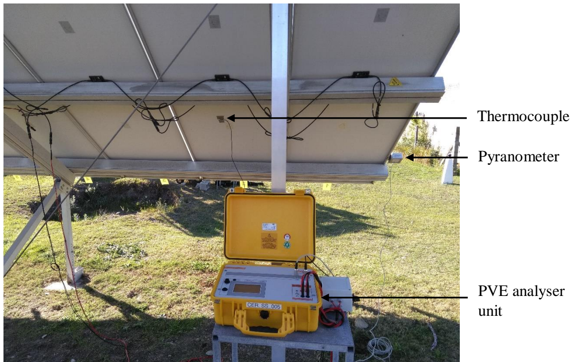
Figure 3-9: I-V measurement equipment set up at ORF.
