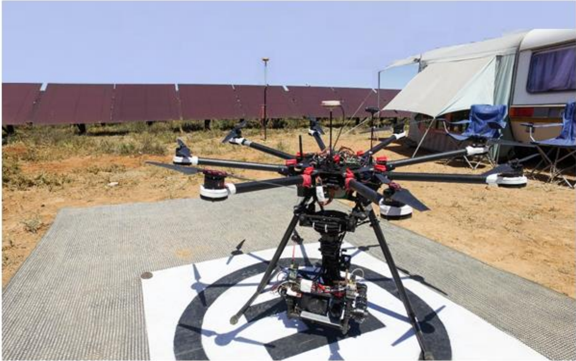
Figure 3-2: UAV with I-R camera used for monitoring PV module strings at ERIC.
