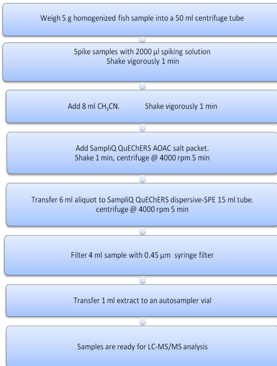
**Scheme 4.5.3: Flow chart of QuEChERS AOAC sample preparation procedure (fish)**
