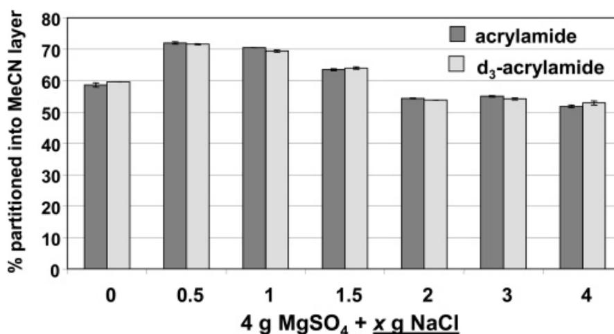
**Figure 3.5.3: Partition of acrylamide and  $d_3$ -acrylamide (in %) into the MeCN layer in the experiments involving addition of 4 g of  $\text{MgSO}_4$  and 0-4 g of NaCl to 50 ng/ml composite solutions of acrylamide and  $d_3$ -acrylamide in water-MeCN [189]**
