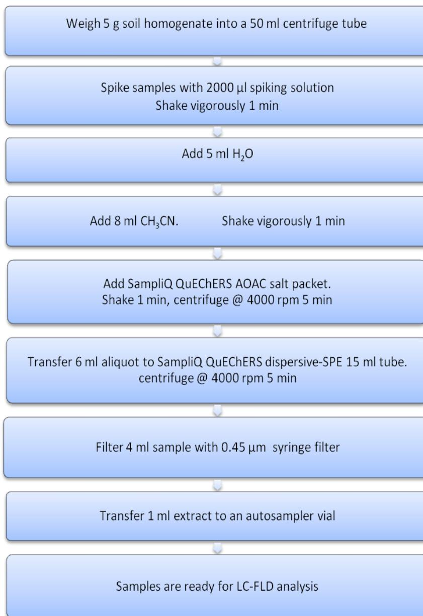
**Scheme 4.5.4: Flow chart of QuEChERS AOAC sample preparation procedure (soil)**
