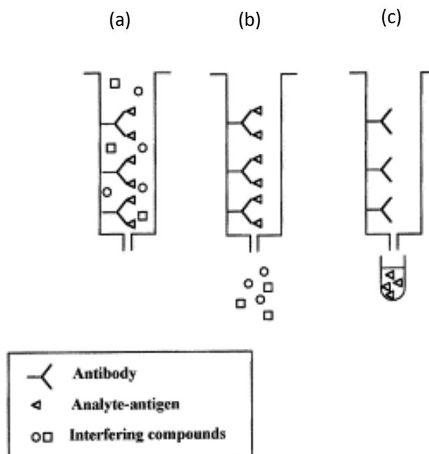
**Figure 2.5.2.2: Off-line procedure used for the immune-sample pretreatment on immunosorbents. (a) percolation of the sample; (b) washing to eliminate the non-retained compounds; (c) elution of compounds retained by the immobilized antibodies [75].**
