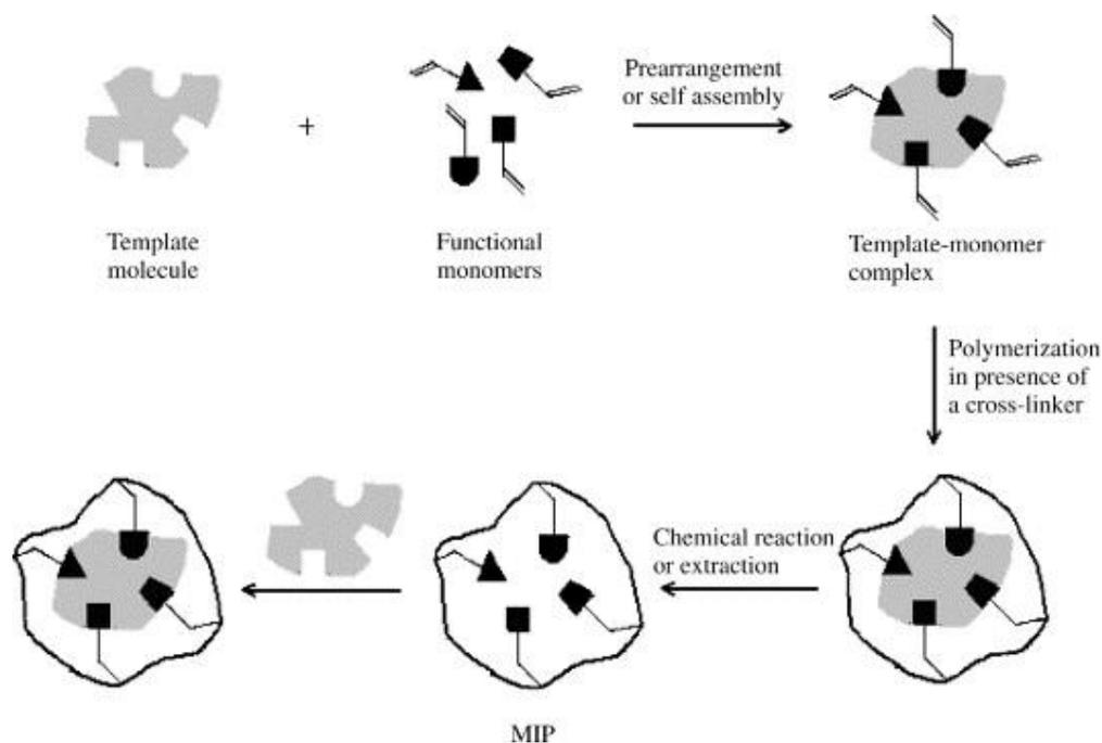
Figure 2.5.2.3: Synthesis of MIPs and its selective recognition to target molecule [82]
