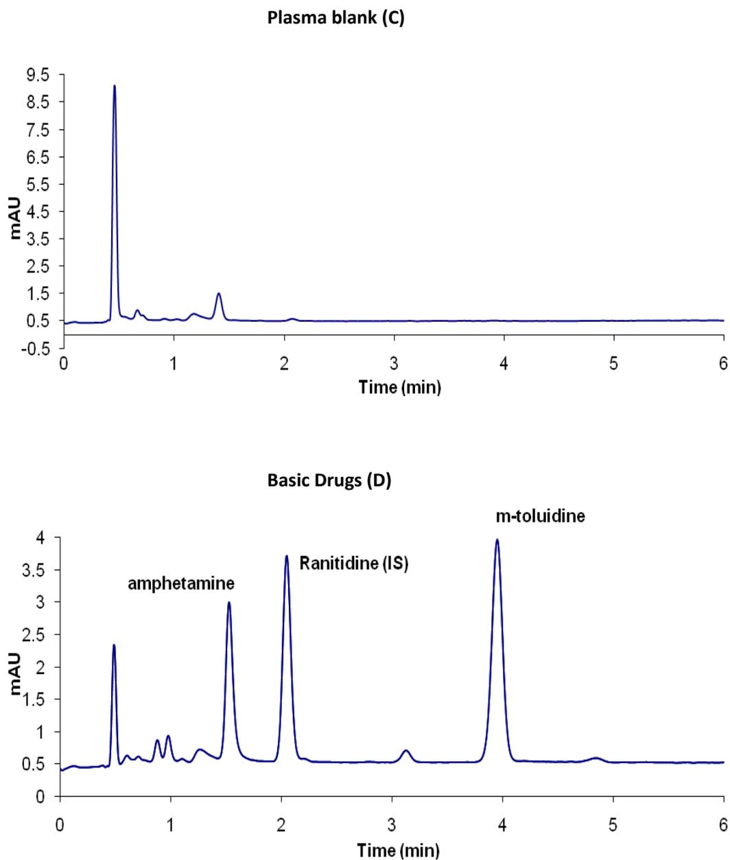
**Fig. 5.1.4:** (continuation) Eluate 2 Chromatograms of (c) blank plasma extract; (d) spiked plasma extract; *Chromatographic conditions:* stationary phase, ZORBAX C<sub>18</sub> column (4.6 mm × 75 mm i.d., 3.5 μm); mobile phase, methanol /25 mM phosphate buffer containing pH 7; flow rate, 1.5 ml/min; injection volume, 5 μL; detection wavelength, 210 nm.
