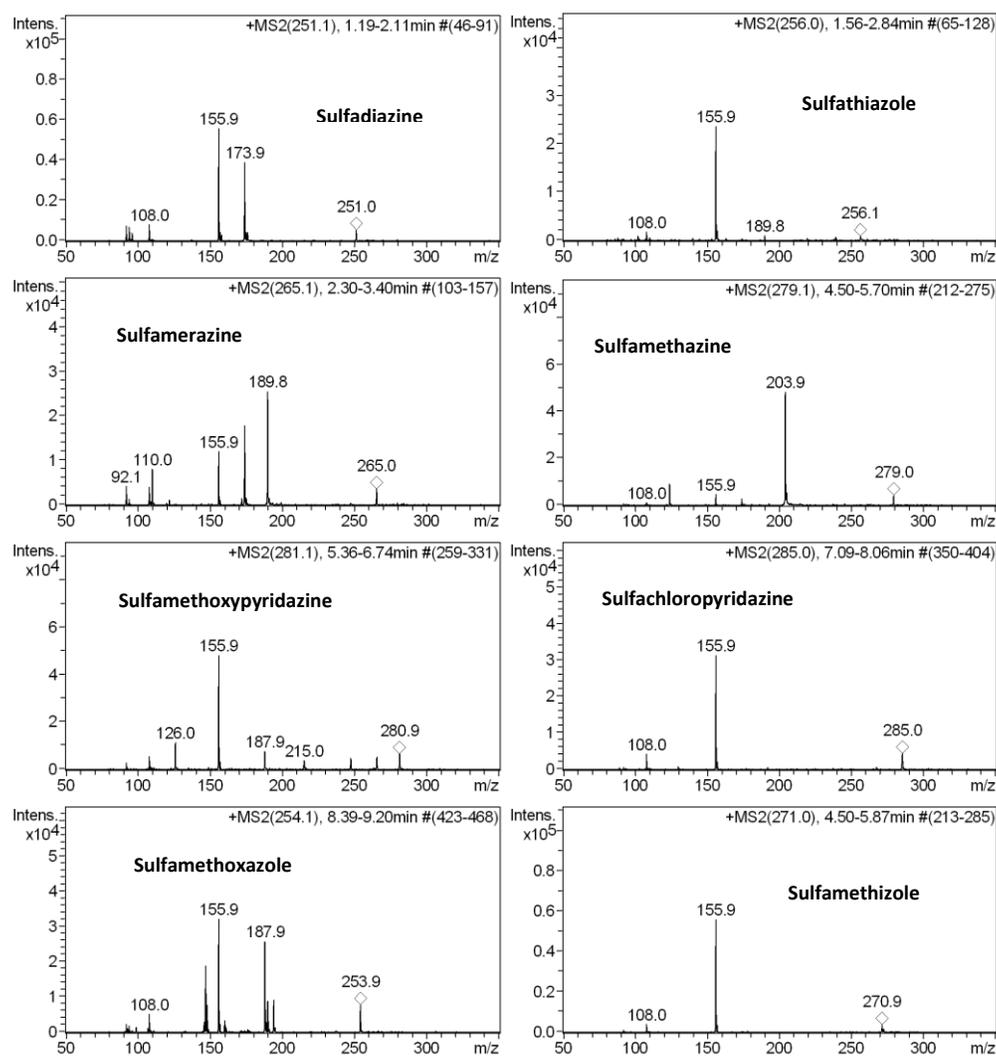
**Figure 5.3.4: Mass spectrum of chicken muscle sample spiked with sulfonamides (200 ng/g) using conditions described in Table 4.4.4**
