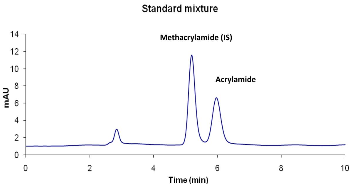
Figure 5.4.1: Chromatogram of the standard mixture of acrylamide and methacrylamide (IS)
