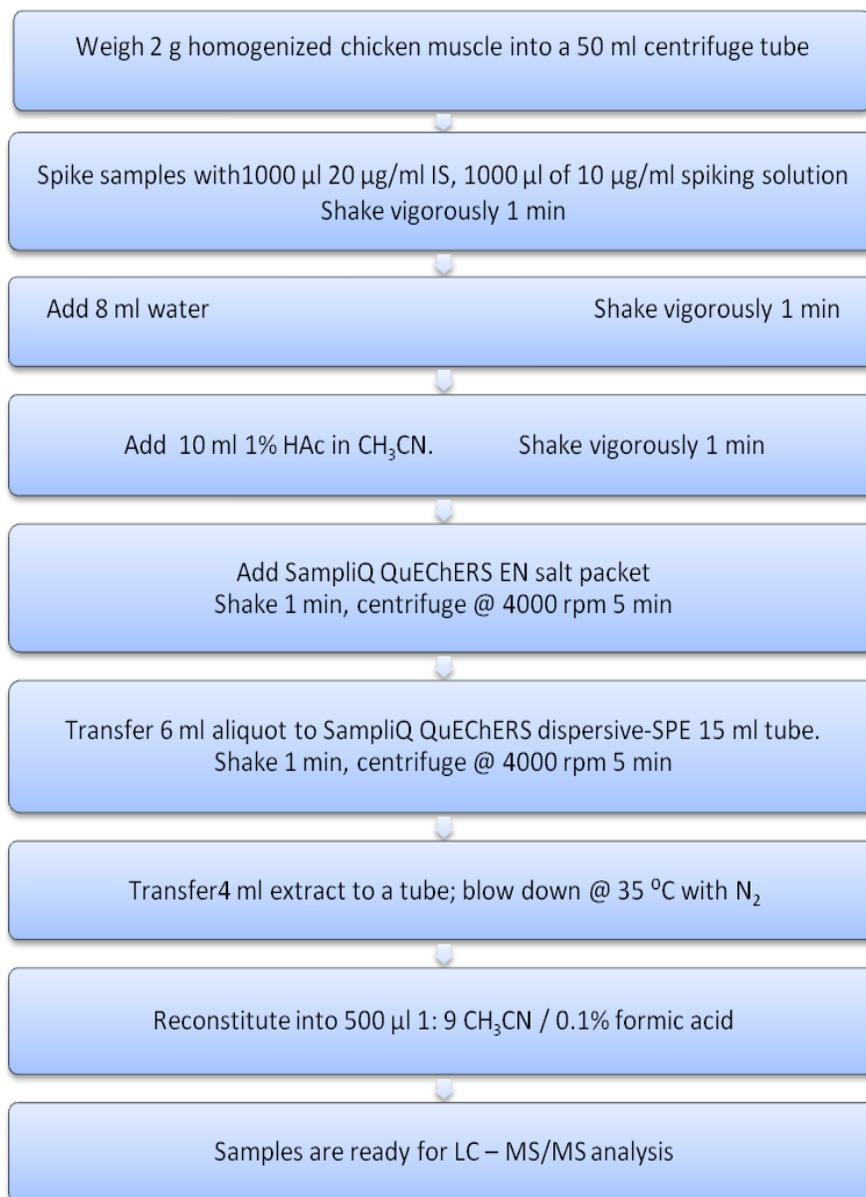
**Scheme 4.5.5 (b): Flow chart of QuEChERS AOAC procedure (LC-MS/MS analysis)**
