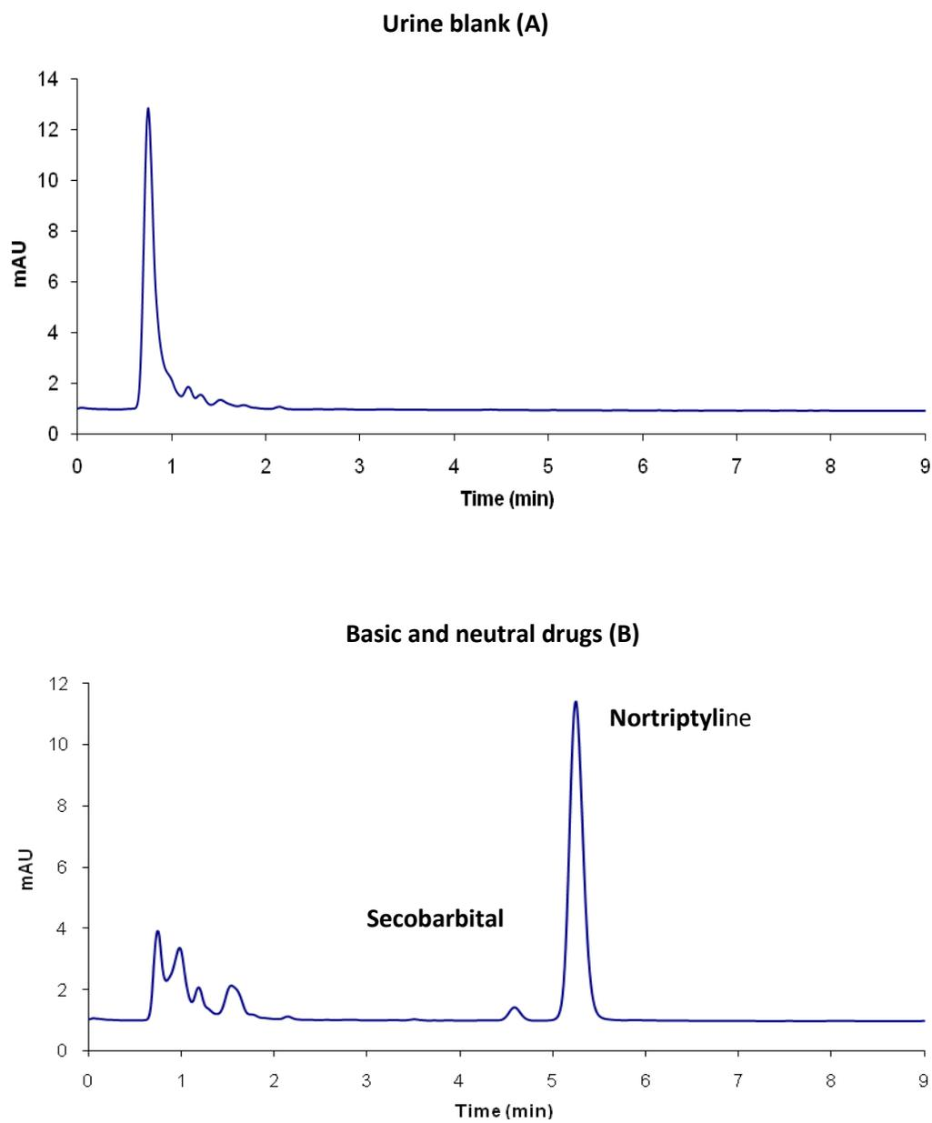
Figure 5.1.3: Eluate 1 chromatograms of (a) blank urine sample; (b) spiked urine sample
