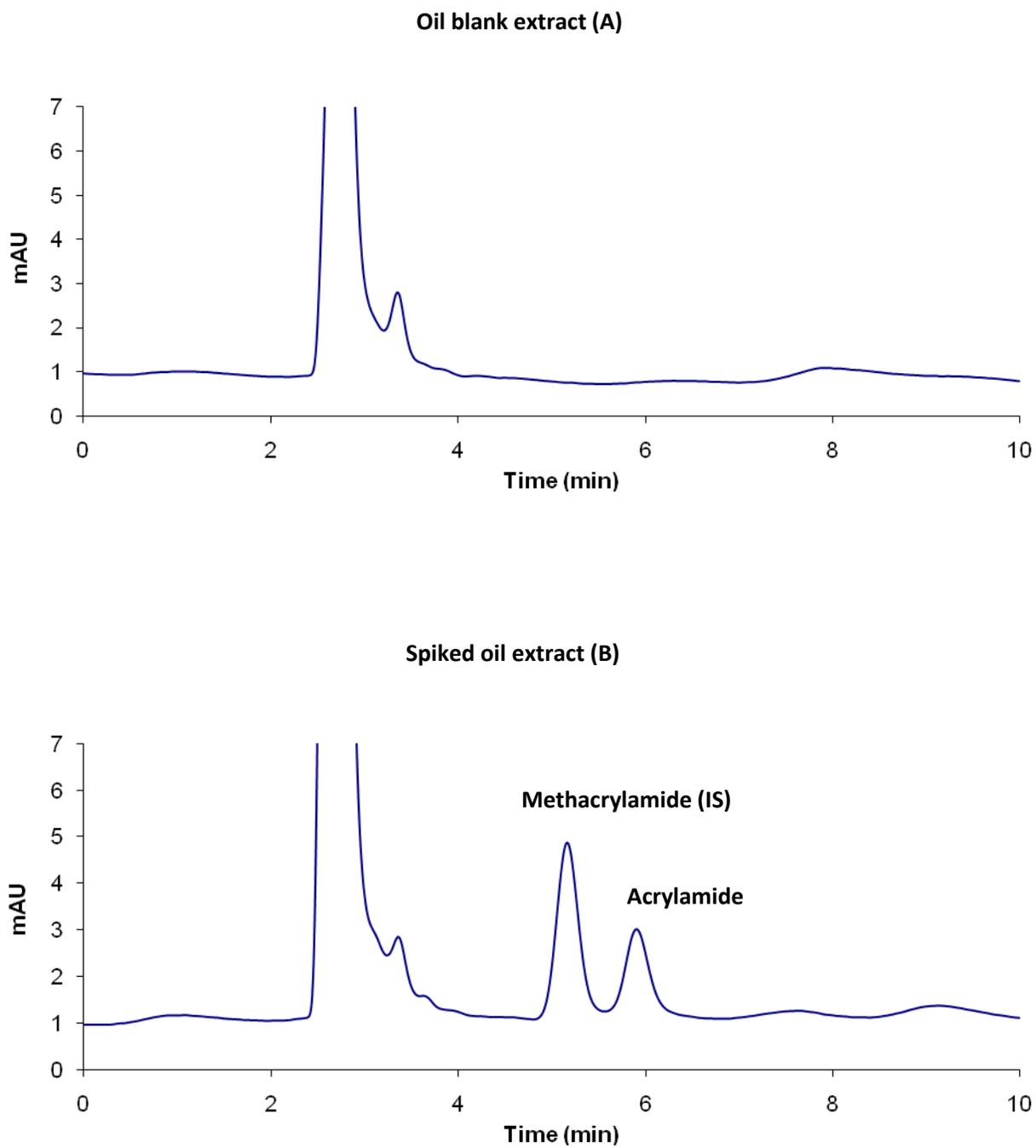
Figure 5.4.2: Chromatograms of; (A) blank oil extract and (B) spiked oil extract
