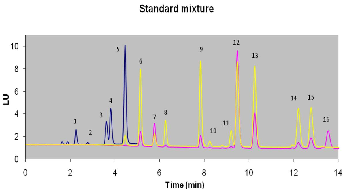
**Figure 5.2.1: Overlay HPLC – FLD chromatograms of the standard mixture containing: 1. Nap 2. Acy 3. Ace 4. Flu 5. Phe 6. Ant 7. Fln 8. Pyr 9. BaA 10. Chr 11. BeP 12. BeA 13. BkF 14. DahA 15. BghiP 16. InP**
