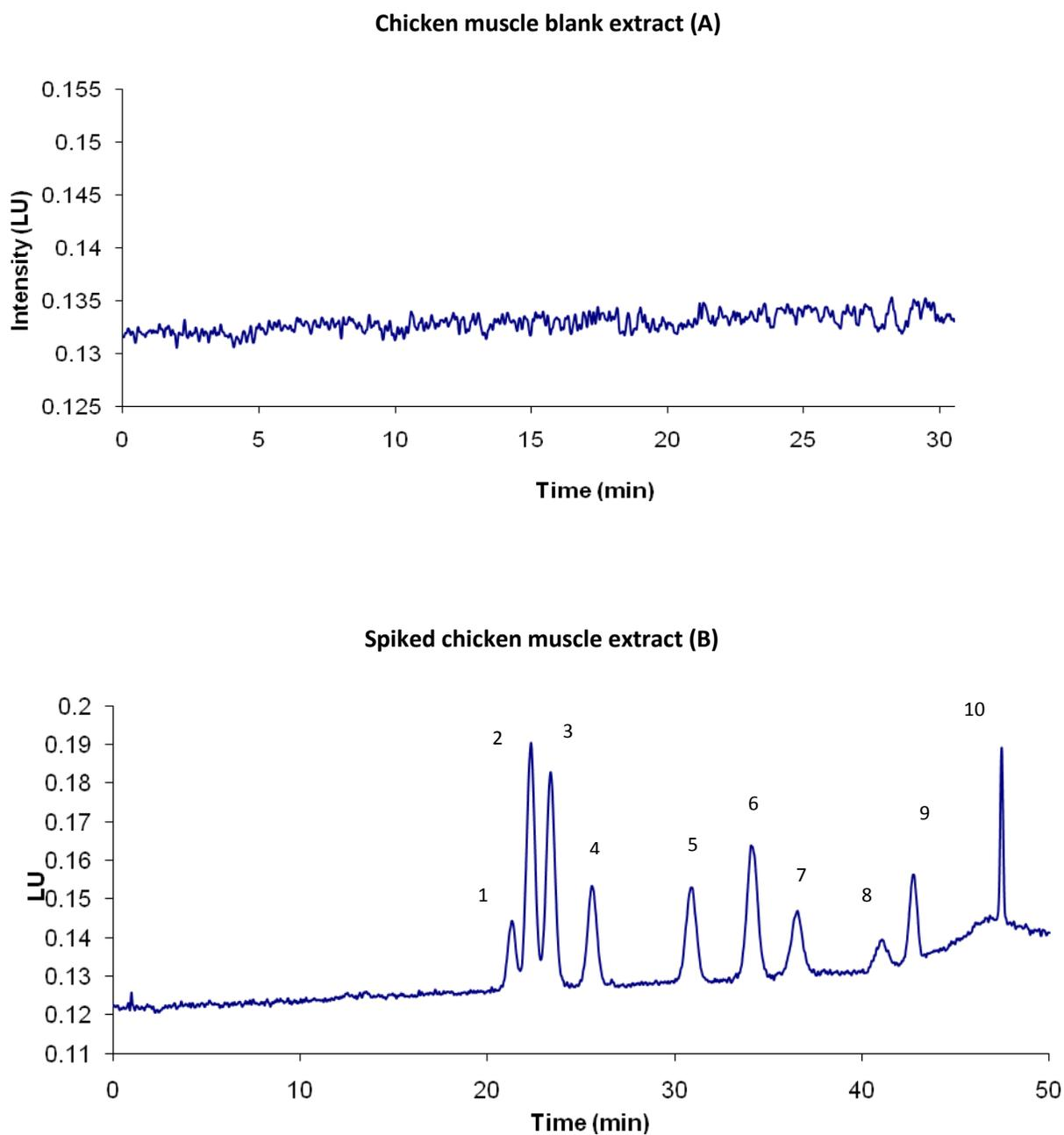
**Figure 5.3.2: Chromatograms of (A) blank chicken muscle; (B) spiked chicken muscle at 50 ng/g level: 1. Sulfadiazine 2. Sulfathiazole 3. Sulfapyridine (IS) 4. Sulfamerazine 5. Sulfamethazine 6. Sulfamethizole 7. Sulfamethoxyypyridazine 8. Sulfachloropyridazine 9. Sulfamethoxazole 10. Sulfadimethoxine (see Fig. 5.3.4 for the mass spectra of these SAs)**
