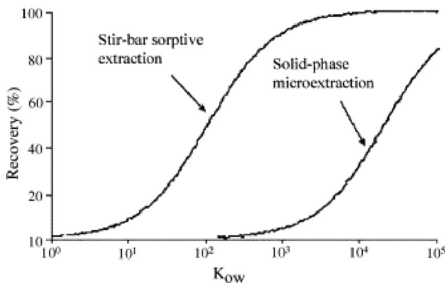
Fig. 2.5.3: Theoretical recovery (%) in function of solute log  $K_{o/w}$  for SPME (100  $\mu\text{m}$  fiber, 0.5  $\mu\text{l}$  PDMS) and SBSE (1 cm  $\times$  0.5 mm df, 25  $\mu\text{l}$  PDMS) and 10 mL sample volume. Equilibrium sampling is assumed [84].
