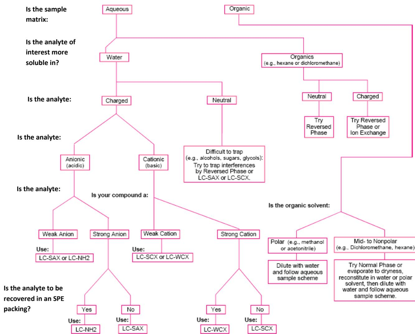
Scheme 2.5.1: Method guide for selection of SPE procedure [62]
