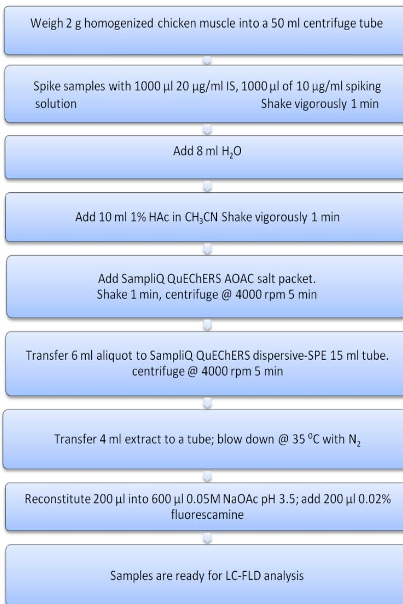
**Scheme 4.5.5 (a): Flow chart of QuEChERS AOAC procedure (LC-FLD analysis)**
