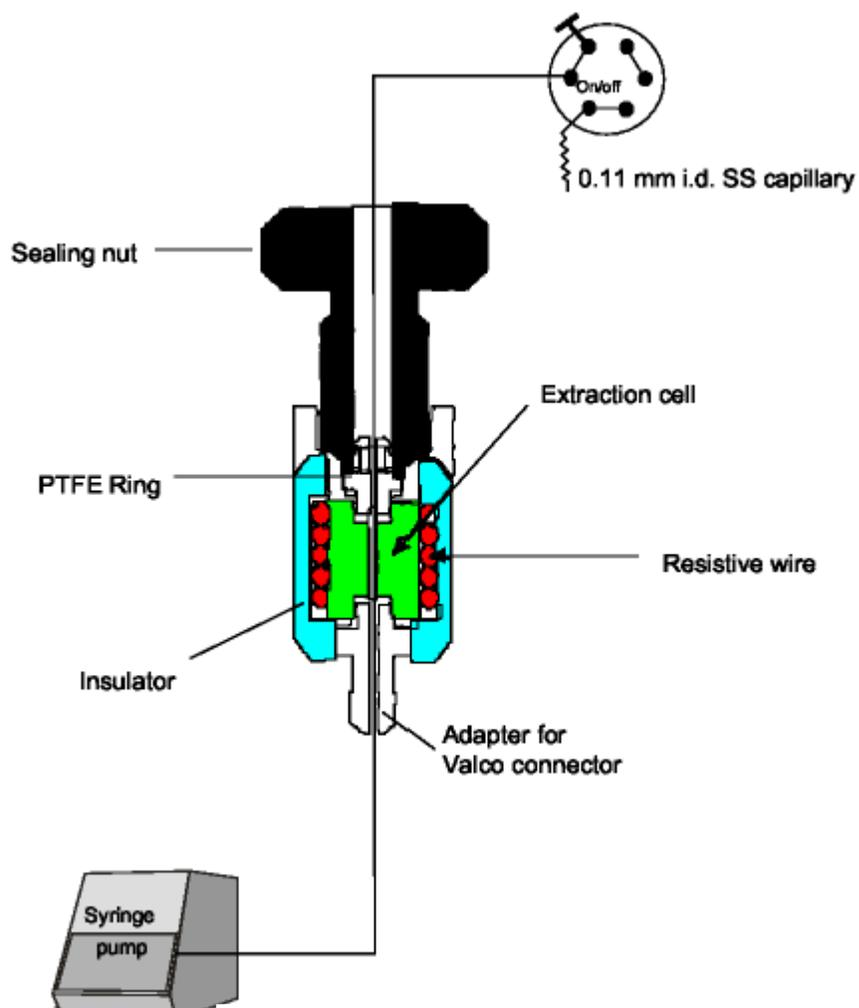
Figure 3.3.2: PLE device for extraction of solid and semi-solid samples [121]
