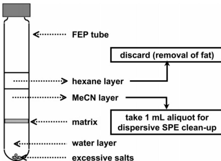
**Figure 3.5.2:** Schematic picture of the solvent layer arrangement in a FEP tube after the centrifugation of a food extract [189].
