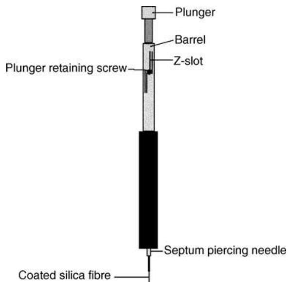
Figure 2.5.3.1: Components of SPME device [90]
