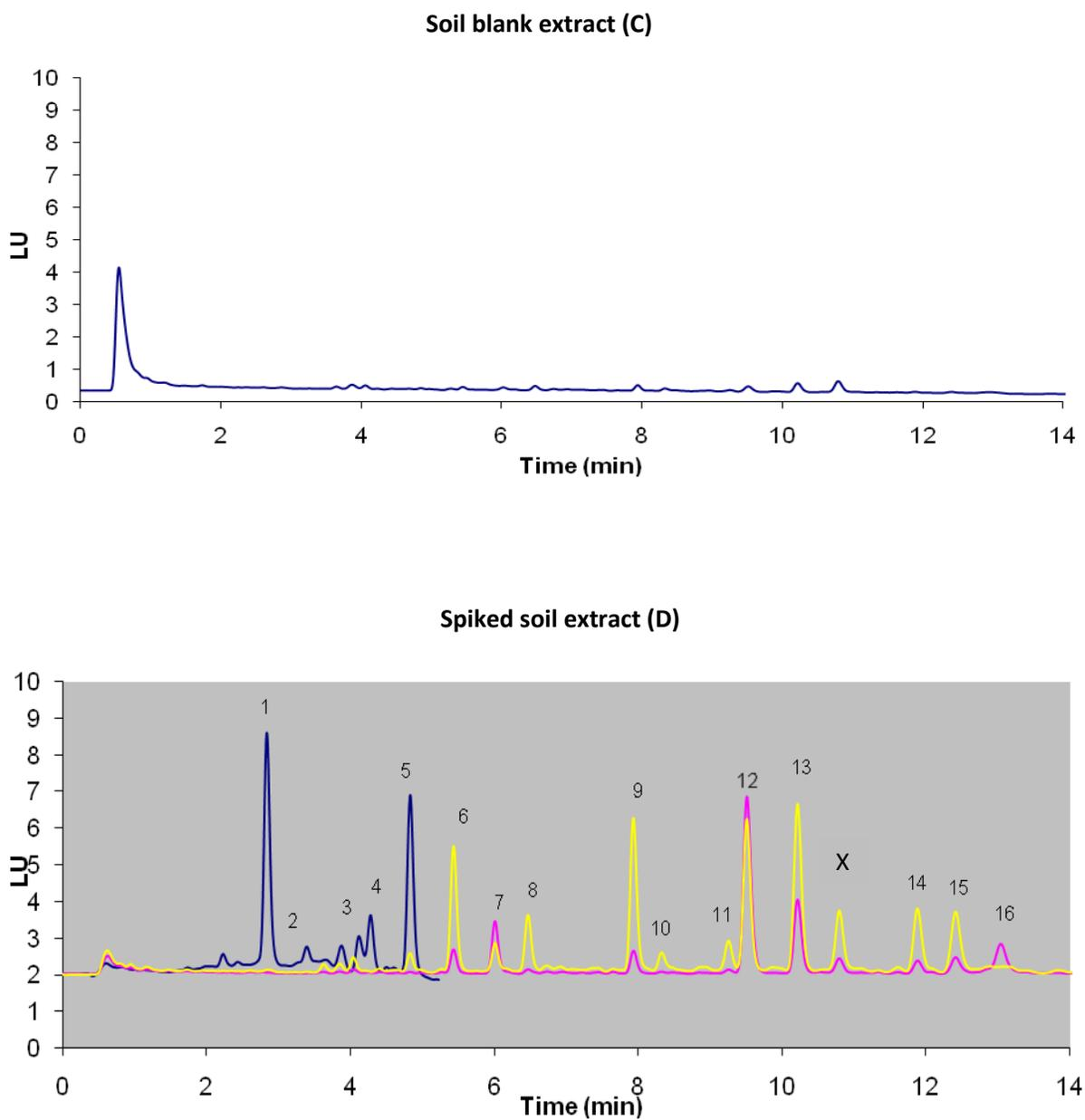
**Figure 5.2.3: (C) Chromatogram of the blank soil extract; (D) Overlay HPLC - FLD chromatograms of the spiked soil sample containing: 1. Nap 2. Acy 3. Ace 4. Flu 5. Phe 6. Ant 7. Fln 8. Pyr 9. BaA 10. Chr 11. BeP 12. BeA 13. BkF 14. DahA 15. BghiP 16. InP X = unknown**
