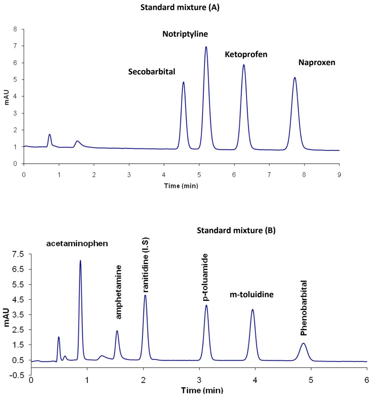
**Figure 5.1.1:** Typical RP-HPLC-DAD chromatograms of standard mixtures: (A) drugs in urine; secobarbital (10  $\mu\text{g}/\text{ml}$ ) nortriptyline (5  $\mu\text{g}/\text{ml}$ ), ketoprofen (5  $\mu\text{g}/\text{ml}$ ) and naproxen (2  $\mu\text{g}/\text{ml}$ ): (B) drugs in plasma (7  $\mu\text{g}/\text{ml}$ ).
