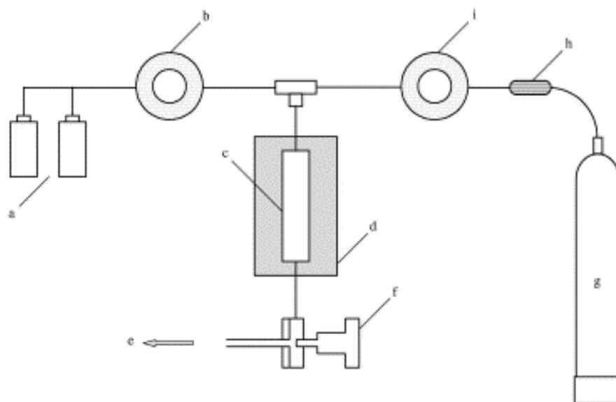
**Fig. 2.3.1: Schematic of SFE equipment: (a) modifier supply, (b) pump, (c) extraction cell, (d) furnace, (e) to collection, (f) flow restrictor, (g) fluid supply, (h) filter and (i) dual high-pressure piston pump [53].**
