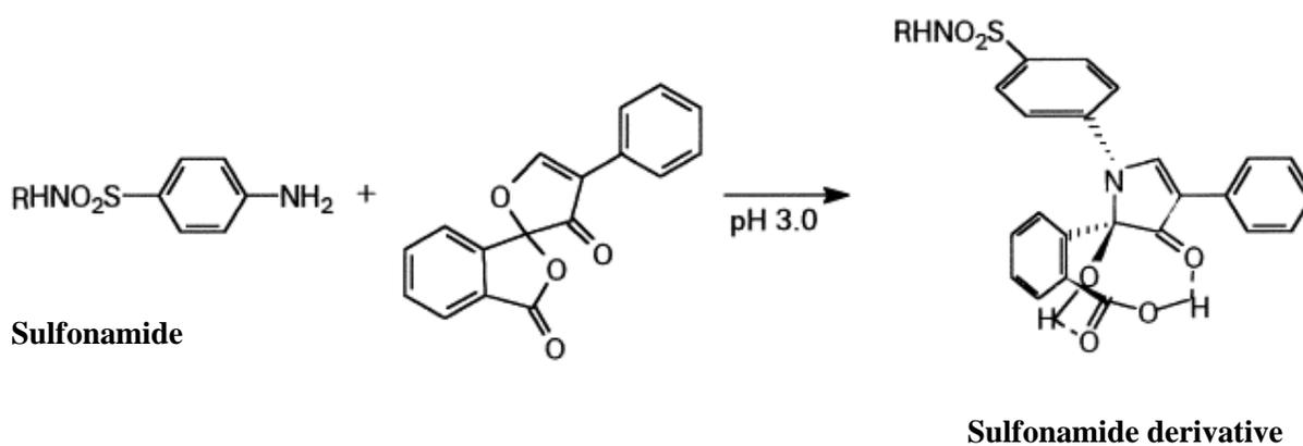
**Figure 3.4.3: A depiction of a chemical reaction for the derivatization of sulfonamides [168].**
