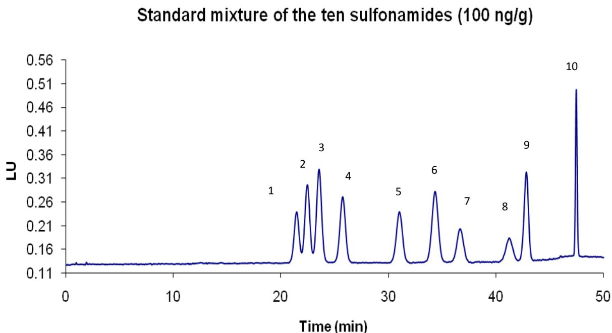
**Figure 5.3.1: Chromatogram of the standard mixture of the sulfonamides (100 ng/g):**
