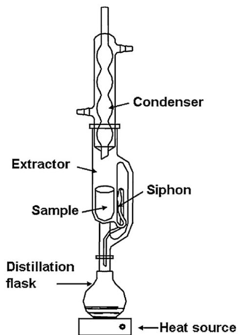
Figure 2.2.1: Conventional Soxhlet extractor [49]
