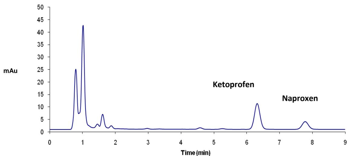
Fig. 5.1.3: (continuation) Eluate 2 Chromatograms of (c) blank urine sample; (d) spiked urine sample; **Chromatographic conditions:** stationary phase, ZORBAX C<sub>18</sub> column (4.6 mm × 75 mm i.d., 3.5 μm); mobile phase, methanol /25 mM phosphate buffer containing pH 2.7; flow rate, 1.5 ml/min; injection volume, 5 μL; detection wavelength, 222 nm.
