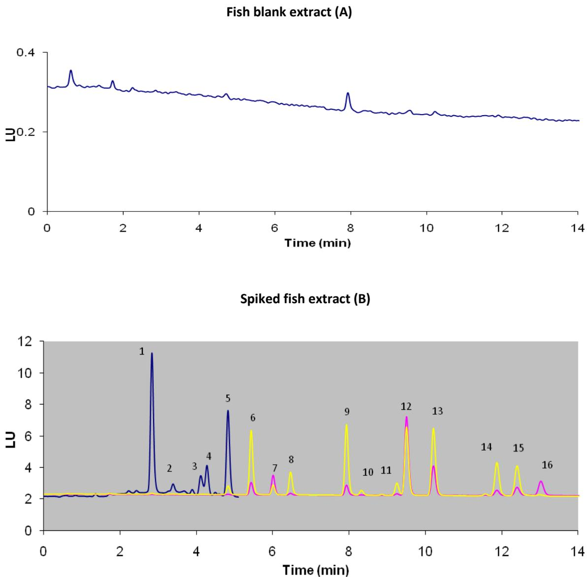
**Figure 5.2.2: (A) Chromatogram of the blank fish extract; (B) Overlay HPLC - FLD chromatograms of the spiked fish sample containing: 1. Nap 2. Acy 3. Ace 4. Flu 5. Phe 6. Ant 7. Fln 8. Pyr 9. BaA 10. Chr 11. BeP 12. BeA 13. BkF 14. DahA 15. BghiP 16. InP**
