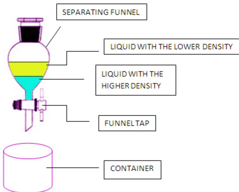
**Figure 2.4.1: Liquid-liquid extraction [57]**
