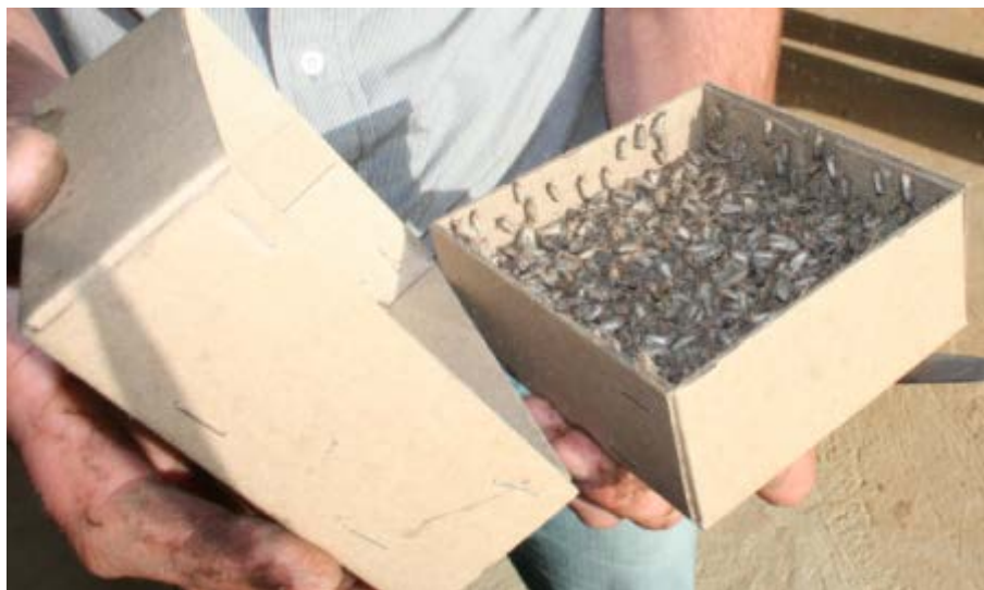
Figure 2.1 A cardboard container used for storage and shipping of irradiated FCM.
