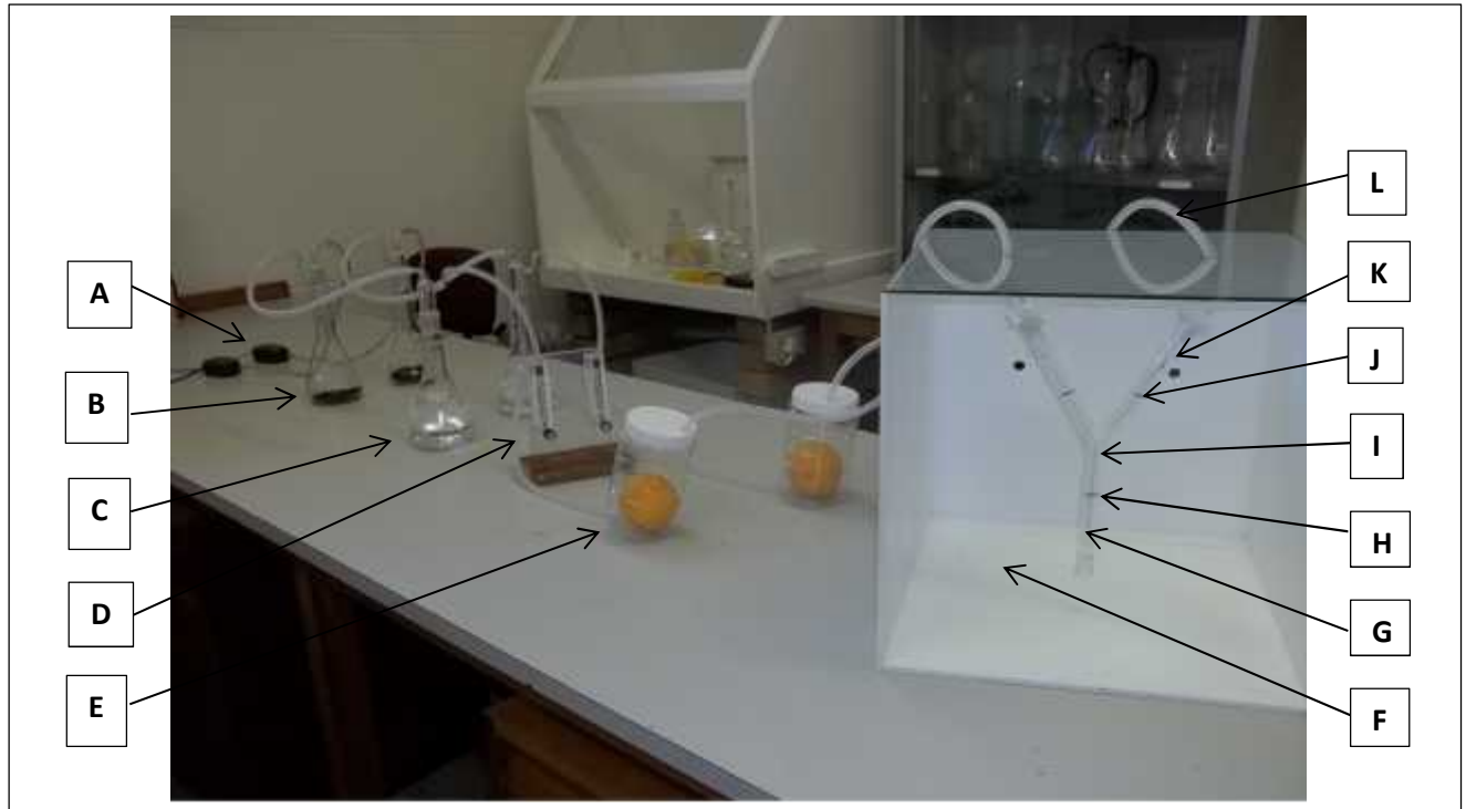
Figure 3.1 Olfactometer setup. A=Air pump; B=Activated charcoal filter; C=distilled water; D=Flow meter; E=Odour source container; F=Perspex cage housing the Y-tube; G=Base arm of Y-tube; H=Starting line; I=Y-tube olfactometer; J=Choice line; K=Upper arm of Y-tube; L=Air flow tubes.
