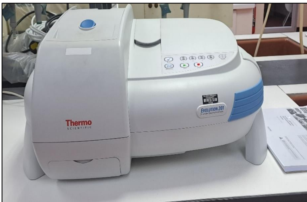
Figure 3.5: Thermofisher Scientific spectrophotometer (UV-Vis Evolution 200 series) used in this research.
