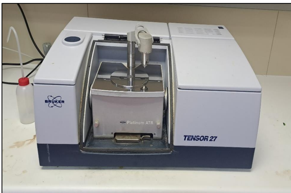
Figure 3.4: Bruker platinum ATR Tensor 27 IR spectrophotometer used in this work.
